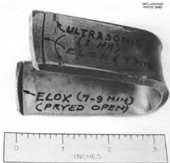
Fig. F-1. Ultrasonic and Elox Cutting of Inconel.
