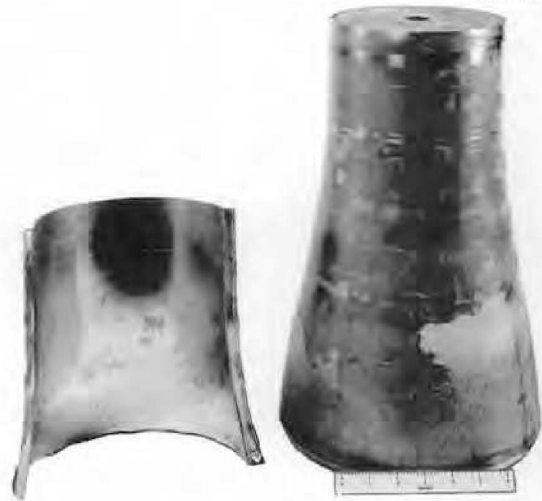
Fig. 15. Lead Alloy Replica of a Reactor Component.
