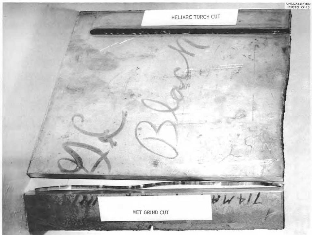
Fig. 12. Wet Grind Cut. A 1-ft length of \frac{1}{2} -in.-thick Inconel plate, cut in approximately 1 min with a water-flushed, 24-in.-dia abrasive wheel operating at about 10,000 surface feet per minute.
