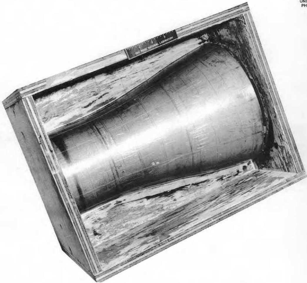
Fig. 17. Mold for Making Replicas of Radioactive Components.
