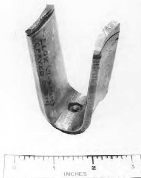
Fig. G-1. Inconel Plate Cut by Elox Process.
