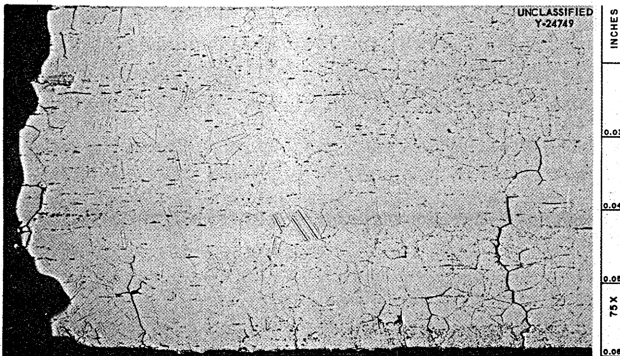
Fig. 2.1.31. Diverse Cracks in Hastelloy B Nipple. Etchant: chromic and hydrochloric acids. 75X.
