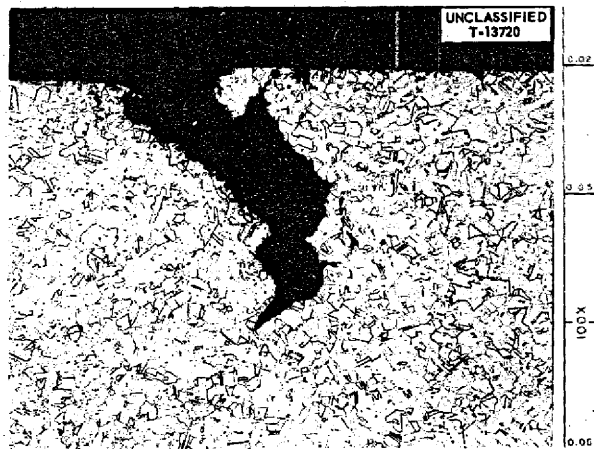
Fig. 2.1.38. Specimen Showing a Crack Found in Weld Area of Weld drawn INOR-8 Tubing. Etchant: aqua regia. 100X. Reduced 31%.
