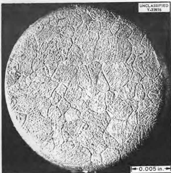
Fig. 1.2.12. Surface of the End of an Yttrium Cylinder Following Exposure to Lithium for 100 hr at 1500°F. Reduced 34%. (Secret with caption)
