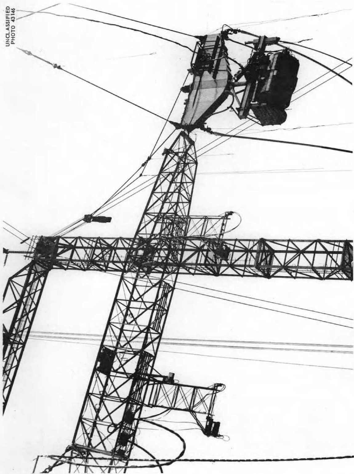
Fig. 4.4.6. Closeup of the ASTR and Two Groups of Detectors Suspended from the Truss.
