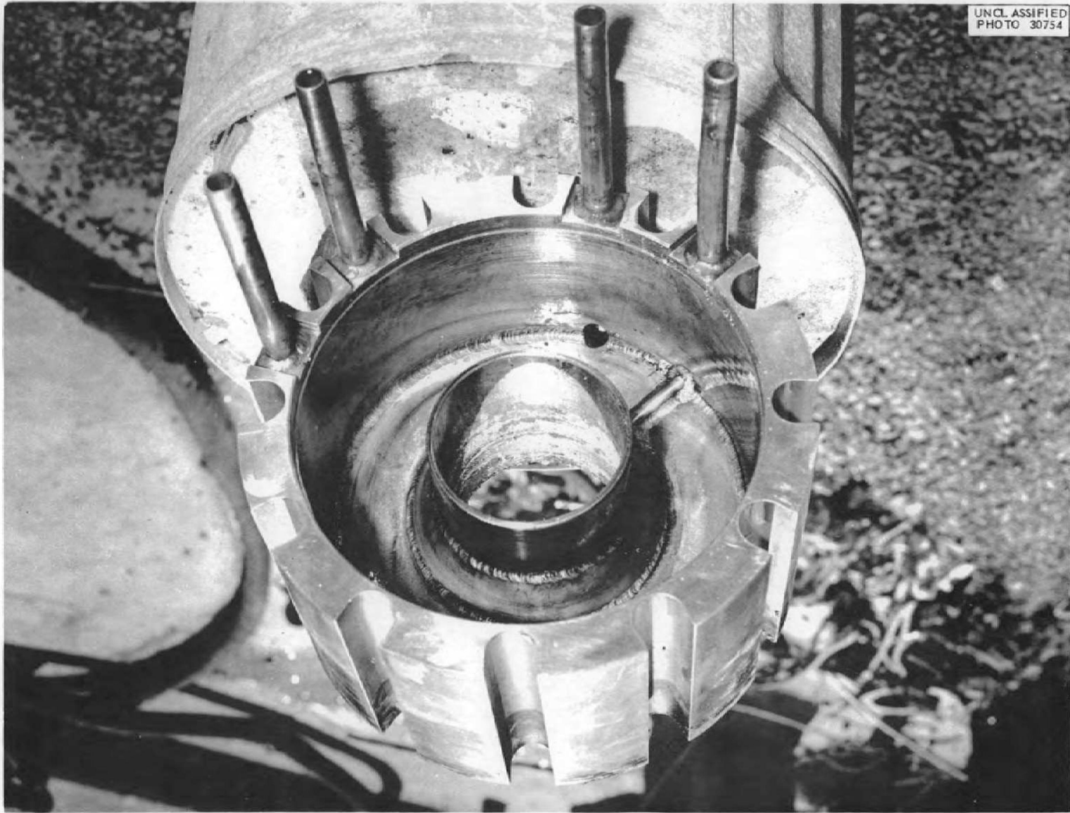
Fig. 3.1.2. Oil-Leakage Catch Basin and Outer Wall of Shaft Annulus of Centrifugal Pump Operated with a Split-Purge Arrangement to Prevent the Rise of Vapor from the Pumped Fluid.
