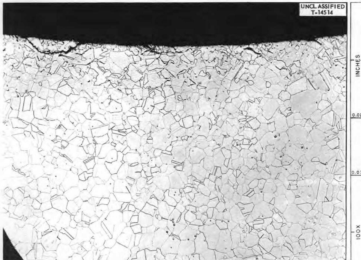
Fig. 3.2.1. Effect of High-Frequency Thermal Cycling on Inconel in an \text{NaF-ZrF}_4\text{-UF}_4 (56-39-5 mole %) Environment - Test 6. Etchant: Marble's reagent. 100X. (Secret with caption)
