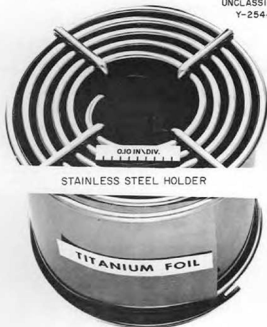
Fig. 1.2.8. Titanium Gettering Foil and Stainless Steel Support Assembly for Foil.
