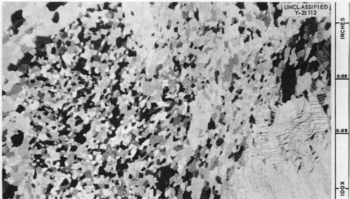
Fig. 1.1.4. Sample L-10A-2 Under Polarized Light Illumination. 100X. Etchant: \text{HNO}_3\text{-H}_3\text{PO}_4\text{-CH}_3\text{COOH} .
