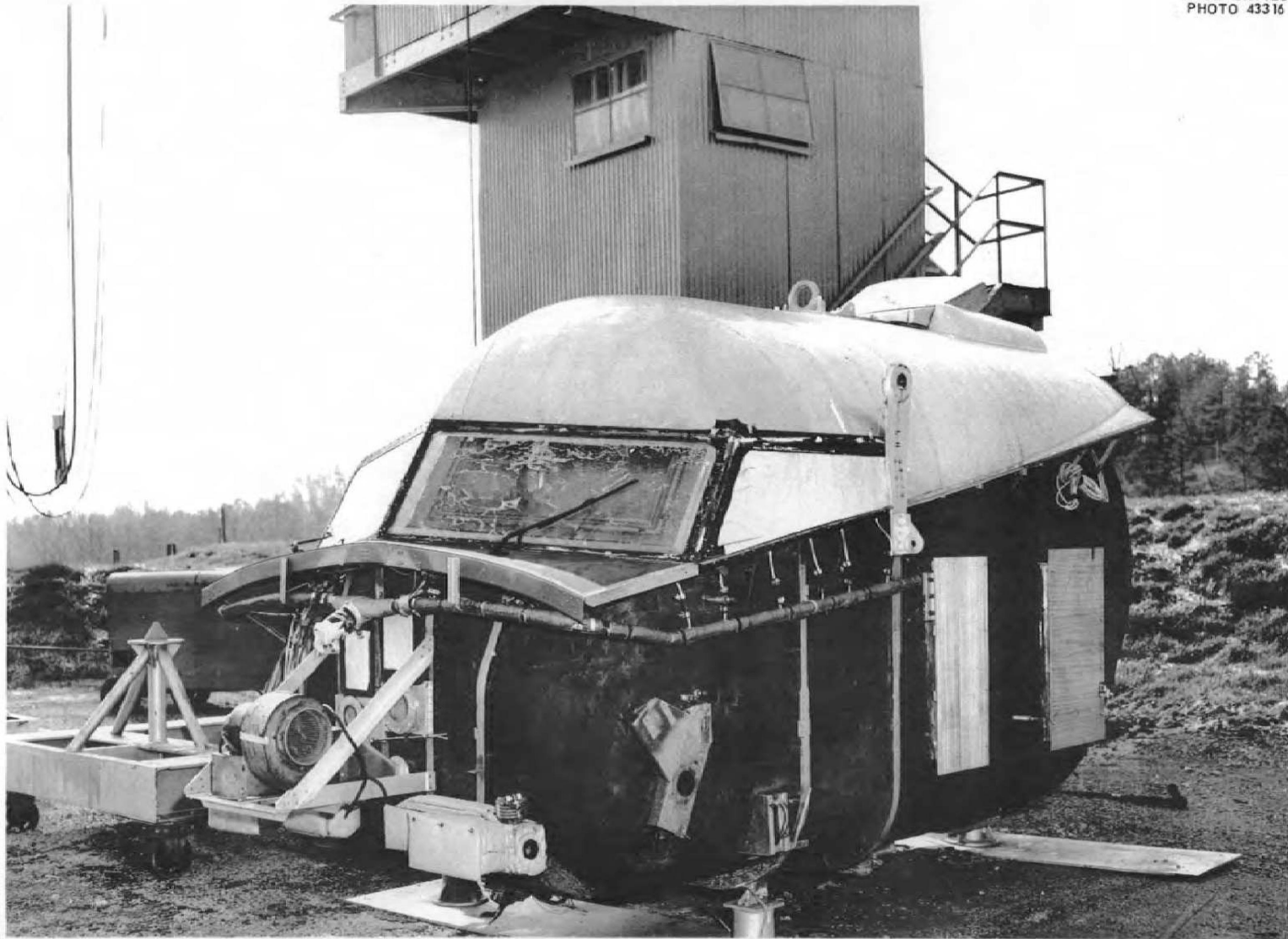
Fig. 4.4.3. The NTA Crew Compartment.
