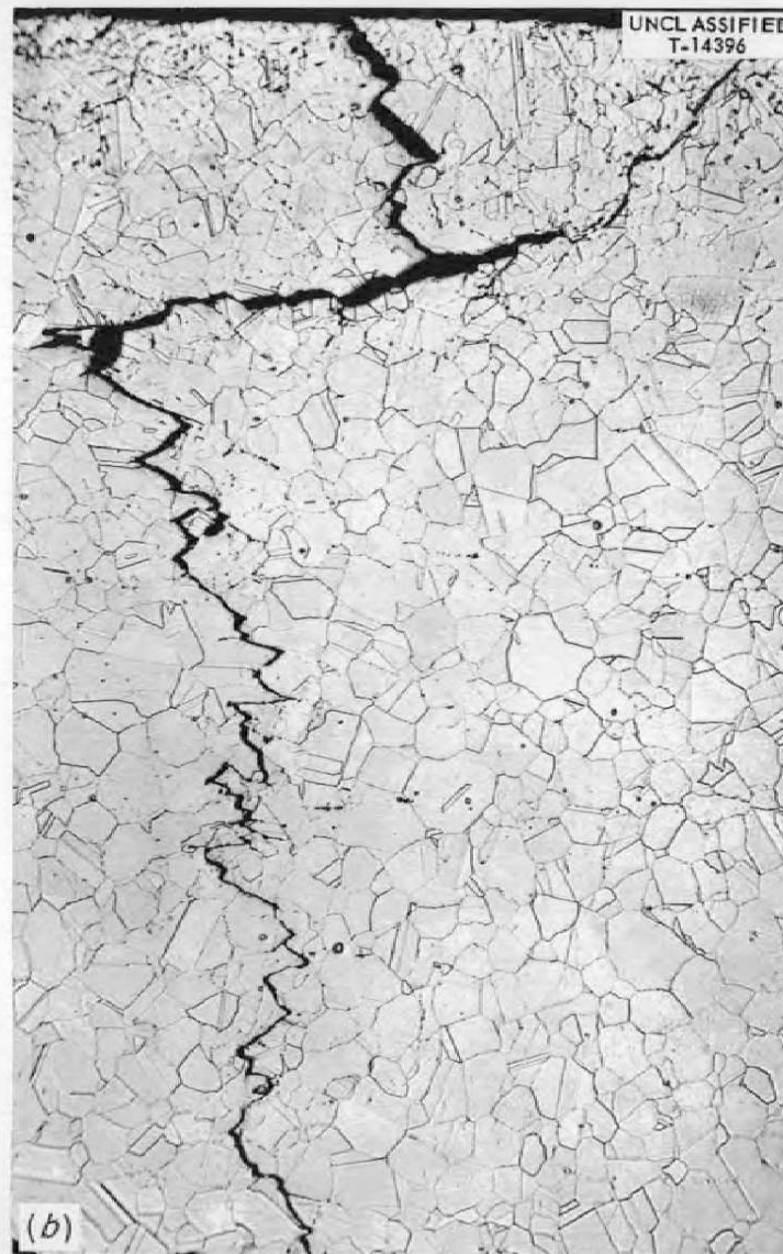
Fig. 3.2.2. Effect of High-Frequency Thermal Cycling on Inconel in an \text{NaF-ZrF}_4\text{-UF}_4 (56-39-5 mole %) Environment - Test 8. Etchant: Marble's reagent. (a) 75X; (b) 100X. Reduced 4%. (Secret with caption)
