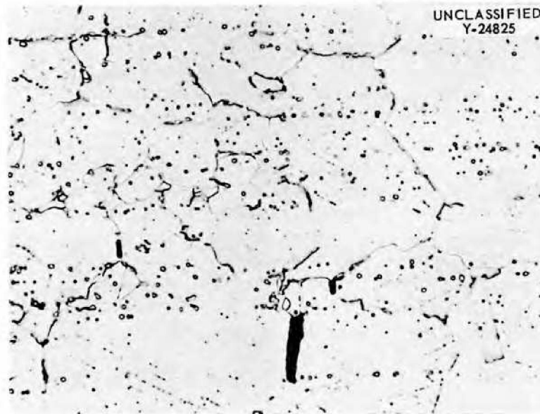
Figure 24. Alloy VT-45, 15 Mo - 5 Cr - 4 Fe - 0.5 Al - 0.5 Mn - 0.06 C - Balance Ni. Longitudinal section in gage length of creep-rupture specimen. Rupture life: 218.2 hr. Etchant: Glycera Regia. 500X.
