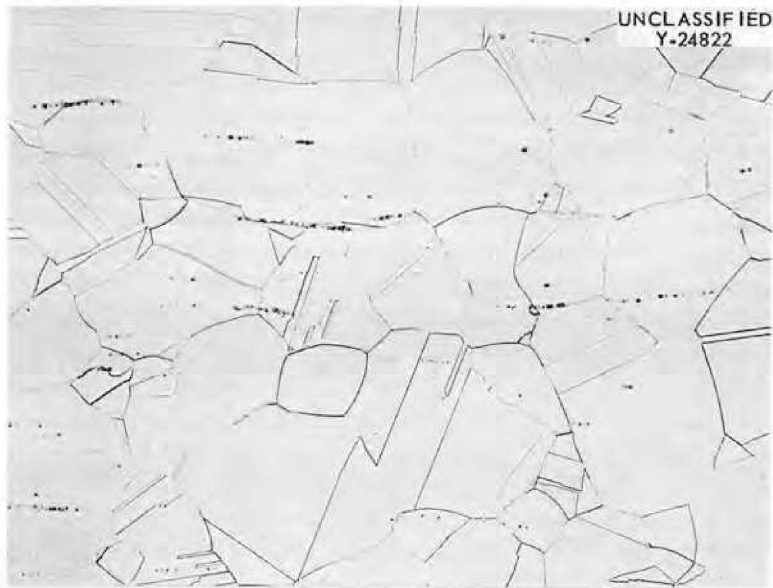
Figure 9. Alloy VT-47, 10 Mo - 7 Cr - 4 Fe - 0.5 Al - 0.5 Mn - 0.06 C - Balance Ni. Solution-annealed 1/2 hr. at 2100°F. Etchant: Glycera Regia. 100X.
