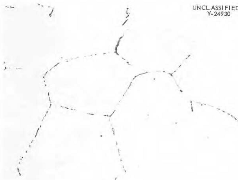
Figure 39. Alloy VT-87, 15 Mo - 7 Cr - Balance Ni. Solution-annealed 1/2 hr. at 2100°F, aged for 100 hr. at 1500°F. DPH 158. Etchant: Glycera Regia. 500X.
