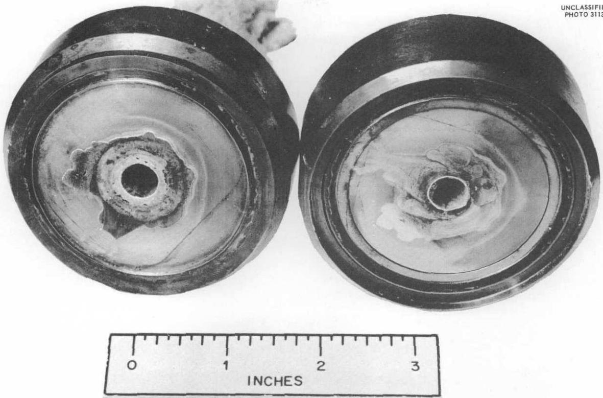
Fig. 1.2.4. Indented-Seal Flange Joint Separated After Testing.
