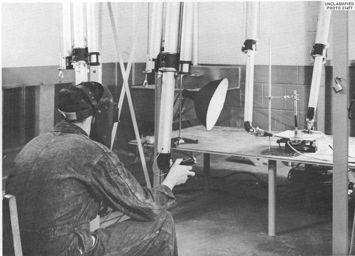
Fig. 1.2.8. Remote Welding of Plate.
