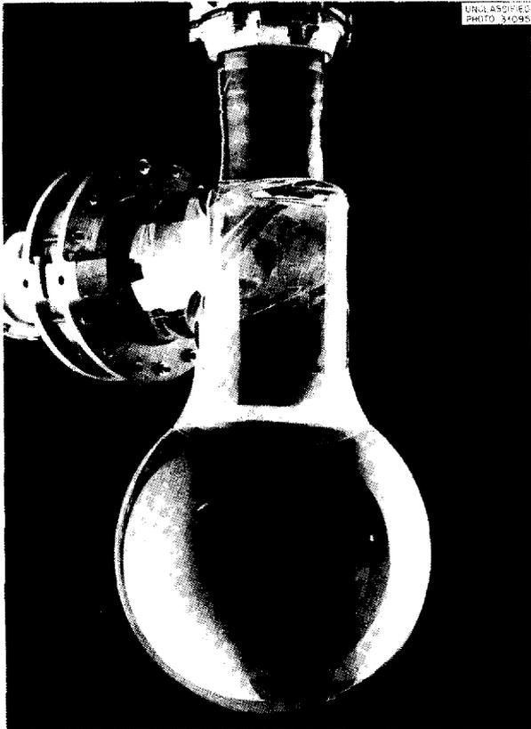
Fig. 1.3.3. Concentric Entrance-Exit Model (MSR-3) Designed for Fluid Entrance Through Outer Annulus.
