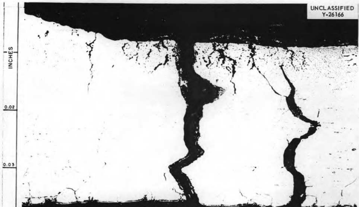
Fig. 1.7.2. Typical Cracks Found in Tension Side of a Tube. Etchant: 10% oxalic acid. 100X.
