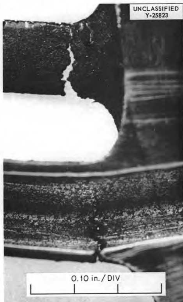
Fig. 1.7.1. Cracks in Two of Three Cracked Inconel Tubes Found in the High-Temperature Header Area of a Semicircular Fused Salt-to-NaK Heat Exchanger. Cracks are in the tension side of the tubes.
