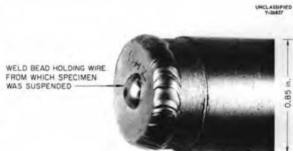
Fig. 1.2.7. Enlargement of Hot-Zone End of Molybdenum Capsule From Test SS-526. Welding operations were performed in an inert-atmosphere chamber. This section of the test capsule was at 1800°F for 500 hr. (Continued with caption)
