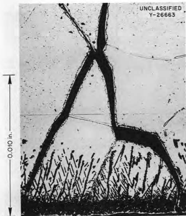
Fig. 1.2.4. Enlargement of Crack Shown in Fig. 1.2.3a.
