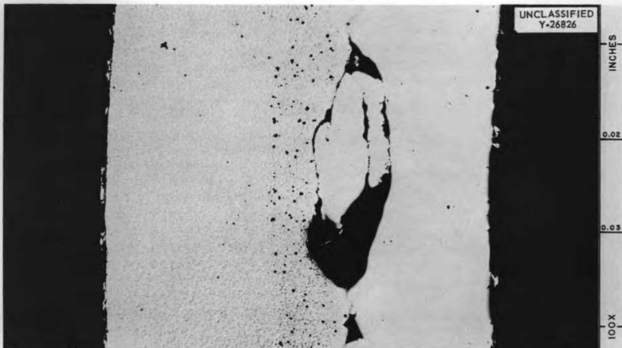
Fig. 1.6.1. Very Poor Bond Between Type 1030 Steel Cladding and Type 304 Stainless Steel in 1/2-in.-OD, 0.042-in.-Wall Tube.
