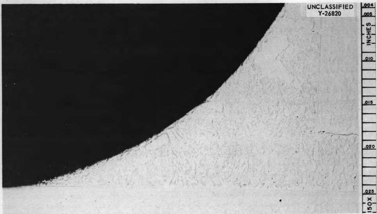
Fig. 1.3.3. Molybdenum T-Joint Brazed with an Alloy Containing 70 wt % Zr and 30 wt % V. As-polished. 50X. ( [redacted] with caption)
