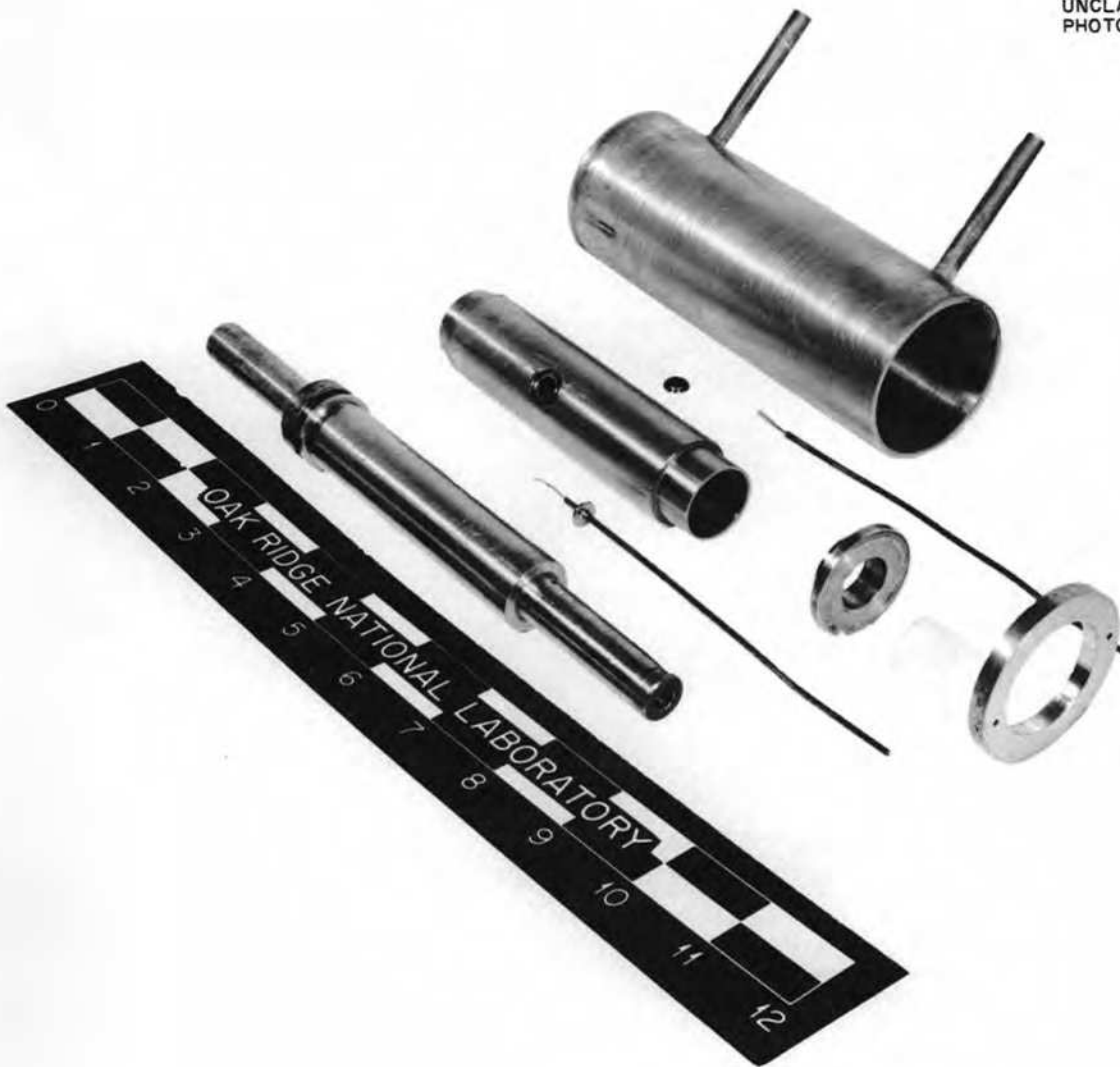
Fig. 2.3.3. Mockup Device Used in Designing and Testing the Thermocouple Installation Used in the Apparatus for High-Temperature Irradiation of Moderator Materials.
