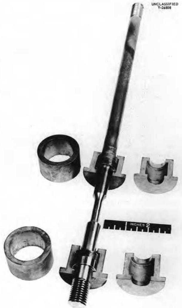
Fig. 1.4.2. Specimen, Pull Rods, and Grips Used in Apparatus Shown in Fig. 1.4.1.
