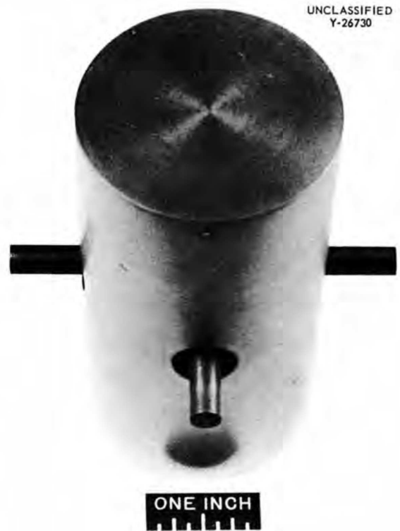
Fig. 2.1.29. Pump Journal Bearing Subassembly After Brazing.
