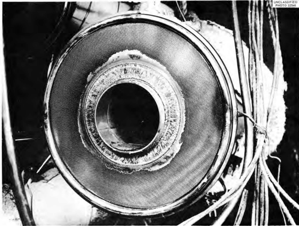
Fig. 1.2.13. Disassembled Freeze-Flange Joint Showing Frozen Salt Seal on Insert Screen.
