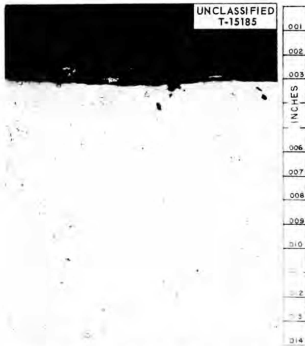
Fig. 2.1.3. Hot-Leg Sample from Salt Circuit of Inconel Forced-Circulation Loop CPR Which Circulated Salt 122 for 9148 hr at 1300°F.
