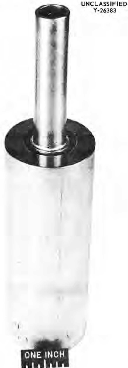
Fig. 2.1.24. Brazed Tube-to-Header Specimen Showing Excellent Filleting.
