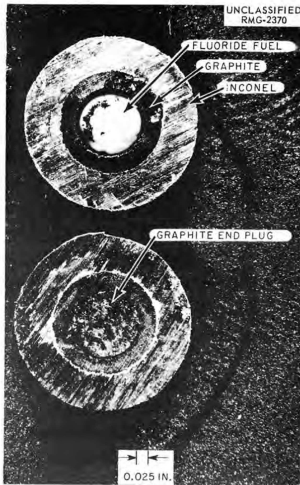
Fig. 2.2.2. Fuel-Filled Graphite Control Capsule Tested Out-of-Pile at 1250°F for 3389 hr. 7X.
