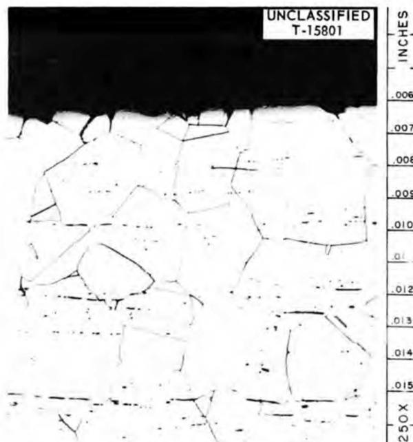
Fig. 1.2.23. Top of INOR-8 Specimen Exposed to Aluminum Chloride Gas at 1200°F for 1000 hr. Etchant: aqua regia. 250X.
