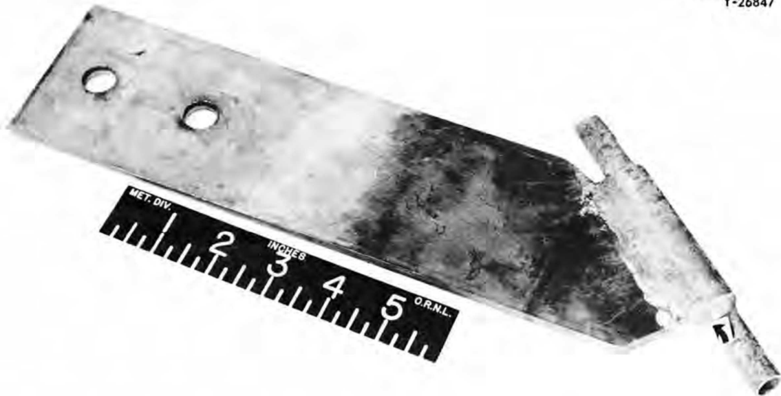
Fig. 2.1.22. INOR-8 Heater Lug Section of Forced-Circulation Loop 9354-1 That Failed During Service. Arrow indicates point of failure.
