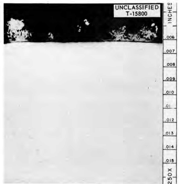
Fig. 1.2.24. Bottom of INOR-8 Specimen Exposed to Aluminum Chloride Gas at 750°F for 1000 hr. As polished. 250X.
