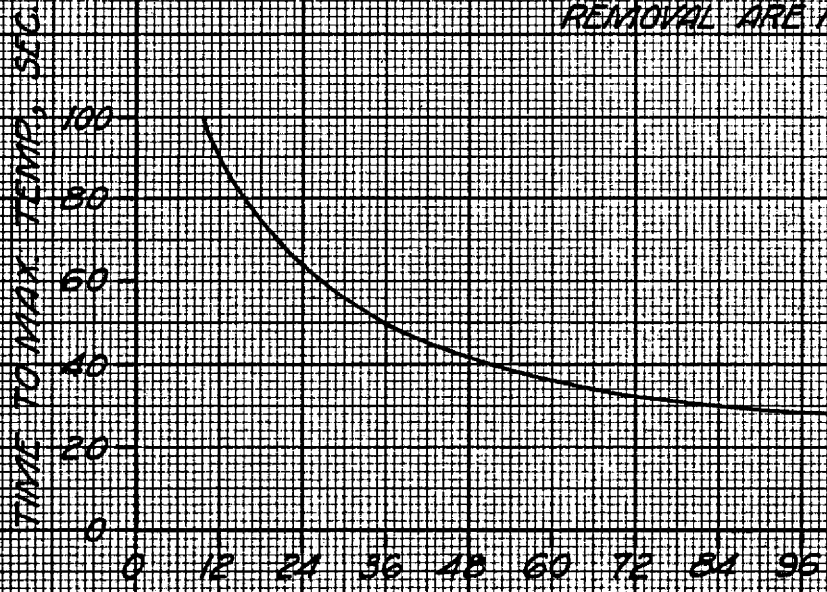
FIG. 115-POWER REMOVAL FROM CORE IN MW WITH NO CORE FLOW FOLLOWING 600 MW OPERATION
