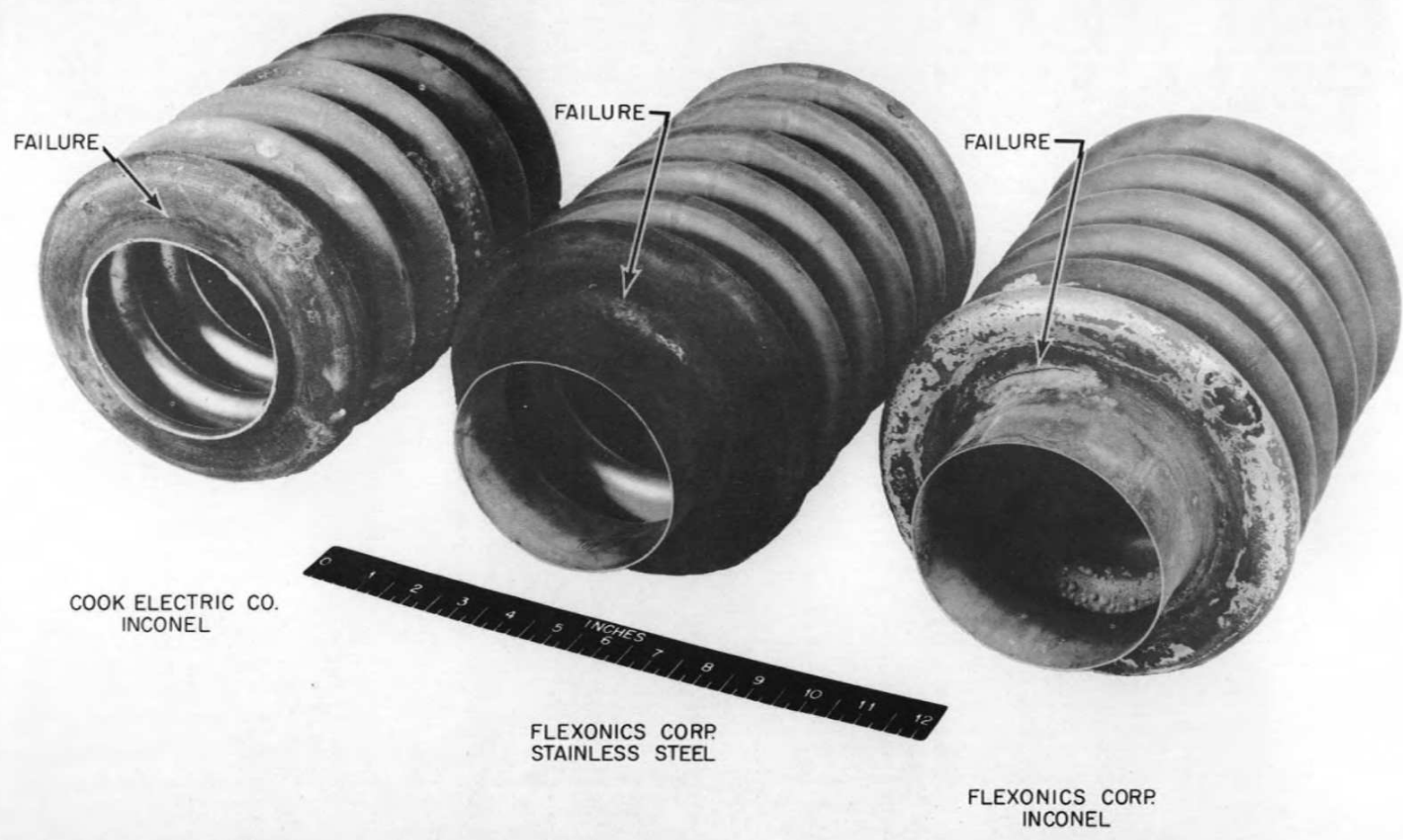
Fig. 1.2.9. Bellows Removed from Expansion Joints Tested in a Molten Salt or Sodium at 1300°F Showing Location of Failure.
