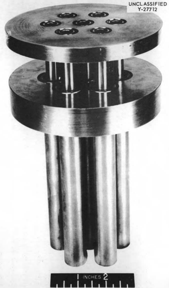
Fig. 2.1.4. Mockup Heat Exchanger Assembly After Welding of Inner and Outer Tubes to Headers.
