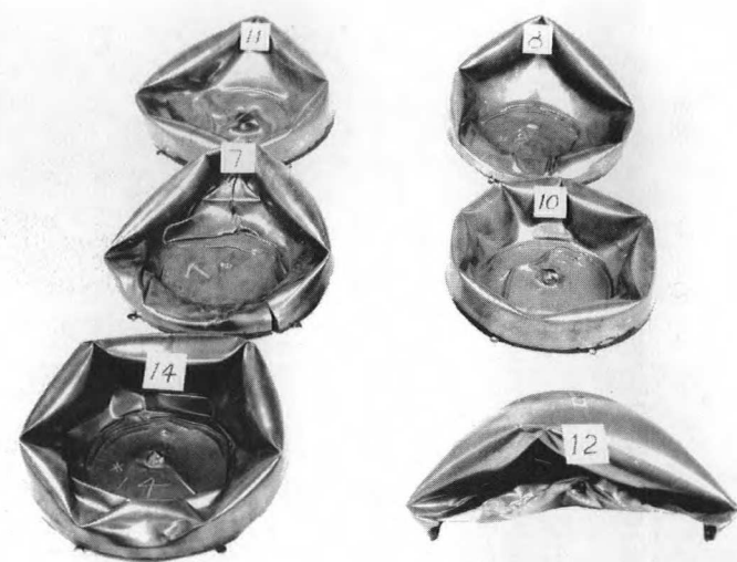
(a) SHELLS 10 in. IN DIAMETER, 0.015-in. WALL, TESTED AT 300°F
