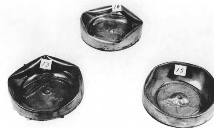
(c) SHELLS 10 in. IN DIAMETER, 0.023-in. WALL, TESTED AT 300°F
