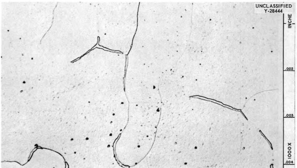
Fig. 1.4.9. Specimen of Heat K-4 Which was Annealed for 2 hr at 1300°C in Vacuum and Tested in Creep at 15,000 psi and 1800°F in an Environment of Static Argon for 718 hr (Test 124). Etchant: H_2O-HF-HNO_3-H_2SO_4 . [REDACTED] with caption)
