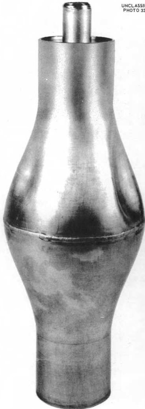
SHELL NO. 3 BUCKLING TIME 199.9 hours
