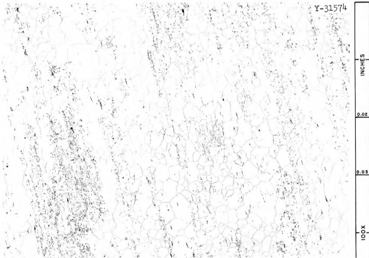
Fig. 2 Heat SP 19 Annealed 1 Hr at 2100°F. Etchant: Aqua Regia. 100X.
