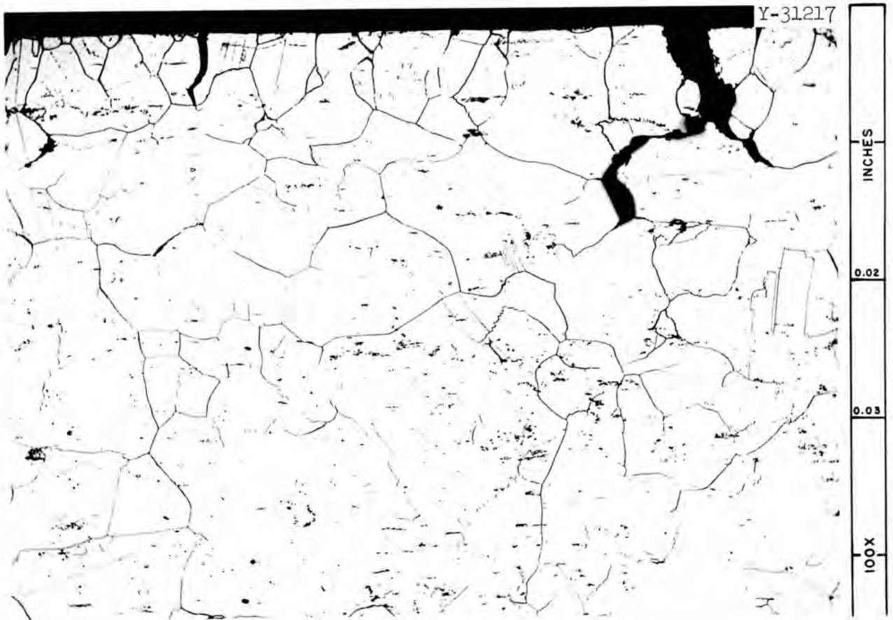
Fig. 30 Heat SP 16 Annealed 1 Hr at 2000°F. Creep tested in molten salt at 1500°F and 8,000 psi. Rupture in 529 hr. Etchant: Aqua Regia. 100X.
