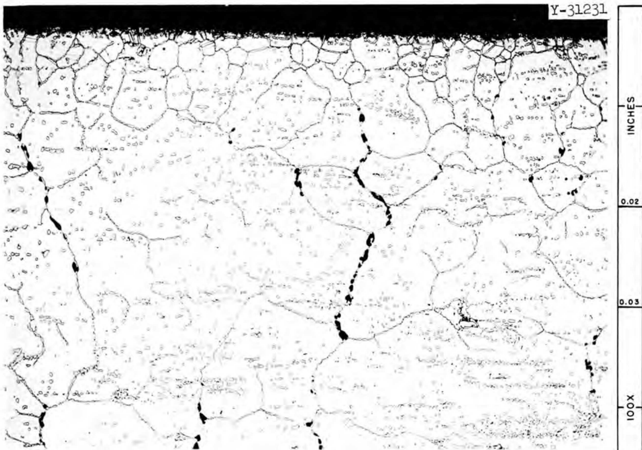
Fig. 33 Heat SP 16 Annealed 1 Hr at 2000°F. Creep tested in molten salt at 1800°F and 2,000 psi. Rupture in 4481 hr. Etchant: Aqua Regia. 100X.
