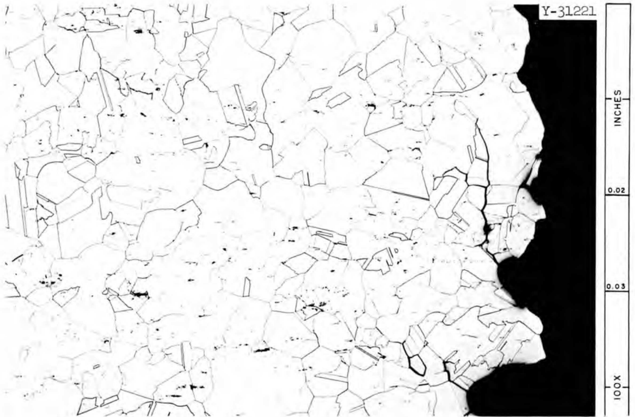
Fig. 26 Heat SP 16 Annealed 1 Hr at 2000°F. Creep tested in molten salt at 1100°F and 30,000 psi. Rupture in 3537 hr. Etchant: Aqua Regia. 100X.
