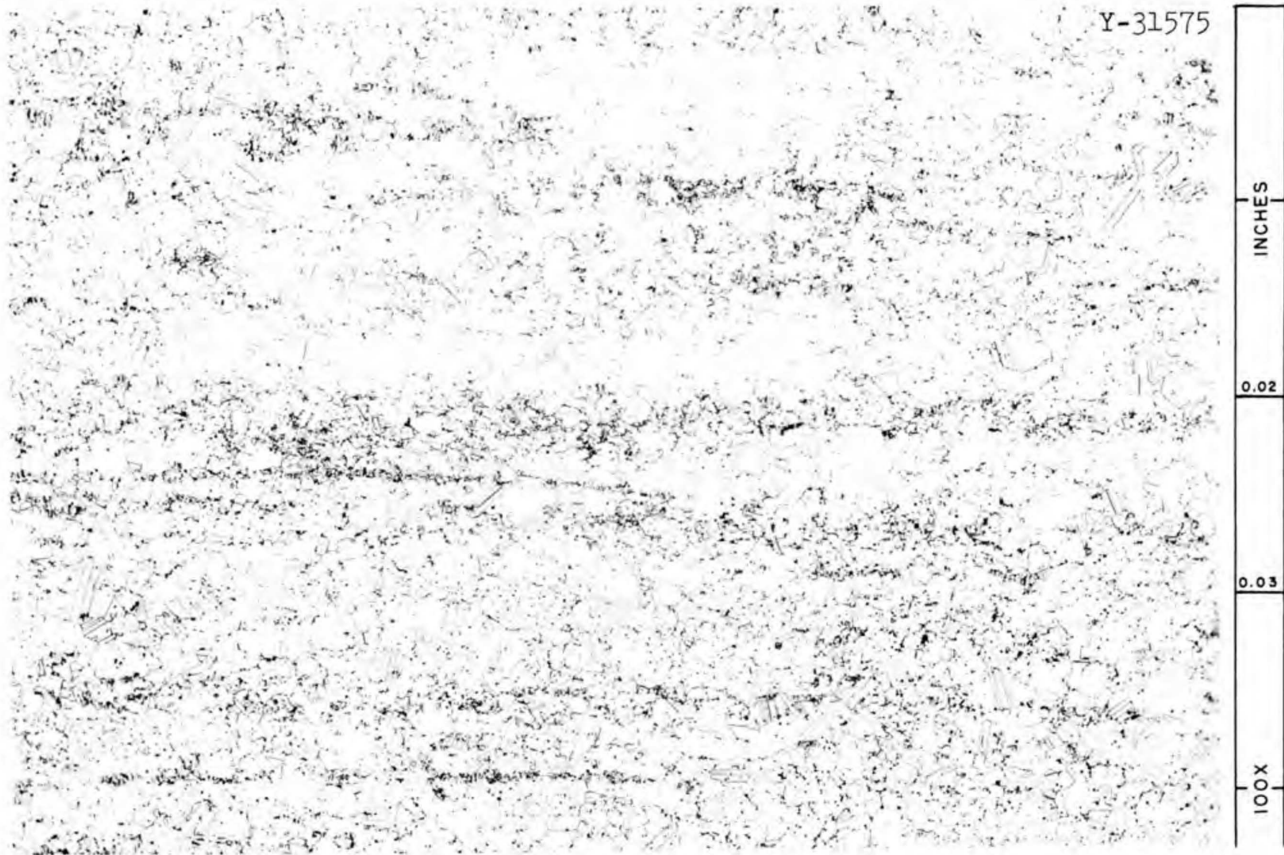
Fig. 4 Heat 8M-1 Annealed 1 Hr at 2100°F. Etchant: Aqua Regia. 100X.
