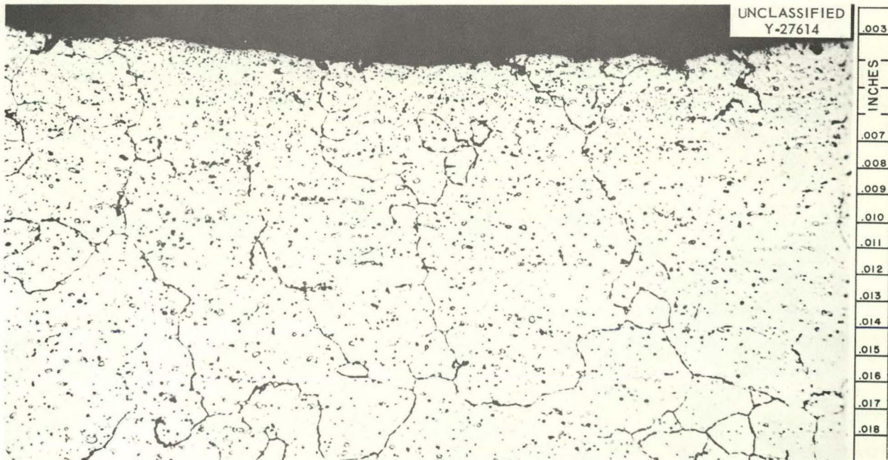
Fig. 75B. Portion of Fig. 75A. Typical Surface and Microstructure. Etchant: Chromium regia. 200X.
