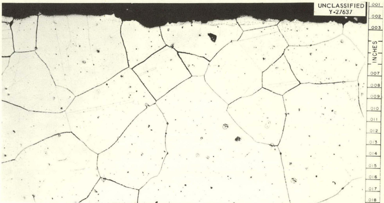
Fig. 77B. Portion of Fig. 77A. Typical Surface and Microstructure, Etchant: Aqua regia. 200X.
