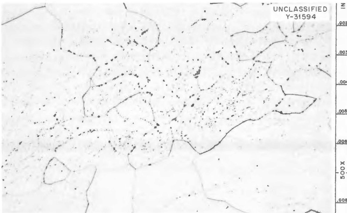
Fig. 1.13. Specimen of Cb-1.5% Zr Alloy Aged 1000 hr at 1500°F. Etchant: 55% H 2 O-25% HF-10% H 2 SO 4 -10% HNO 3 .
