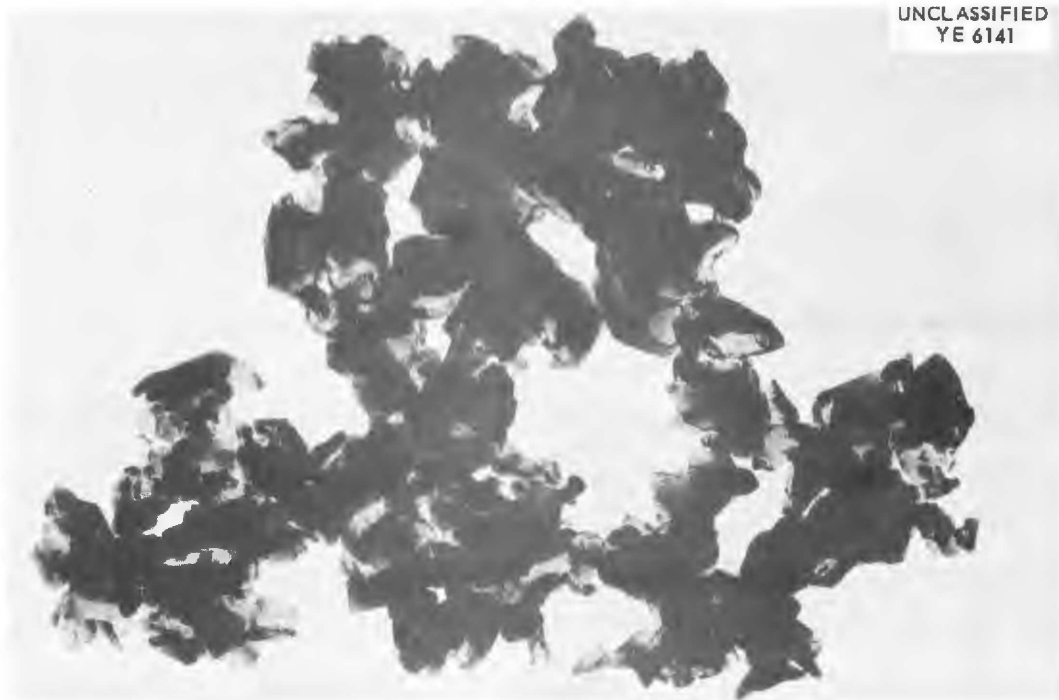
Fig. 6.5. BeO Powder made by Calcining \text{BeSO}_4 \cdot \text{XH}_2\text{O} . 22,700X.
