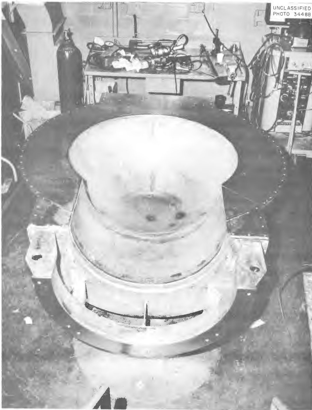
Fig. 12.8. One of the Large Outer Sections of Pratt & Whitney Shield.
