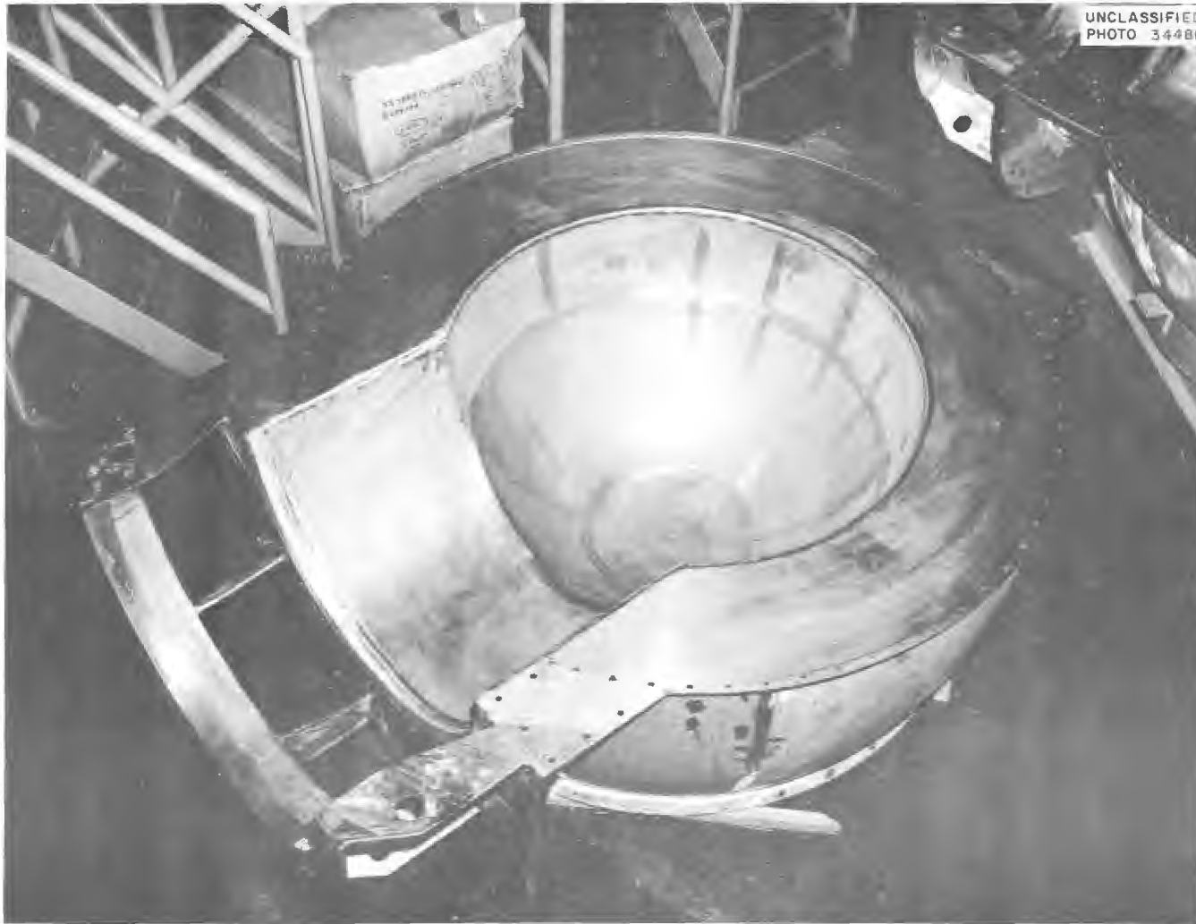
Fig. 12.9. One of the Large Outer Sections of Pratt & Whitney Shield.
