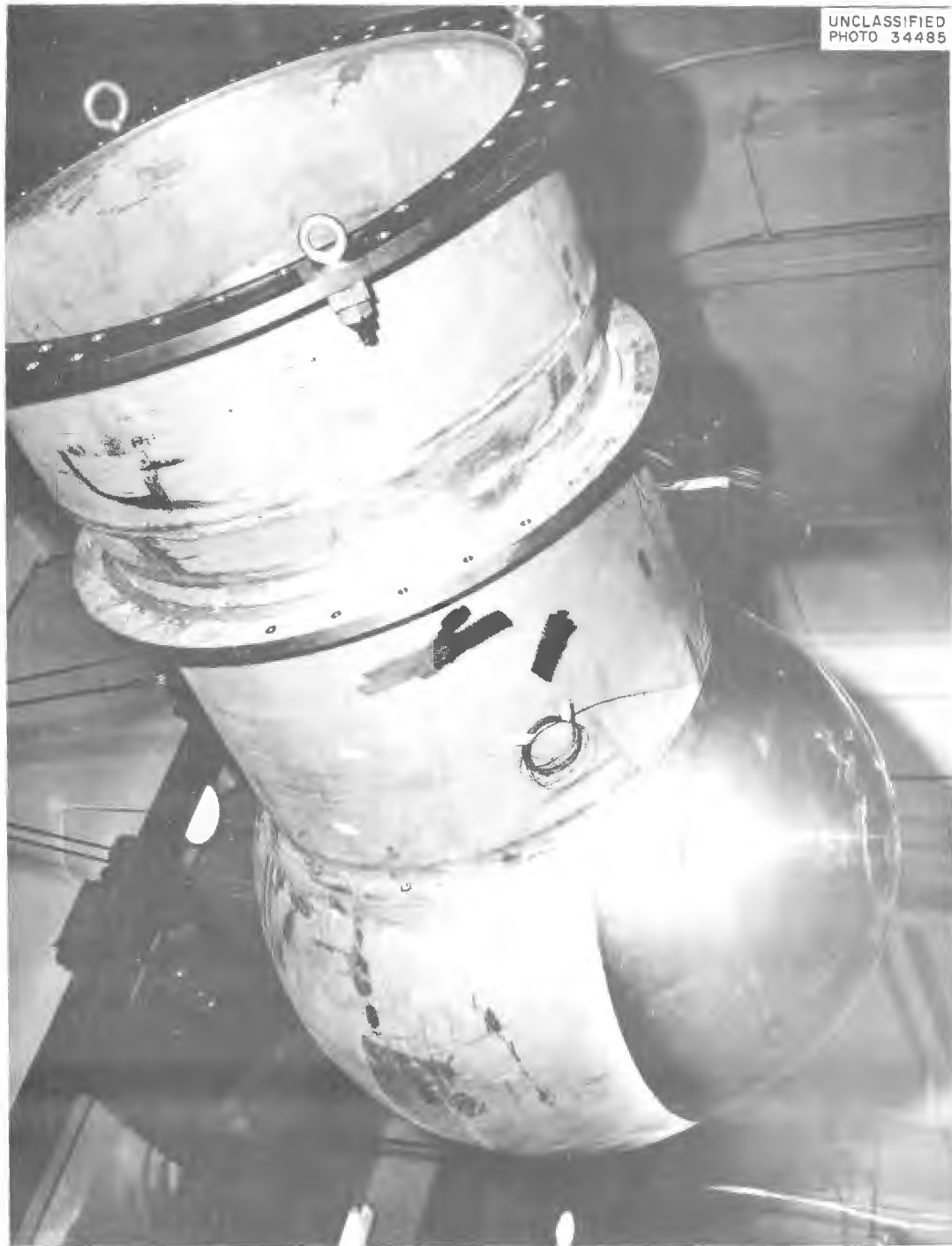
Fig. 12.7. Inner Section of Pratt & Whitney Shield Showing Depleted Uranium Shadow Shield Bolted on the Outside.
