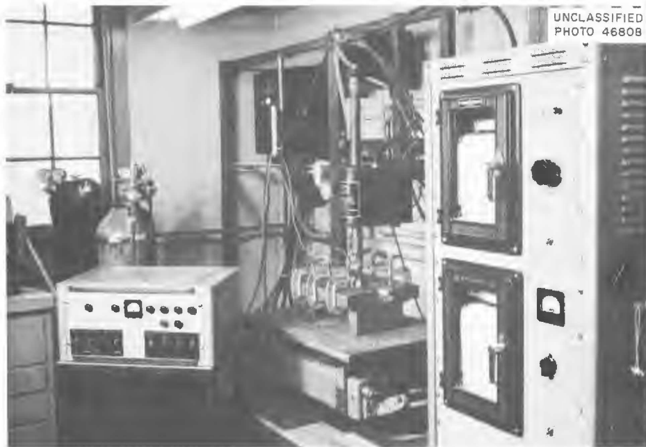
Fig. 3.1. Setup Used for Automatic Inert-Gas-Shielded Tungsten-Arc Welding.
