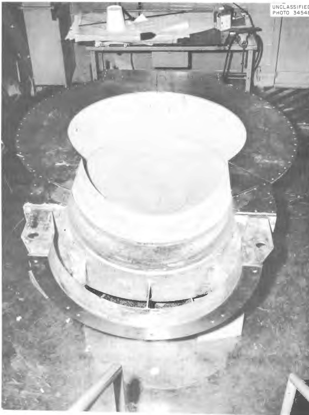
Fig. 12.10. Outer Section of Pratt & Whitney Shield Showing Layers of Lithium Hydride Blocks.
