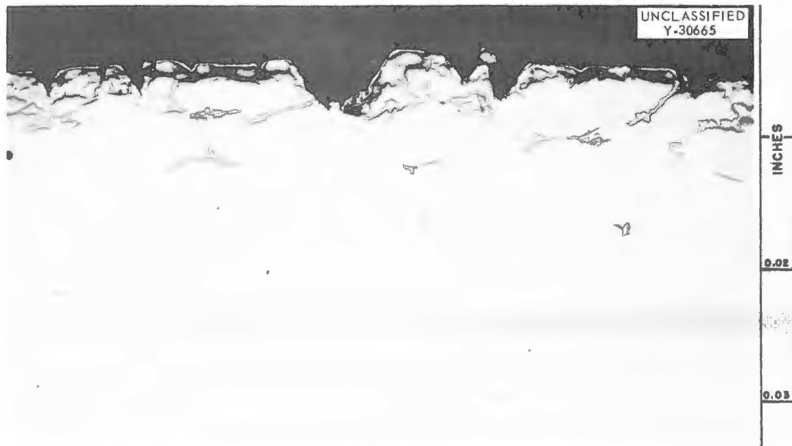
Fig. 4.2. Photomicrograph of Edge of Columbian Specimen 190 After Testing in Nitrogen at 3500 psi and 1850°F. Duration of test was 2321 hr. Etchant: H_2O-HF-HNO_3-H_2SO_4 . 100X.
