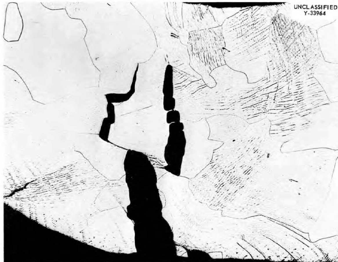
Fig. 2.7. Photomicrograph of a Crack Shown in Fig. 2.6. Both transgranular and intergranular cracks are evident. Etchant: \text{HNO}_3 , \text{H}_2\text{SO}_4 , \text{HF} , \text{H}_2\text{O} . 50X.
