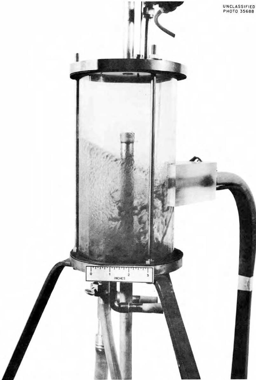
Fig. 6.9. Liquid-Vapor Separator in Operation with an Air-Water Mixture.
