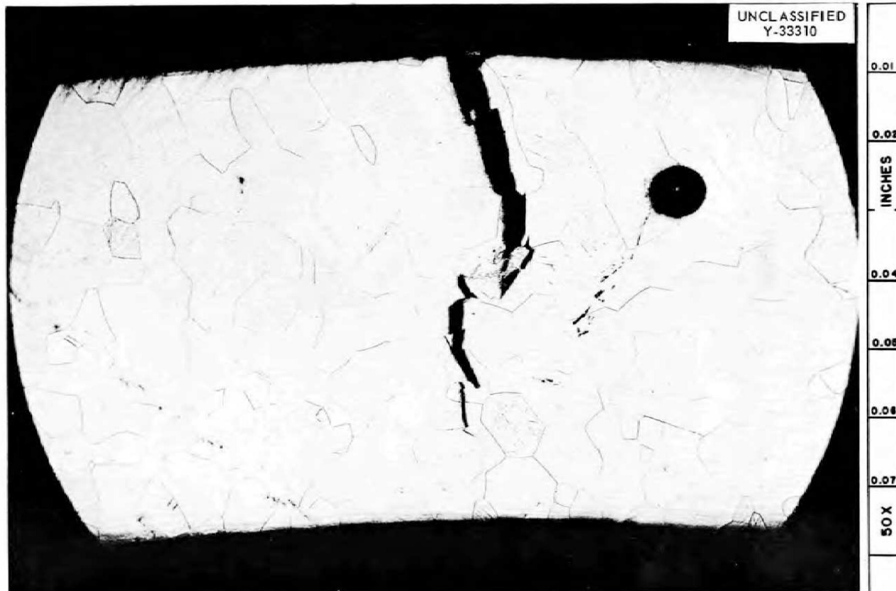
Fig. 2.8. Photomicrograph of a Crack in a Brittle Cb-1% Zr Alloy Weld. The cracking appears to be primarily transgranular. Etchant: \text{HNO}_3 , \text{H}_2\text{SO}_4 , \text{HF} , \text{H}_2\text{O} . 50X.
