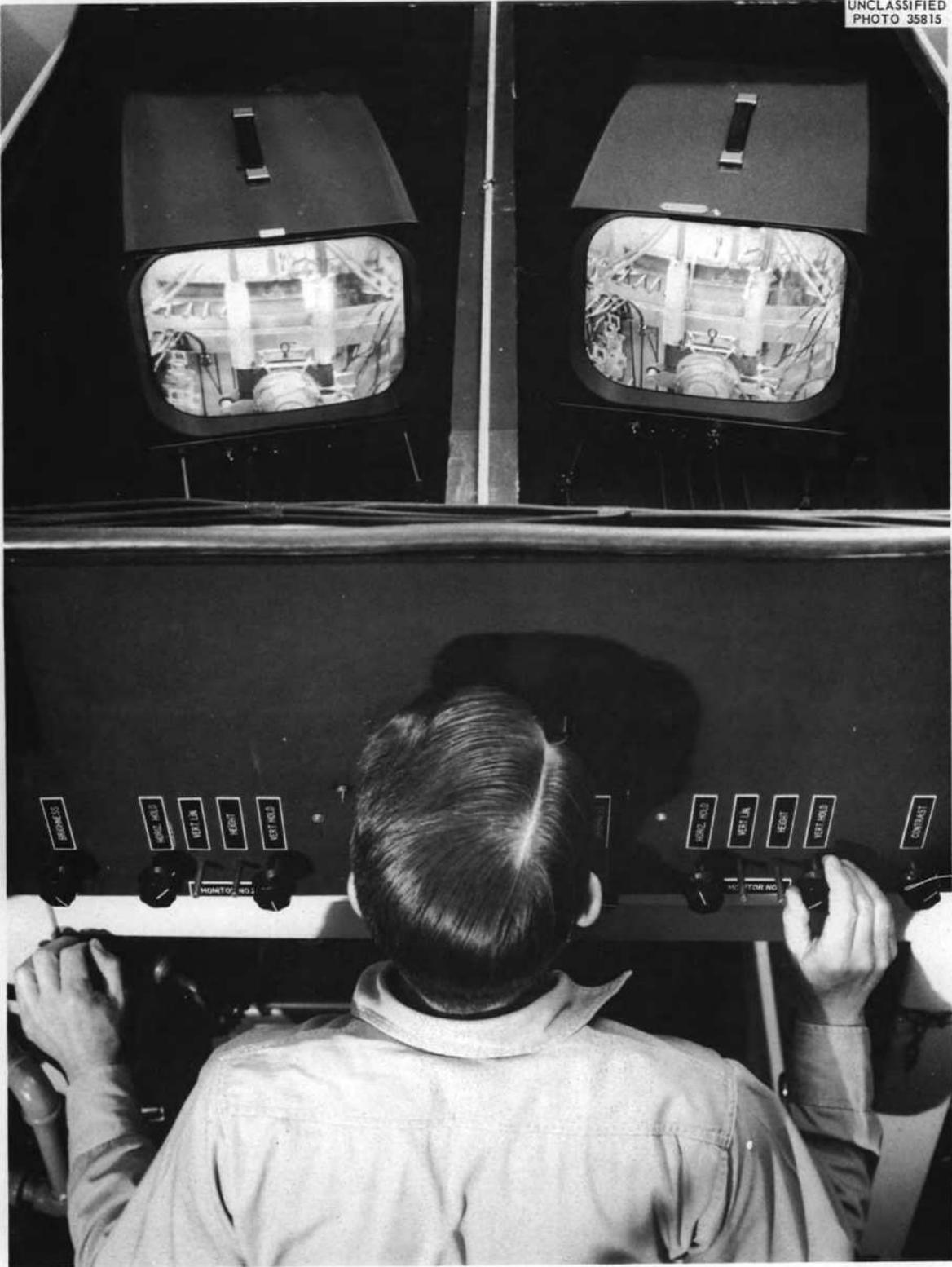
Fig. 1.1.3. Closed-Circuit-Television Stereo Viewer.
