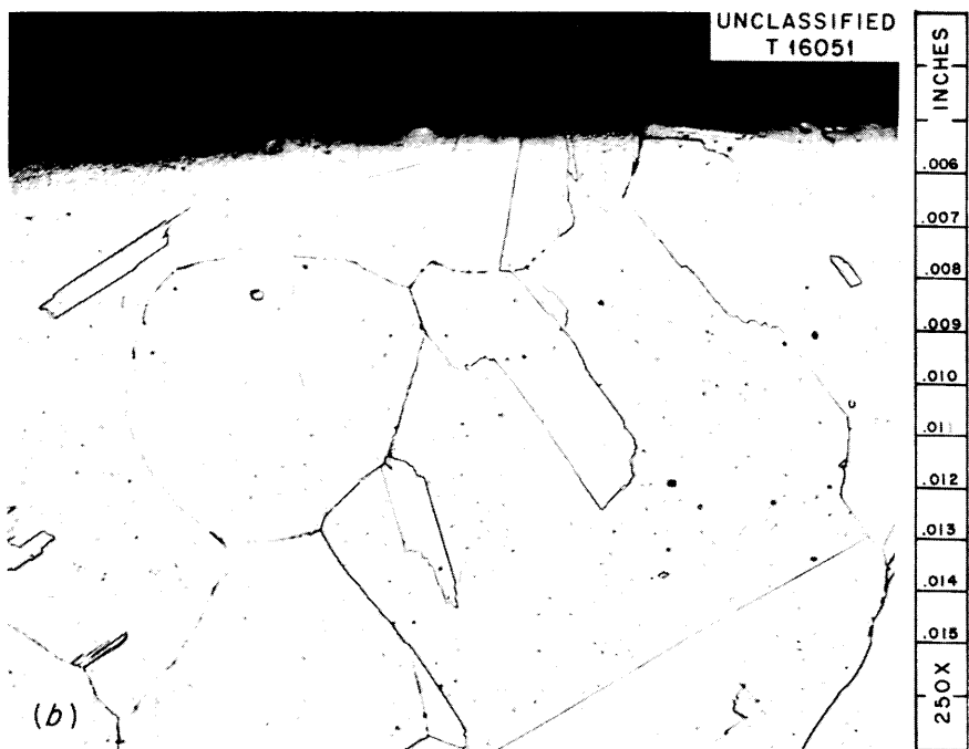
Fig. 3. Photomicrographs of Annealed and Unannealed Inconel Specimens. (a) Specimen unannealed (point A, Fig. 2); D = 78 \times 10^{-15} \text{ cm}^2/\text{sec.} (b) Specimen annealed at 1150^\circ\text{C} for 4 hr; D = 1.7 \times 10^{-15} \text{ cm}^2/\text{sec.} T_{\text{salt}} = 675^\circ\text{C} for both experiments.
