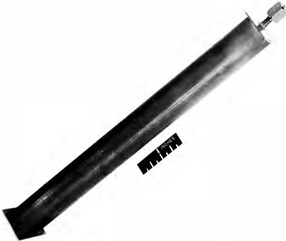
Fig. 4.5. Rig for Testing Graphite-to-Metal Joints.
