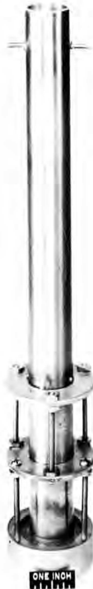
Fig. 4.2. Test Rig with Sump-Type Seal.
