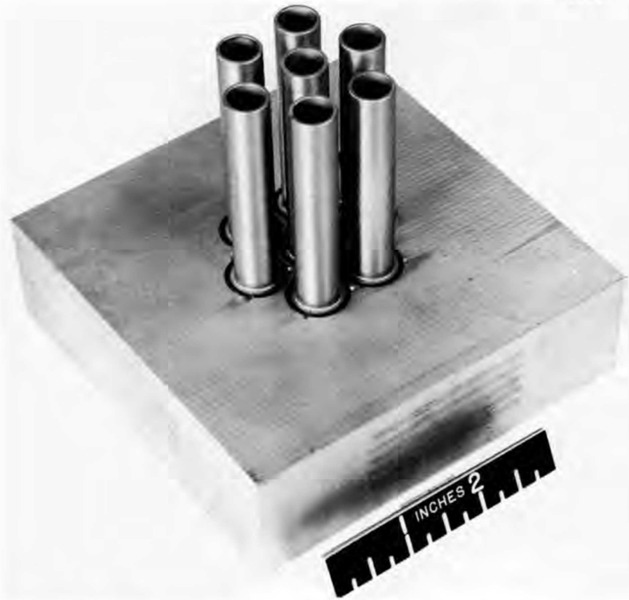
Fig. 4.7. Tube-to-Tube-Sheet Sample, Showing Back Brazing.
