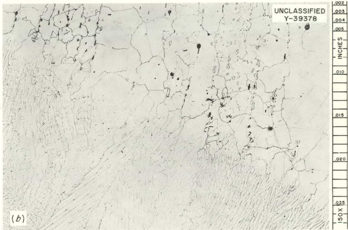
Fig. 4.4. (a) Side-Bend Specimen Made with Niobium-Modified Weld Metal Showing Good Weld-Metal Soundness. (b) Photomicrograph Showing Excellent Weld-Metal Quality. Etchant: 3 parts HCl, 2 parts H 2 O, 1 part 10% chromic acid.
