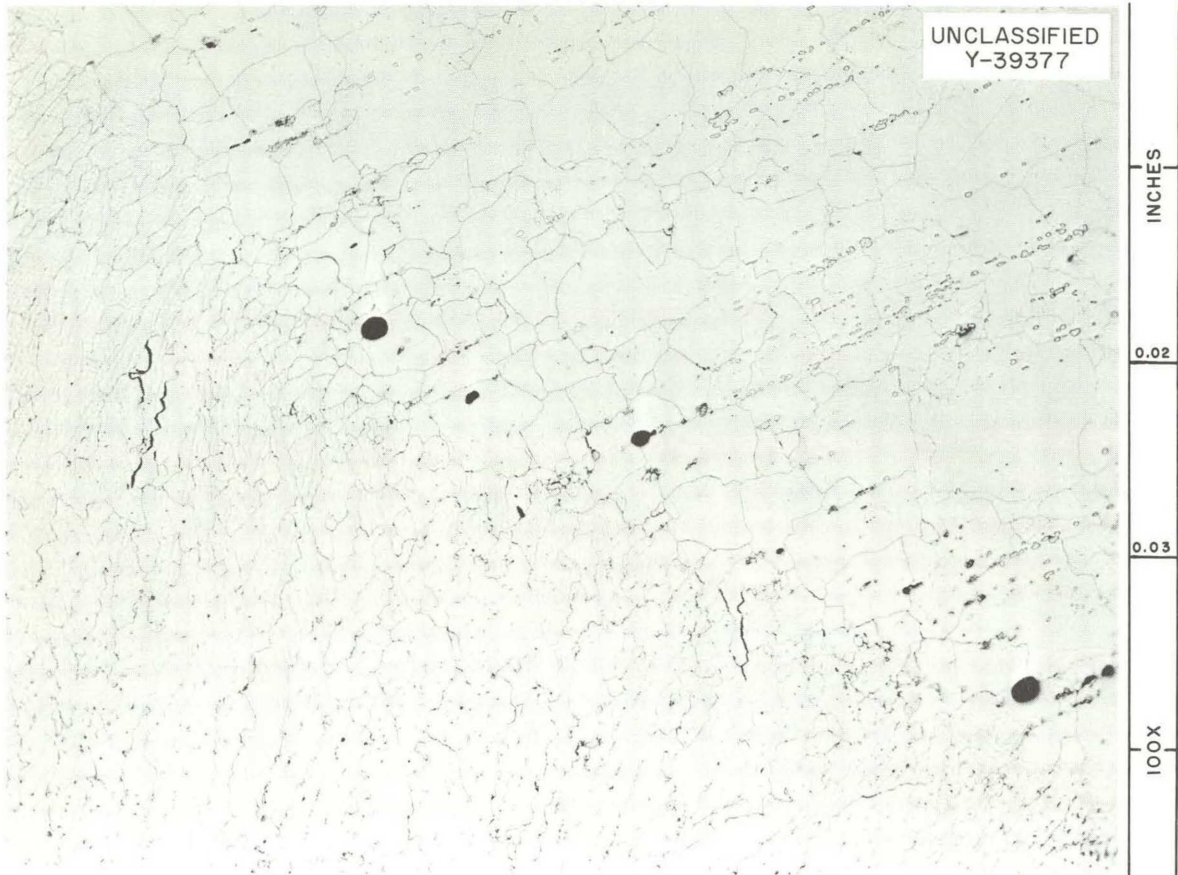
Fig. 4.3. Photomicrograph of Welded Joint Showing Fusion-Line Porosity and Microfissures and Weld-Metal Crack. Etchant: 3 parts HCl, 2 parts H 2 O, 1 part 10% chromic acid.
