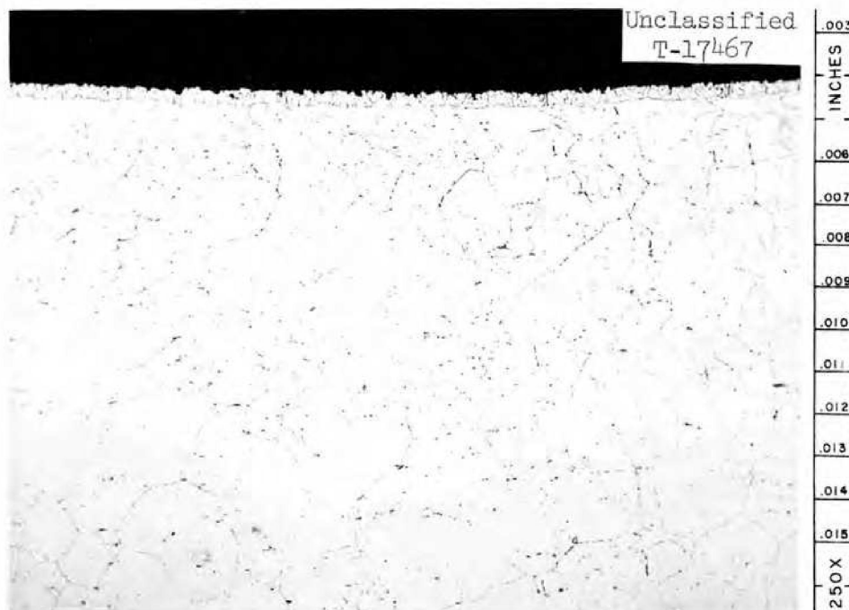
Fig. 9. Appearance of Specimen Removed from End of the Second Heater Leg. Etchant: 3 parts HCl, 2 parts H 2 O, 1 part 10% Chromic acid. 250X
