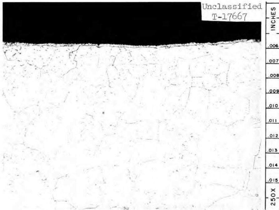
Fig. 8. Appearance of Specimen Removed from End of the First Heater Leg. Etchant: 3 parts HCl, 2 parts H 2 O, 1 part 10% Chromic acid. 250X
