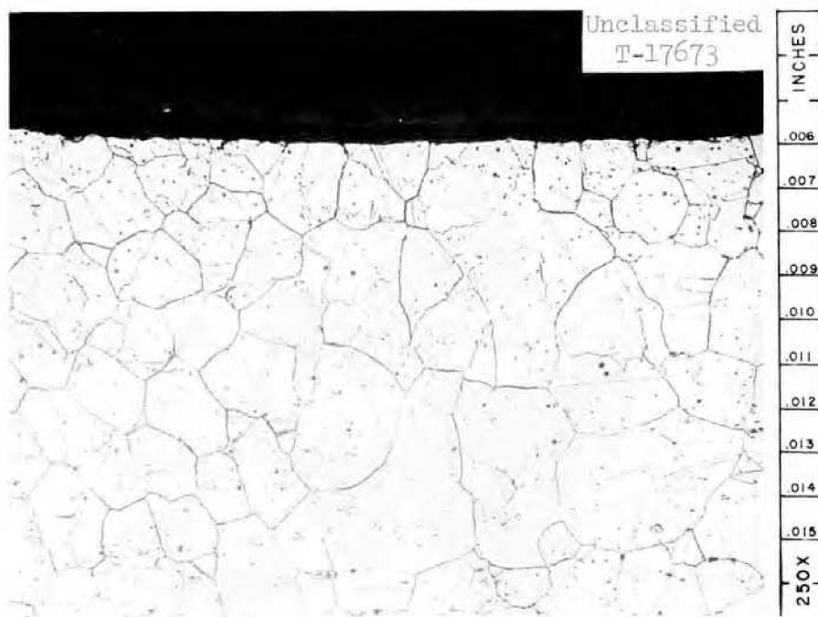
Fig. 10. General Appearance of Cooler Coil. Etchant: 3 parts HCl, 2 parts H 2 O, 1 part 10% Chromic acid. 250X
