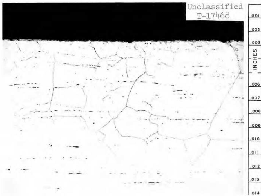
Fig. 11. Specimen Removed from Top of Box Containing Graphite Rods. Etchant: 3 parts HCl, 2 parts H 2 O, 1 part 10% Chromic acid. 250X
