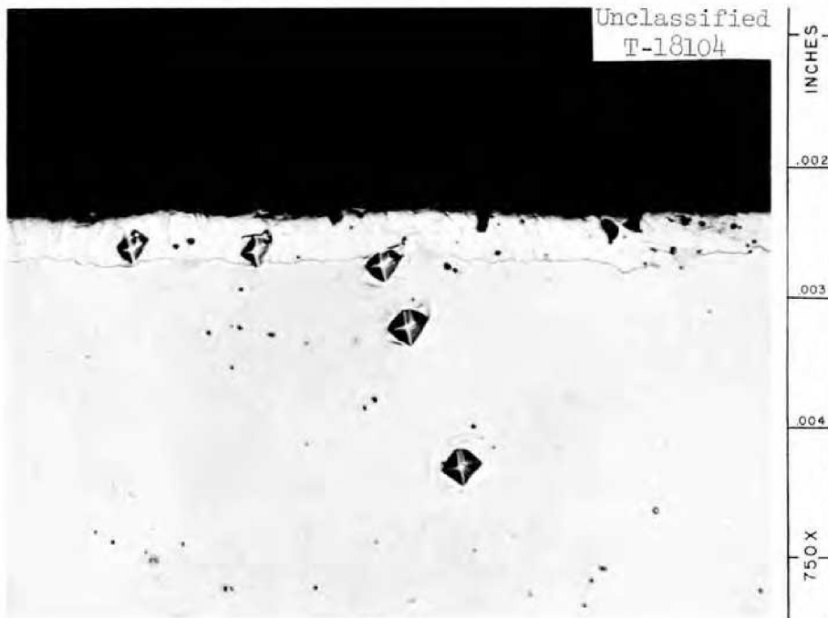
Fig. 14. Microhardness Measurements Made on Specimen Removed from Second Heater Leg. Etchant: None. 750X.
