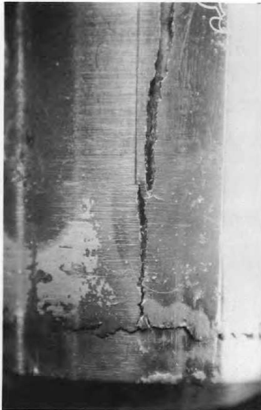
Fig. 8.9. Ruptured Cladding of Capsule 5-7. 4X
