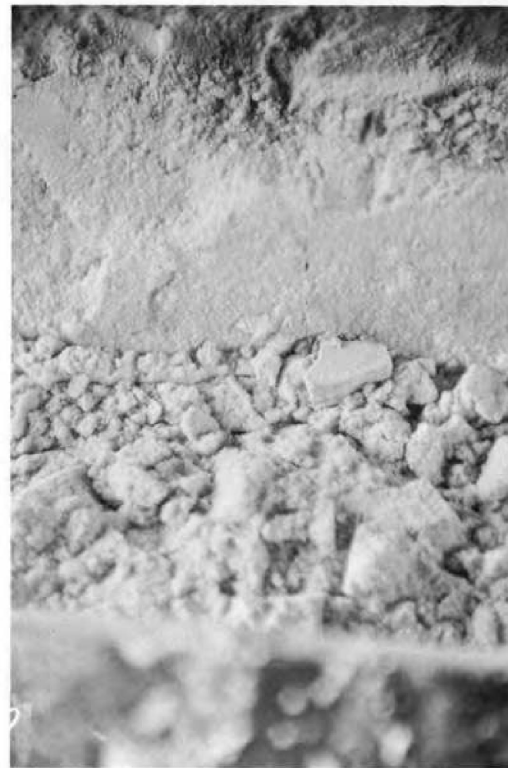
Fig. 8.8. Disintegrated and Fractured Material from BeO Irradiation Capsule 5-7 After a Fast-Neutron Dose of 1 \times 10^{21} Neutrons/cm 2 at 120°C. 4X
