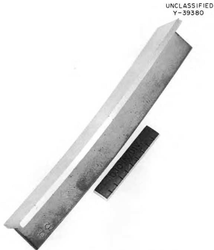
Fig. 5.2. Columbium-to-Stainless Steel Brazed Joint Showing Distortion Resulting from Difference in Thermal-Expansion Coefficients of the Two Materials.
