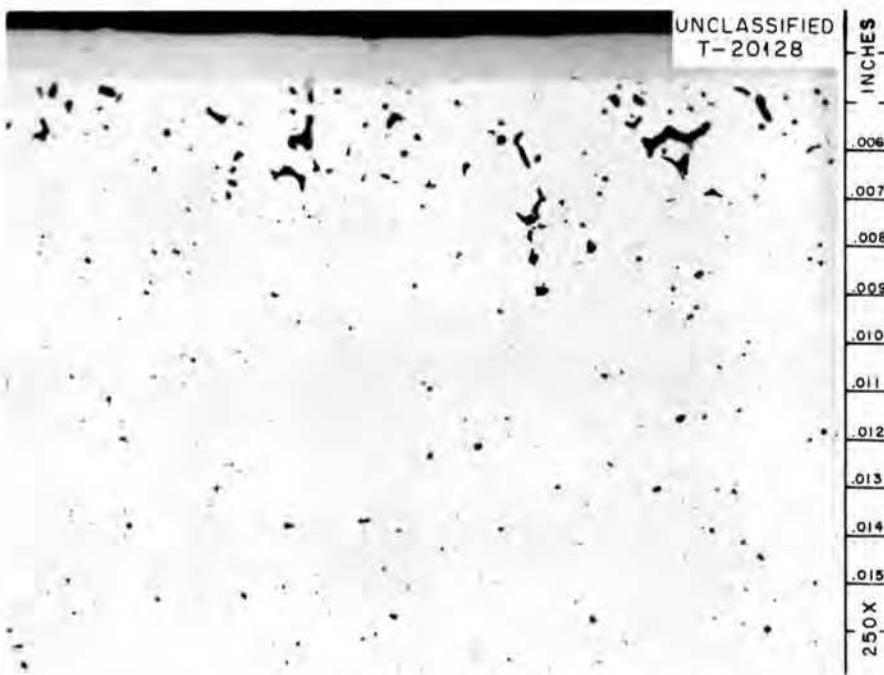
Fig. 4.3. Appearance of Specimen Removed from Point of Maximum Salt-Metal Interface Temperature Region (1500°F) of INOR-8 Forced-Convection Loop MSRP-16. The loop was operated for 20,000 hr.
