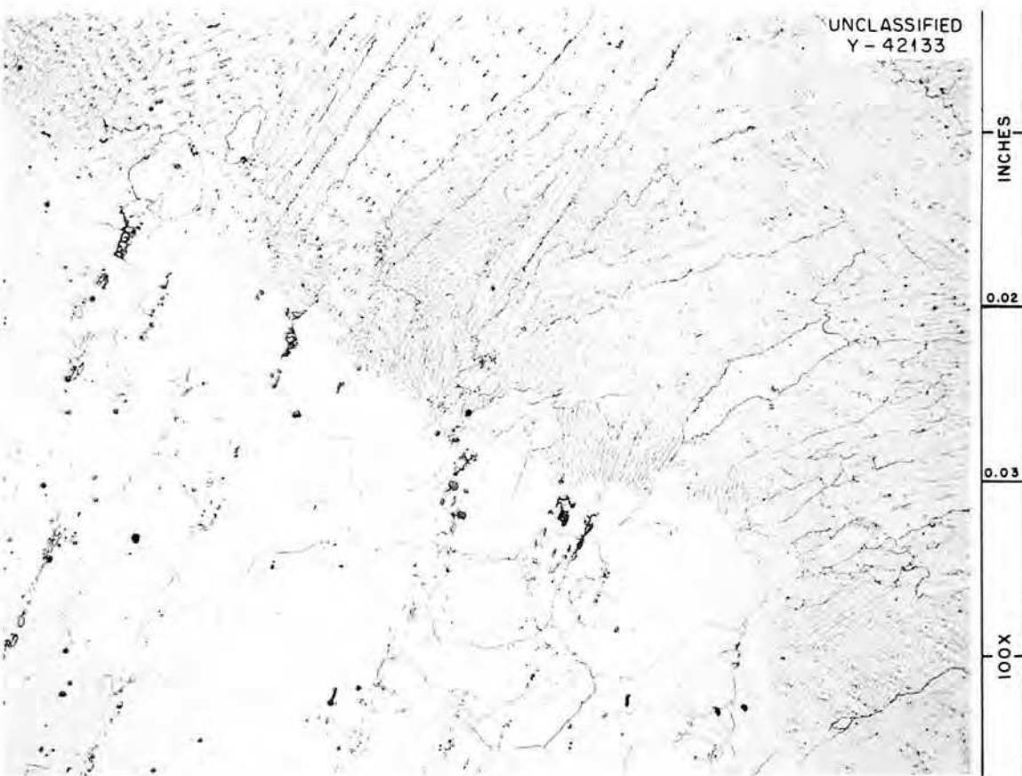
Fig. 4.9. Fusion-Line Area of Weld No. Y-8488-W1. No cracks or porosity is evident. Etchant: CrO<sub>3</sub>-H<sub>2</sub>O-HCl.
