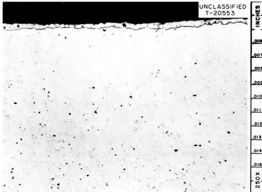
Fig. 4.1. Appearance of Specimen Removed from Point of Maximum Salt-Metal Interface Temperature Region (1300°F) of INOR-8 Forced-Convection Loop MSRP-10. The loop was operated for 20,000 hr.
