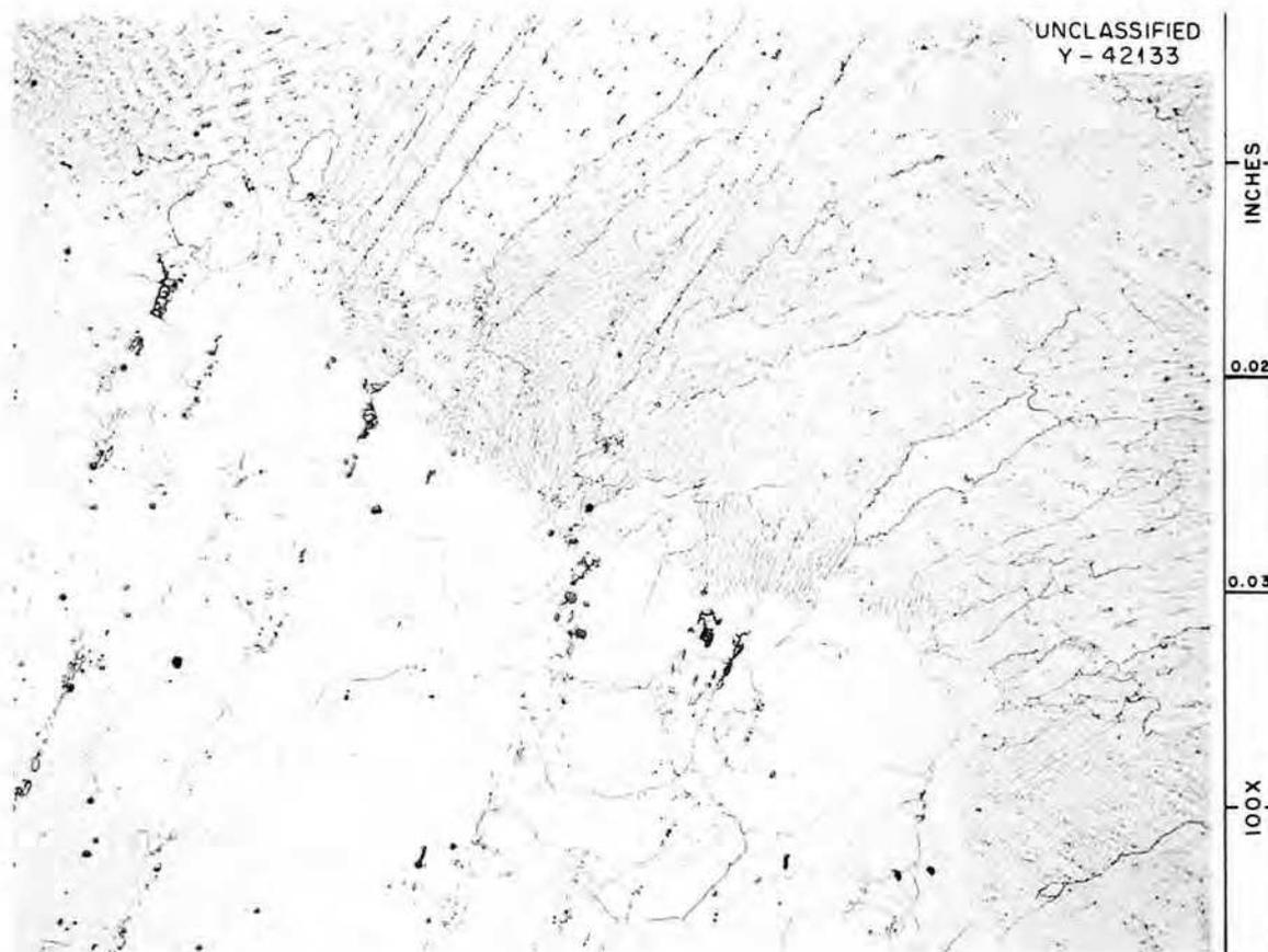
Fig. 4.9. Fusion-Line Area of Weld No. Y-8488-W1. No cracks or porosity is evident. Etchant:  $\text{CrO}_3\text{-H}_2\text{O-HCl}$ .
