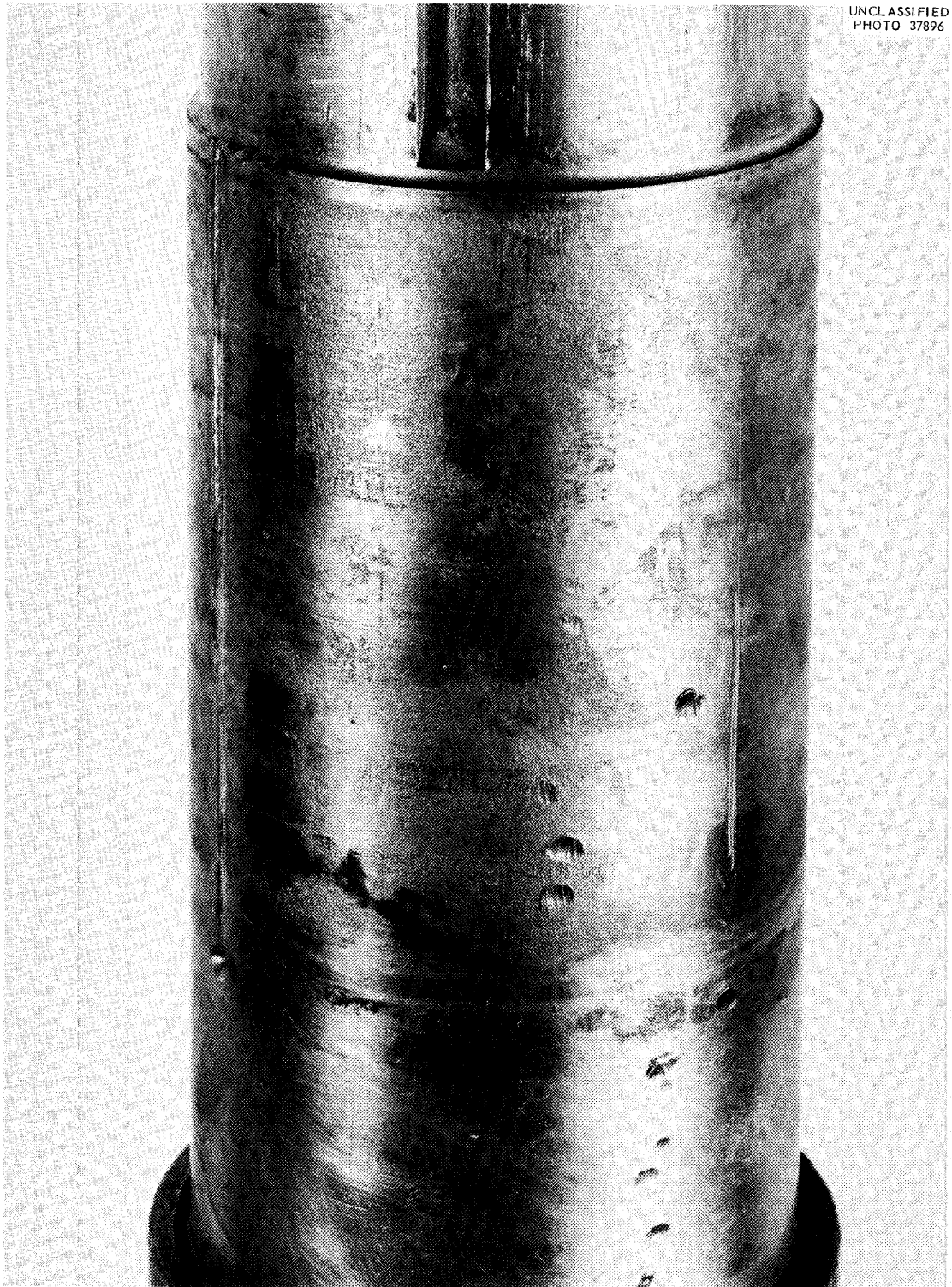
Fig. 2.32. Self-Welding Between Inconel Shaft and INOR-8.
