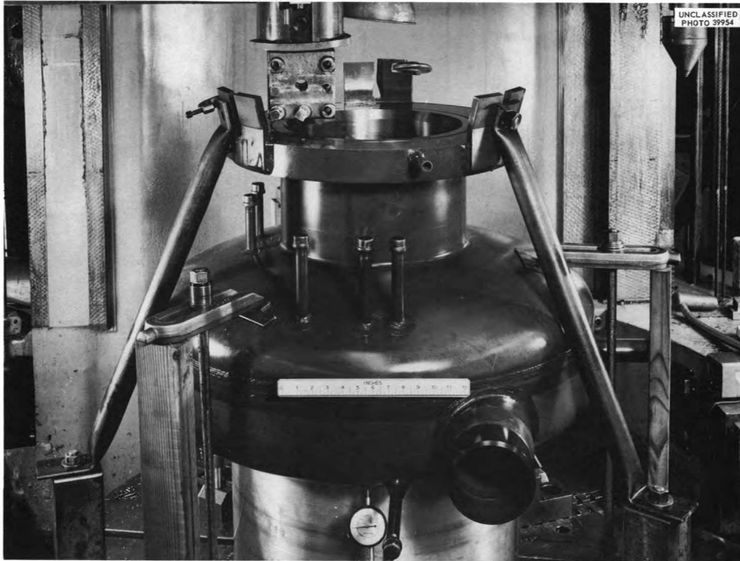
Fig. 1.5. MSRE Coolant Pump Bowl After Final Machining.
