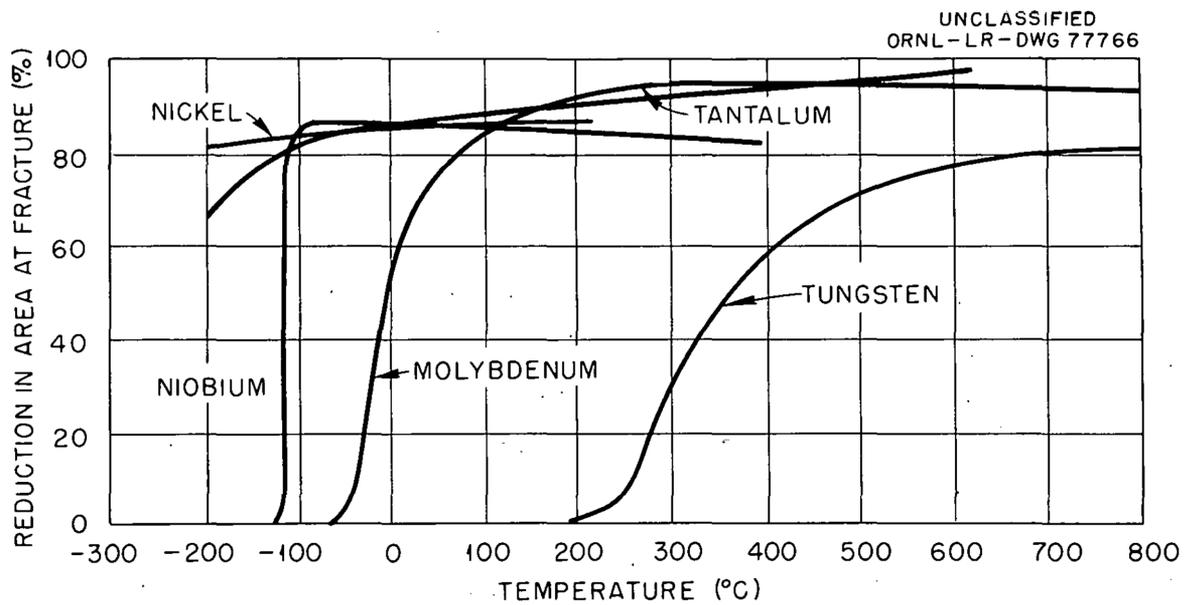
Fig. 1. Effect of Temperature on Ductility. [L. Northcott, "Some Features of the Refractory Metals," p. 8, Niobium, Tantalum, Molybdenum, and Tungsten, (ed. by A. G. Quarrell) Elsevier Publishing Co., New York, 1961.]
