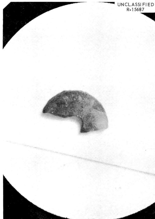
Fig. 5.9. Portion of Graphite Wafer Broken from Core During Disassembly of Capsule 2.
