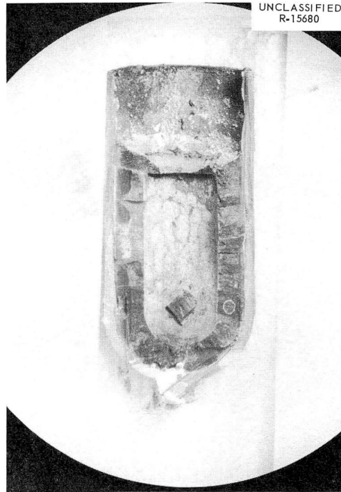
Fig. 5.15. Capsule 4. Other Half, Showing Shiny Film on Fuel and a Wetting Meniscus.
