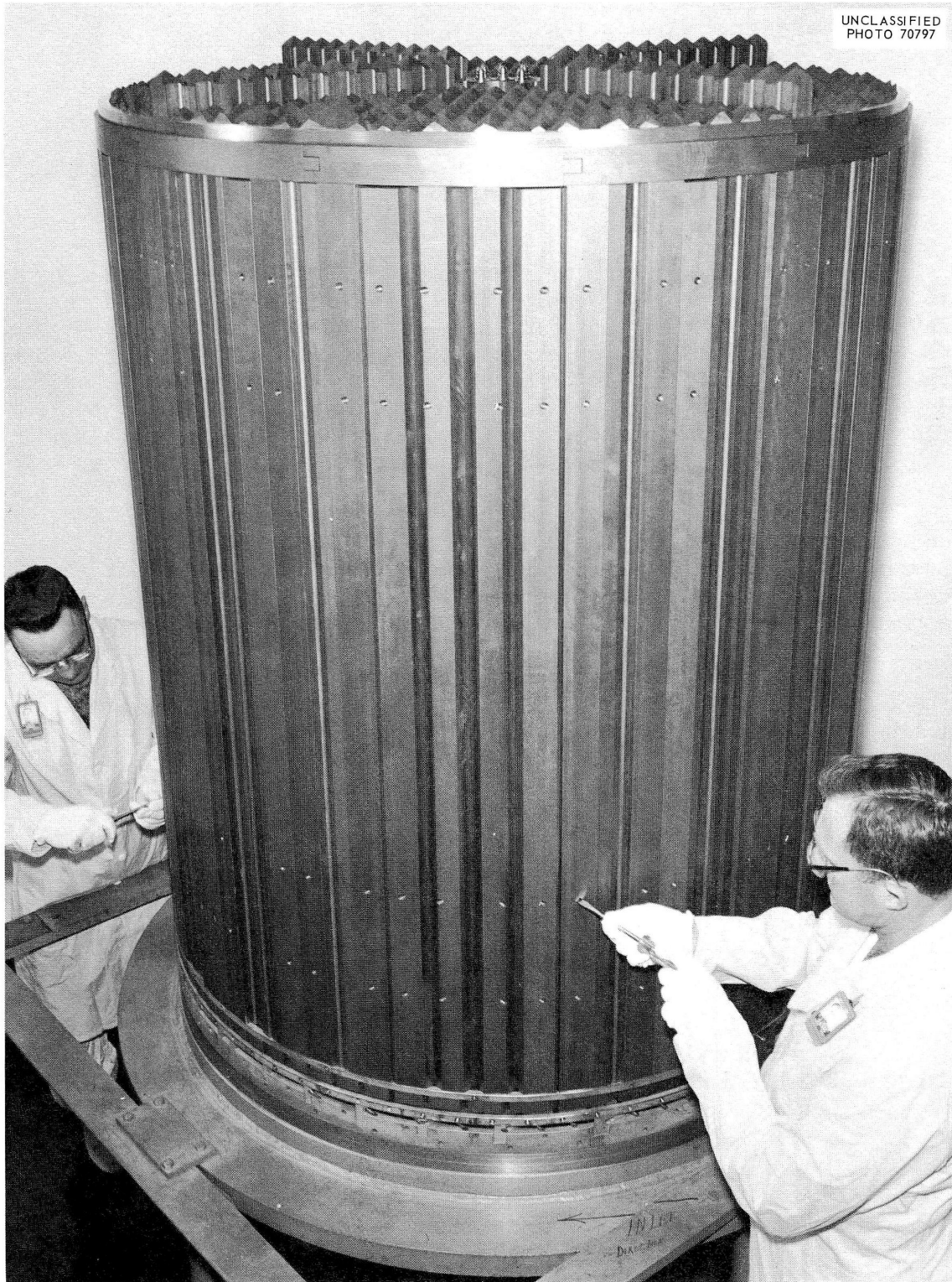
Fig. 1.1. Assembly of the MSRE Graphite Core.
