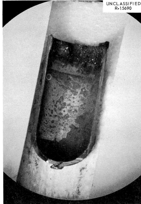
Fig. 5.5. Capsule 1. Other Half of INOR-8 Wall, Showing Salt Splotches Between Graphite and INOR-8.
