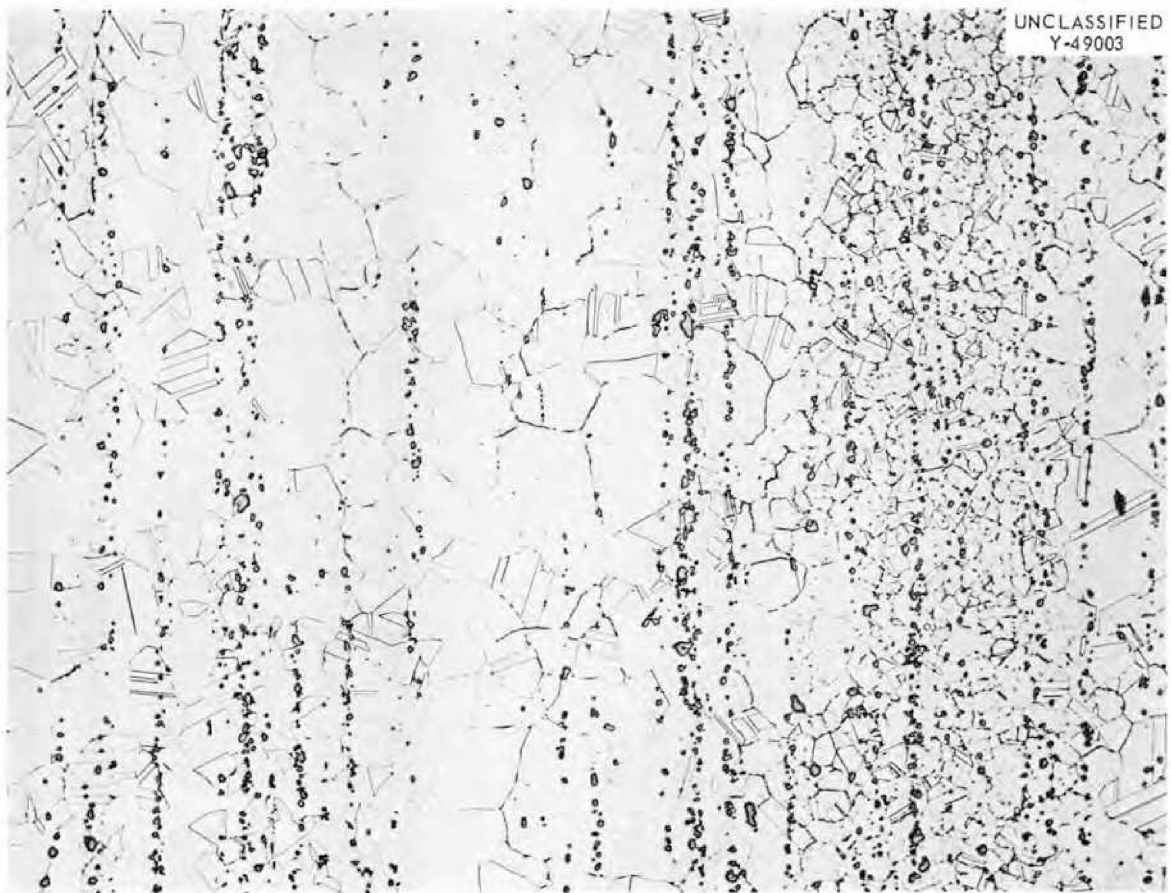
Fig. 6. Photomicrograph of Hastelloy N Annealed 1 hr at 2200°F in Argon and Rapidly Cooled. Heat 5075. Hardness (DPH) average 185; range 174-213. Etched in glyceric acid. 100X
