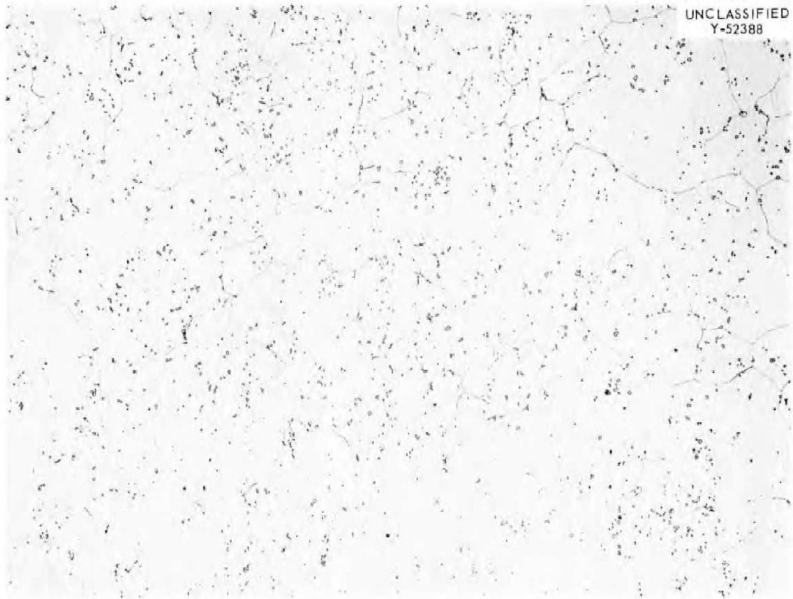
Fig. 12. Photomicrograph of Hastelloy N Annealed 1 hr at 2200°F in Argon and Rapidly Cooled. Heat 2477. Etched in glyceric regia. 100×
