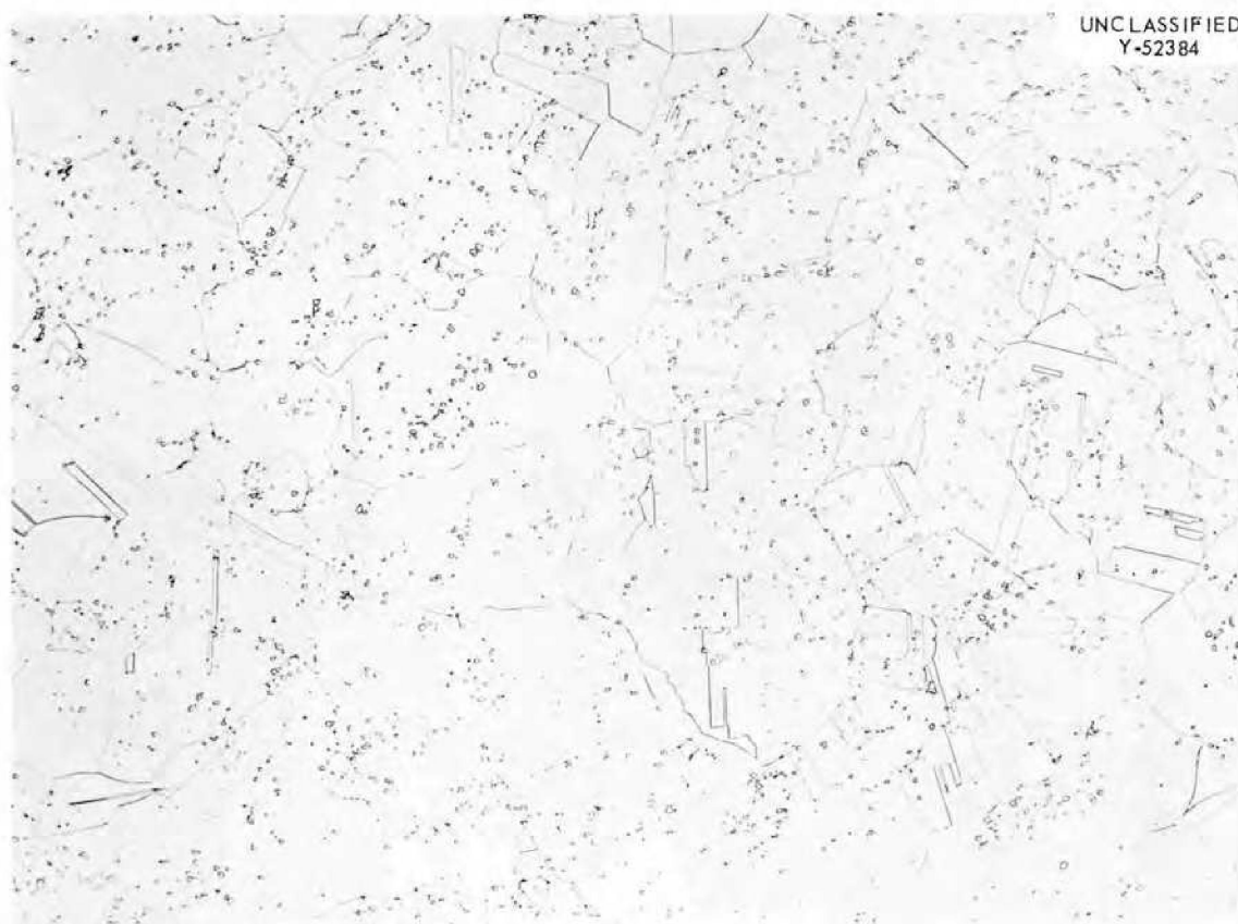
Fig. 11. Photomicrograph of Hastelloy N Annealed 1 hr at 2150°F in Argon and Rapidly Cooled. Heat 2477. Etched in glyceria regia. 100X
