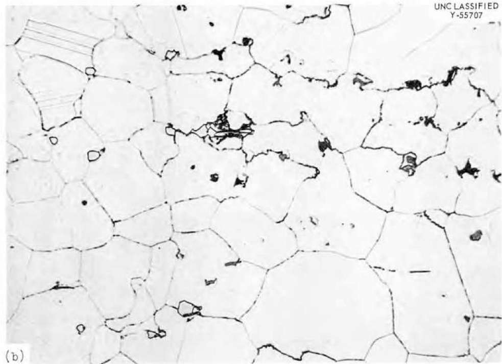
Fig. 35. Hastelloy N Wire Melted on One End. Heat 5075. Etched in glyceria regia. (a) 100X, (b) 500X. Reduced 15%.
