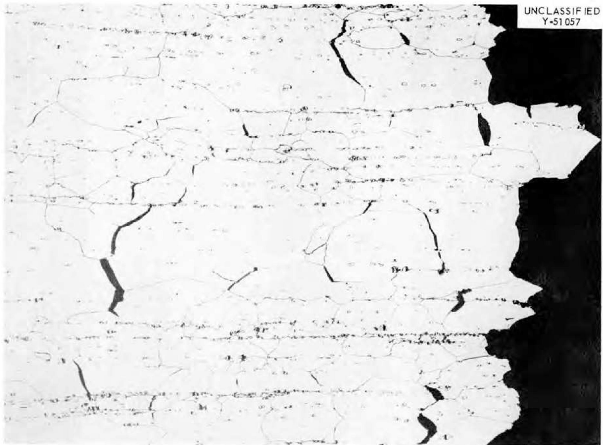
Fig. 28. Fracture of Hastelloy N Specimen Tested at 1600°F, Annealed 1 hr at 2300°F, and Strained 20% at 75°F Prior to Testing. Heat 5075. Etched in glyceria regia. 100X
