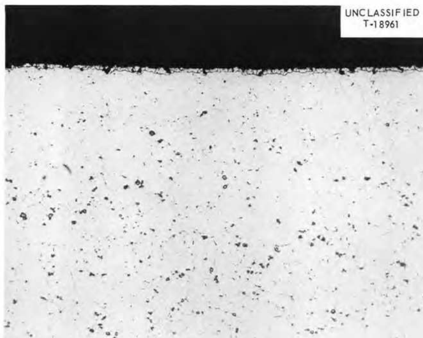
Fig. 2. Typical Appearance of Metallographic Specimen at Hot Leg of INOR-8 Thermal-Convection Loop in Phase II Tests.
