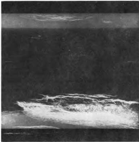
Fig. 5. GCB Graphite Specimens Impregnated with Molten Salt at 50 psig. (a,b,c) As-radiographed and (d) after 100 thermal cycles.
