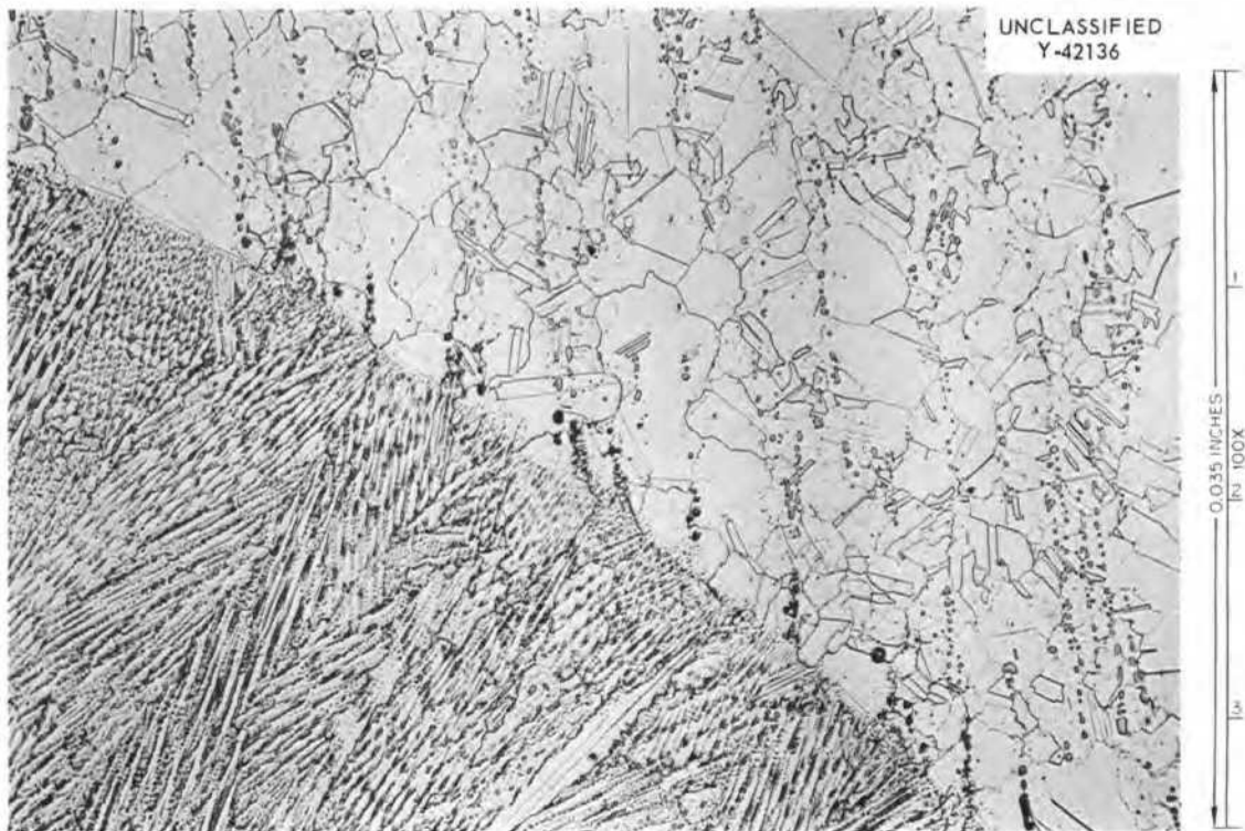
Fig. 24. Weld Metal Structure of Heat 5055 of INOR-8, Showing No Cracking.
