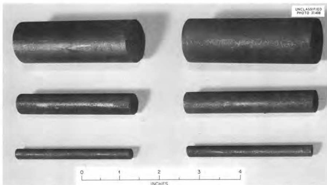
Fig. 20. Graphite Specimens After Exposure to Molten Fluoride.
