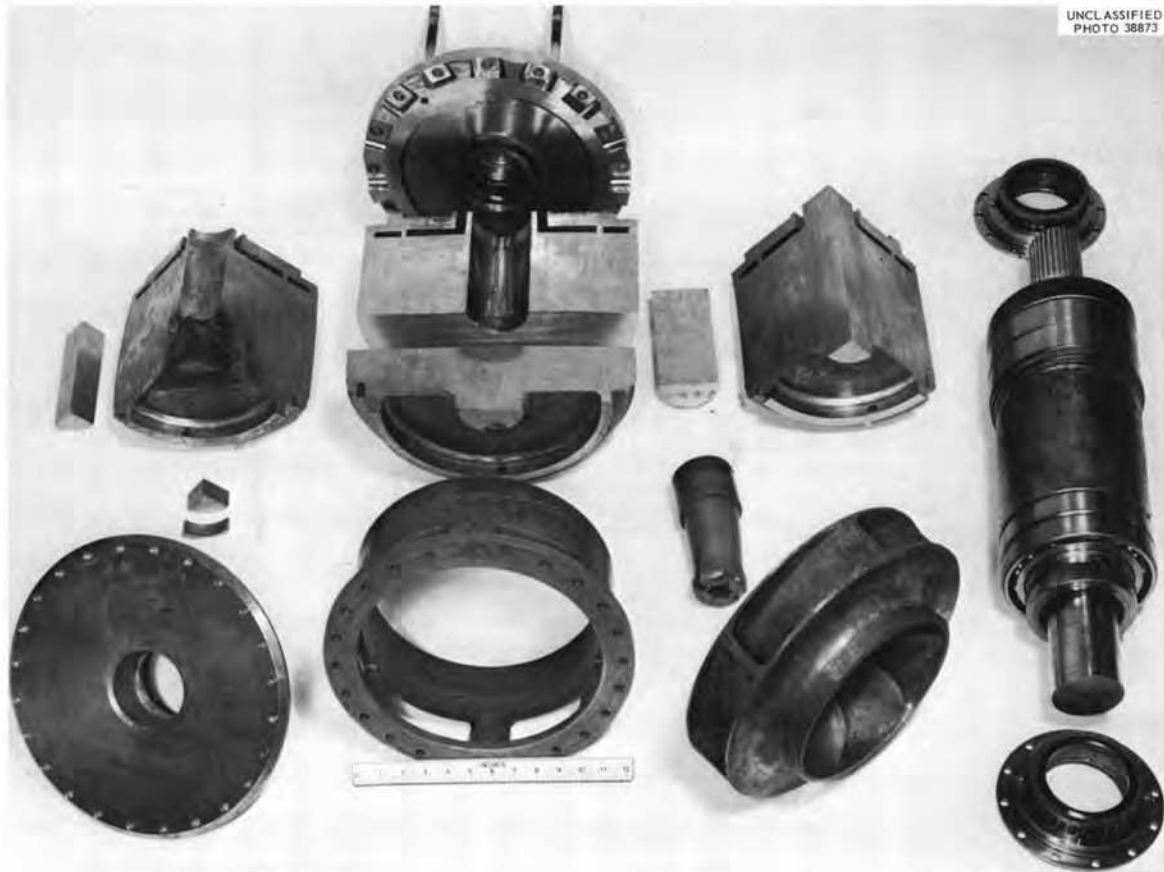
Fig. 15. Results of MSRE Prototype Pump Shaft Seizure.
