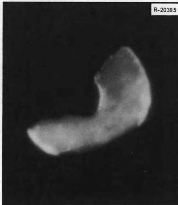
Fig. 5.11. Autoradiograph of Transverse Section of Capsule 2 Graphite Wafer.
