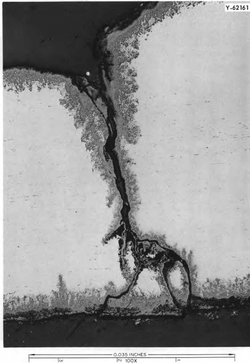
Fig. 4.10. Crack Through Transverse Section of INOR-8 Tube from Drain Tank Cooler Test.
