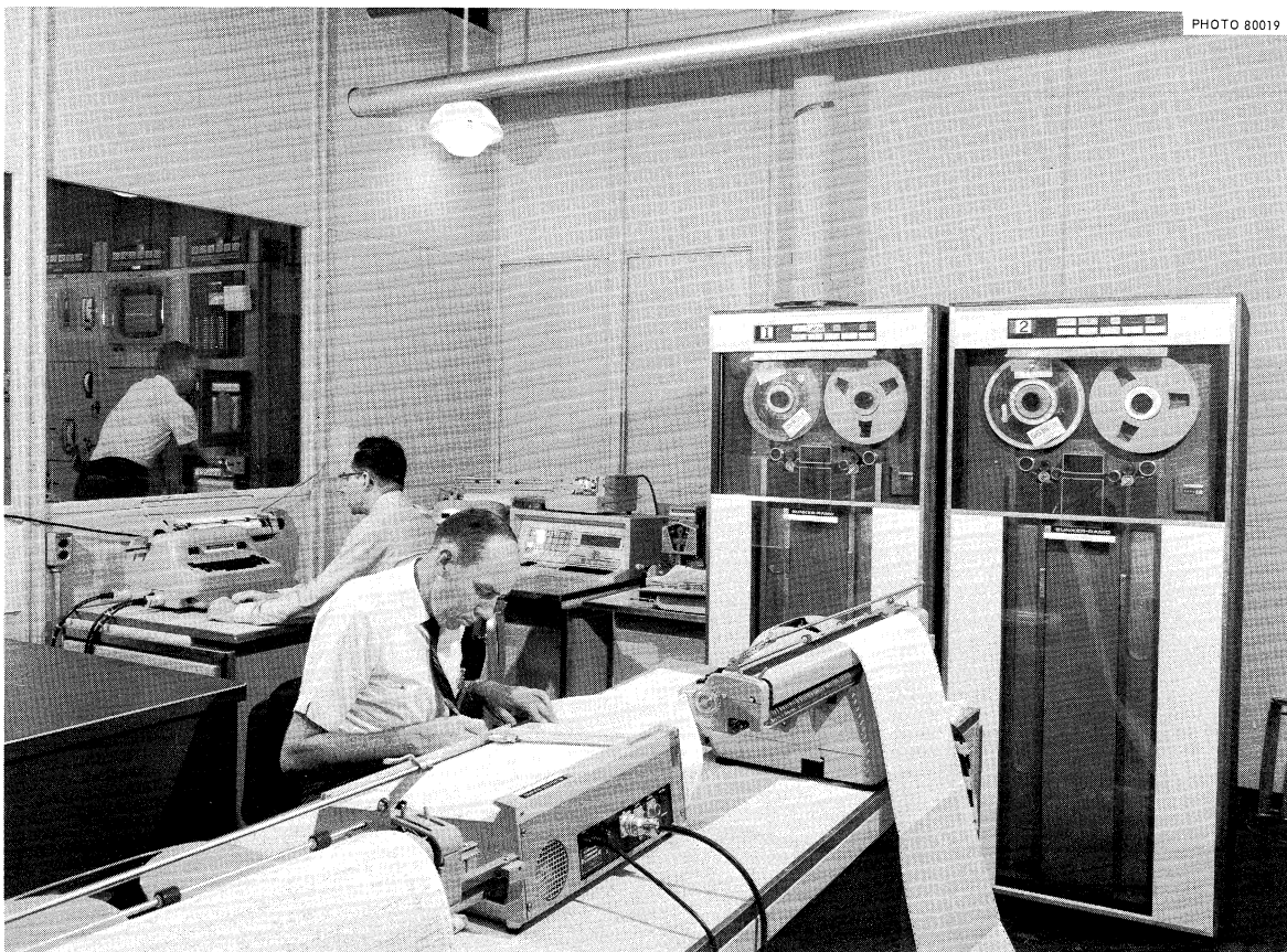
Fig. 1.19. MSRE Computer-Data-Logger System Console, Typewriters, and Tape Units.
