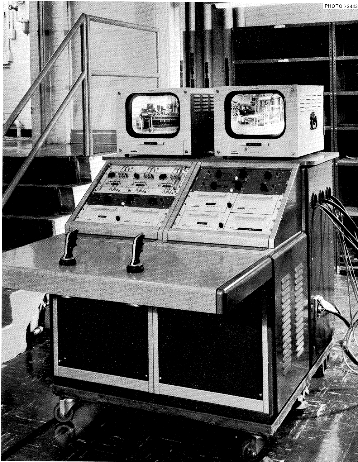
Fig. 1.17. Remote Maintenance Television Control Console.
