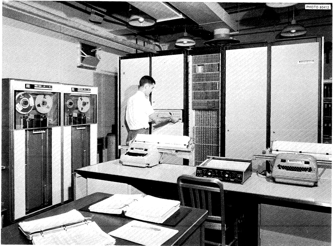
Fig. 1.20. Computer, Typewriters, and Tape Units of the MSRE Computer-Data-Logger System.
