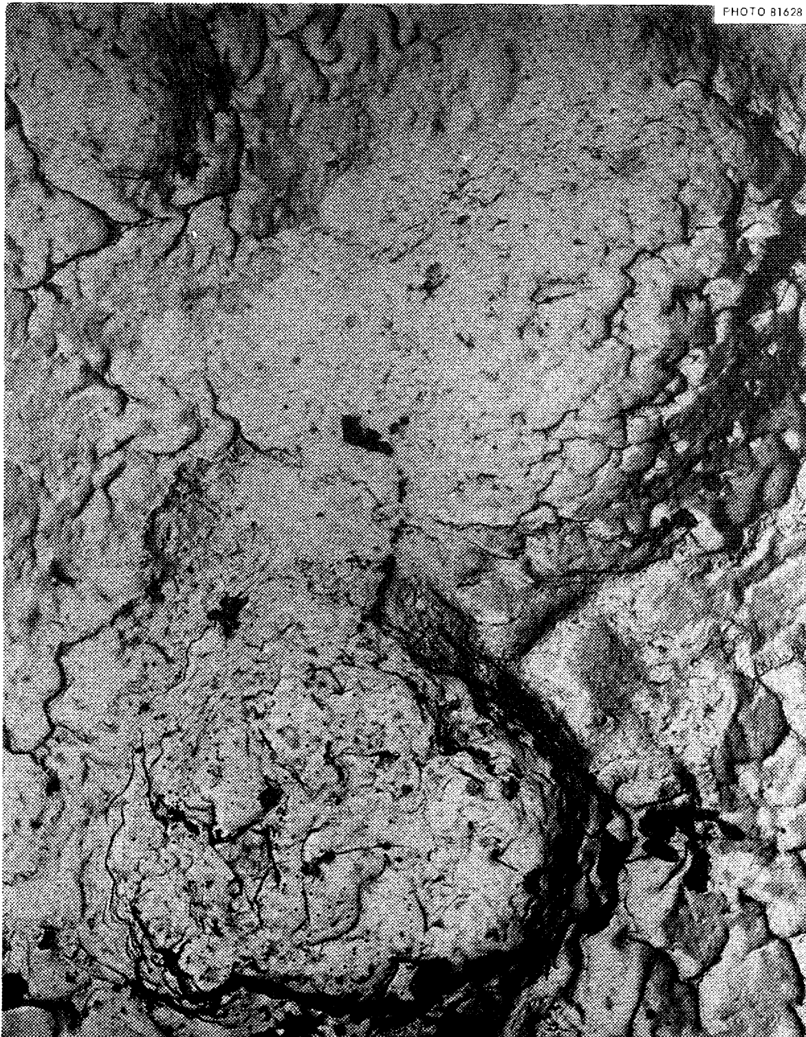
Fig. 12.2. Electron Micrograph of MgO of Density 3.4 \text{ g/cm}^3 and Grain Size 10 \mu Irradiated to a Fast-Neutron Dose of 1.2 \times 10^{21} \text{ Neutrons/cm}^2 ( >1 \text{ Mev} ) at 150^\circ\text{C} at 32,000\times Magnification Showing General Deterioration and Small Cracks. Reduced 12.5%.
