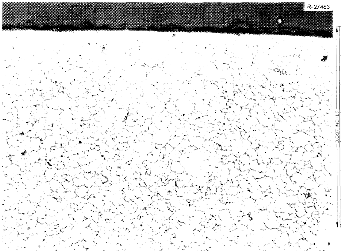
Fig. 4.4. Microstructure of Control Hastelloy N Tensile Specimen. Although the microstructure is extremely fine grained, the specimen is coarser grained than the one removed from the MSRE.
