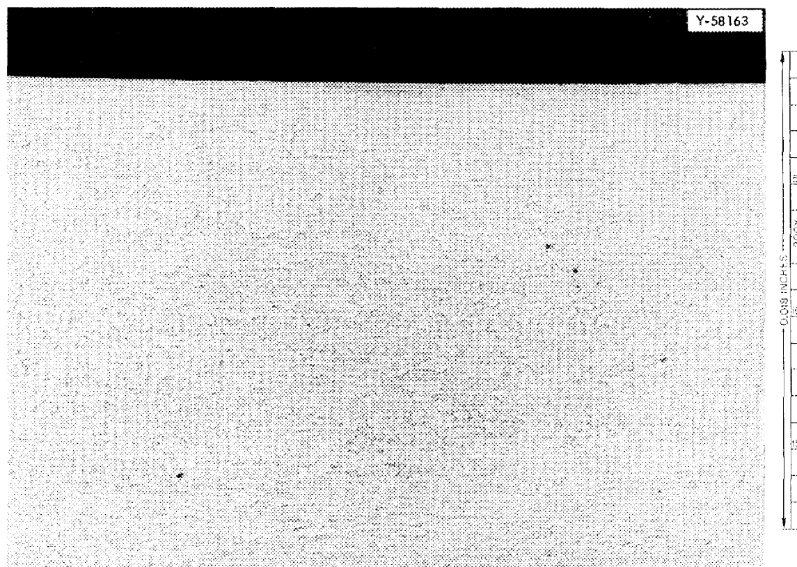
Fig. 4.1. Section Through the Hot Leg of a Cb-1% Zr Loop Which Operated with Lead for Over 5000 hr at 1400°F.
