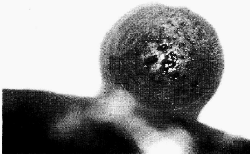
Fig. 2.10. Deposit in the Bottom of Filter 522 Housing.
