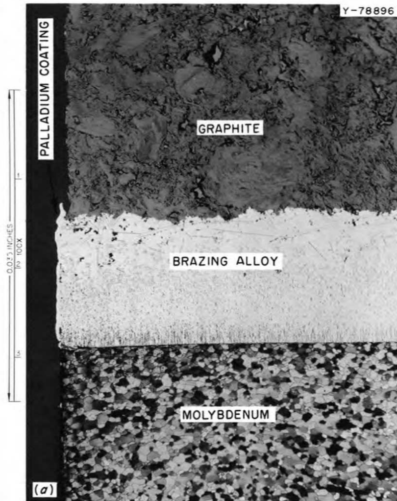
Fig. 6.18. Microstructures of the 60 Pd-35 Ni-5 Cr (wt %) Brazing Alloy Used to Join Grade CGB Graphite to Molybdenum. (a) After 5000-hr exposure to molten fluoride salts at 1300°F (705°C). Etchant: 10% oxalic acid. 100 \times . (b) Enlarged microstructure of palladium coating located primarily on the brazing alloy. Etchant: oxalic acid. 500 \times .
