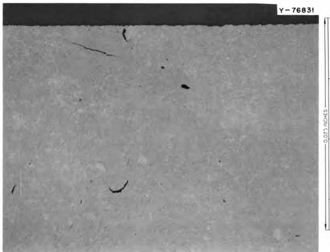
Fig. 6.15. An Experimental Isotropic Graphite, Grade B-5-1, Showing Low Porosity and a Few Flaws. As polished. 100 \times .
