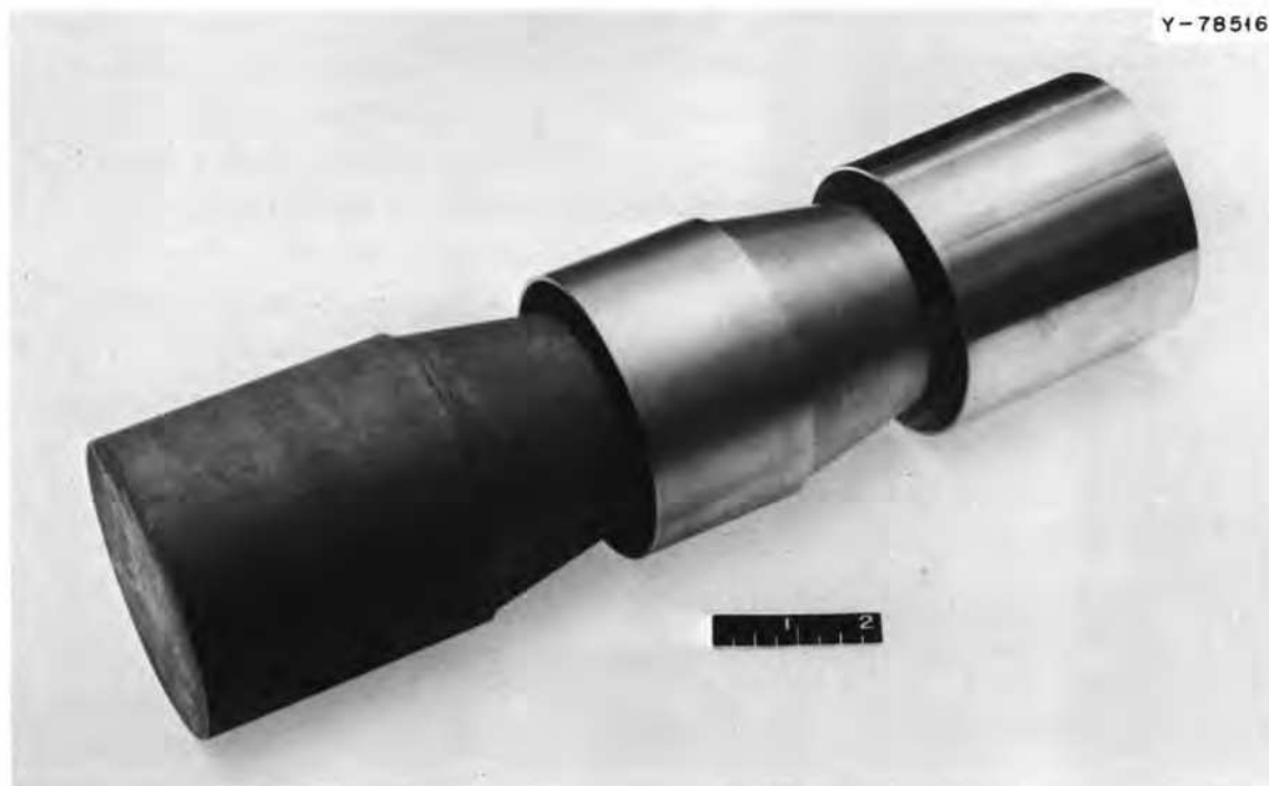
Fig. 6.17. As-Machined Components for Graphite-to-Molybdenum-to-Hastelloy-N Tapered Joint.
