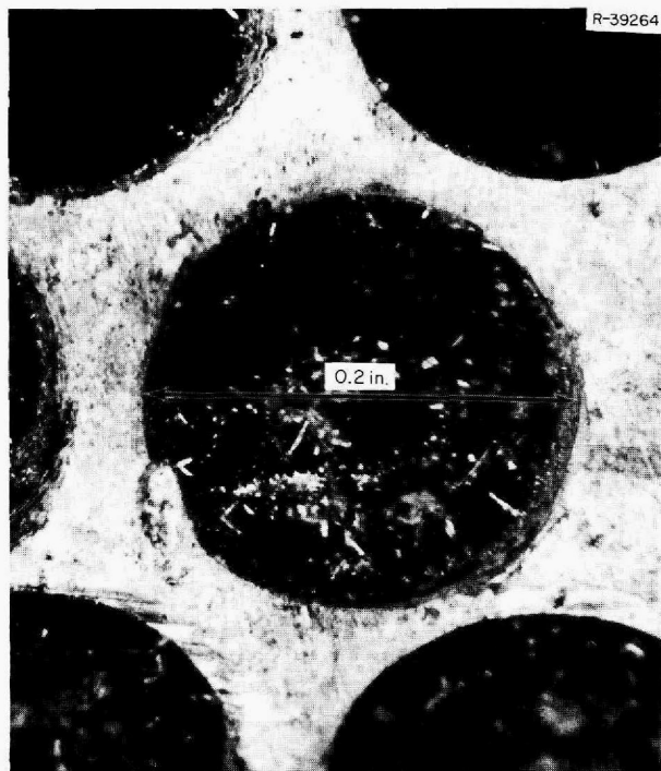
Fig. 8.5. Dendritic Crystals and Salt on Basket of Beryllium Addition Capsule FP12-56.
