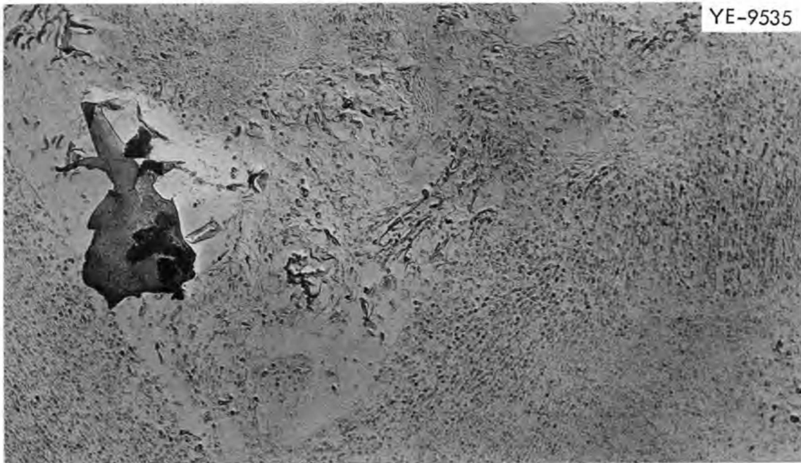
Fig. 4. Electron Micrograph of a Surface Replica of Impregnated CGB Graphite. The surface involved is selected and not necessarily typical; the magnification is approximately 10,000 \times . The radius of the large pore shown here is about ten times greater than the most probable radius for large-pore entrances (see text and Fig. 5).
