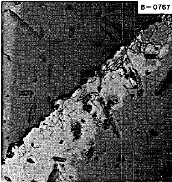
Fig. 18.9. Distribution of Precipitates in Hastelloy N (Heat 66-548, 0.45% Ti) After Irradiating for 1128 hr at 635°C. 10,000X.
