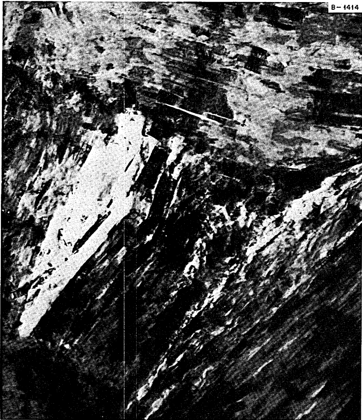
Fig. 17.1. Transmission Electron Micrograph of a Thinned Area in the AXF Graphite. The sample has a uniform thickness and the various tones varying from white to black indicate variations in the orientation of different regions. 85,000X.
