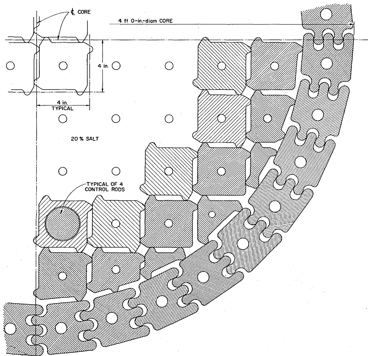
Fig. 5.19. Horizontal Section Through Core of MSBE.
