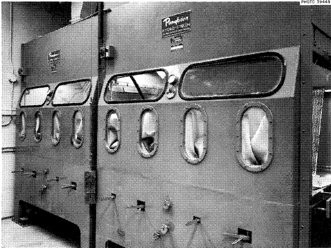
Fig. 2. Facility for Reclaiming Salt-Contaminated Equipment by Wet Sandblasting.
