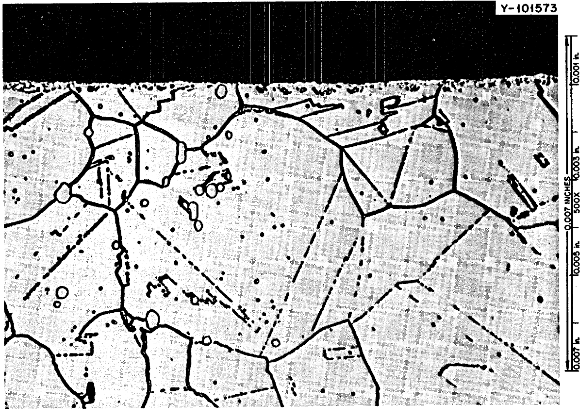
Fig. 13.13. Photomicrograph of the Outside of the Inlet Thermocouple Well That Was Exposed to Coolant Salt. Note the modified layer near the outer surface. Etchant, glycergia.
