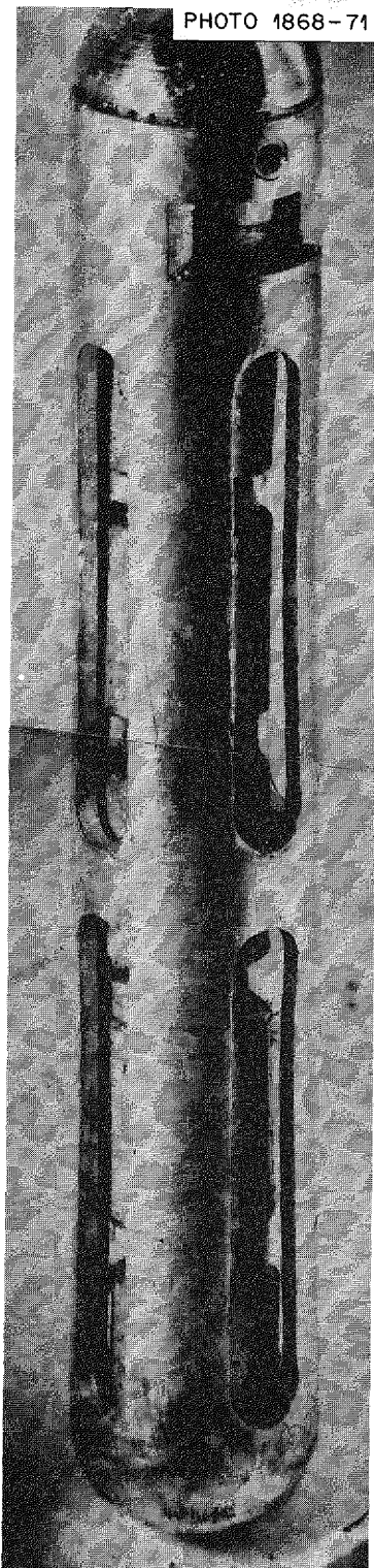
Fig. 6.12. Copper capsule containing several short magnets before exposure to ^{233}\text{U} fuel salt.
