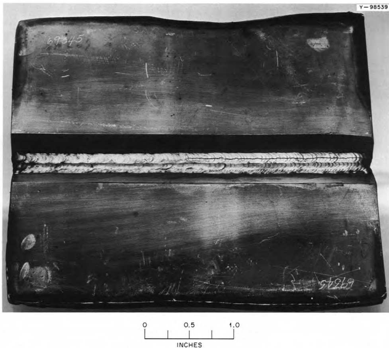
Fig. 15.9. Plate of 69-345 that cracked during welding. The plate was \frac{1}{2} in. thick and was being welded with filler metal from the same heat.
