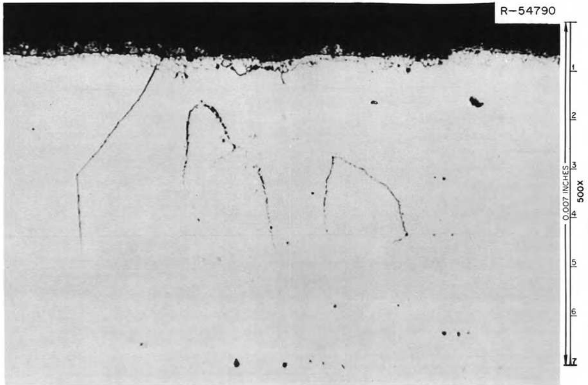
Fig. 13.14. Photomicrograph of the cross section of the Hastelloy N control rod thimble showing the outside diameter in the as-polished condition.
