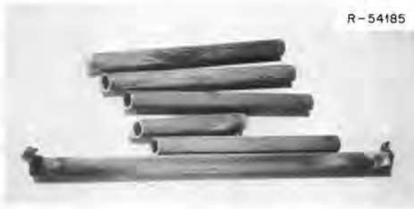
Fig. 13.25. Photograph of the \frac{1}{2} -in.-OD Hastelloy N tubes from the primary heat exchanger. The different shades arise from a dark film that is thought to have been deposited when the shell was being cut. The film was deposited on the side of the tubes facing the shell.
