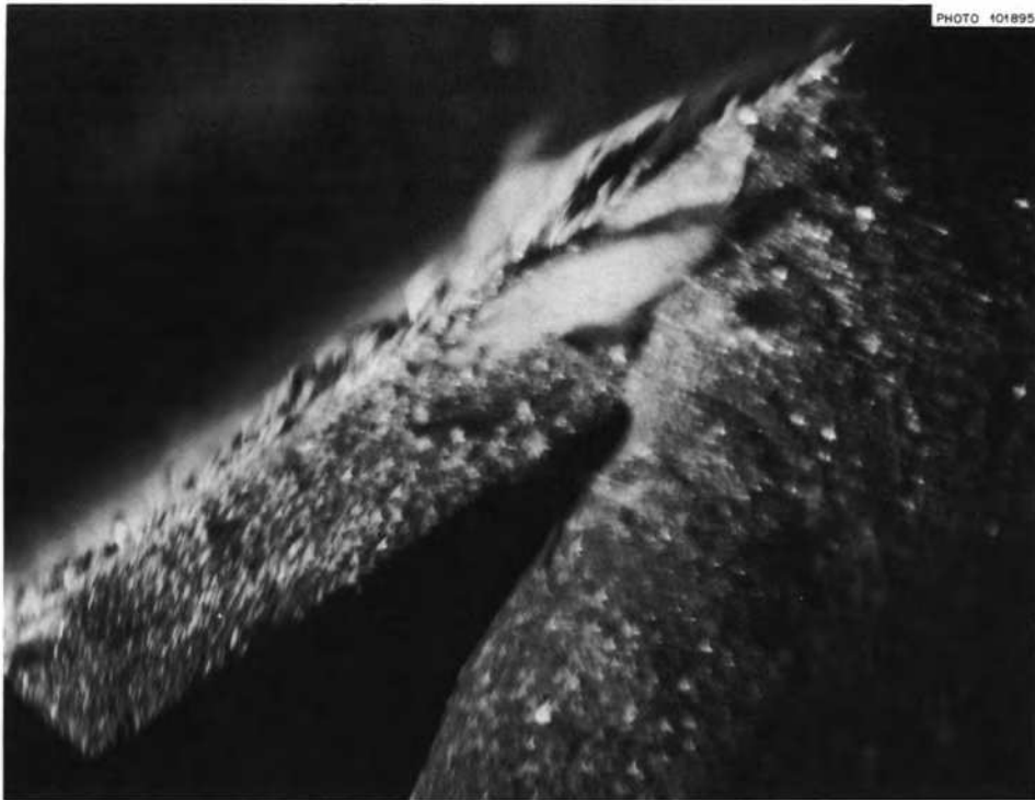
Fig. 1.10. Closeup of end of spray ring and baffle in fuel pump showing deposit.
