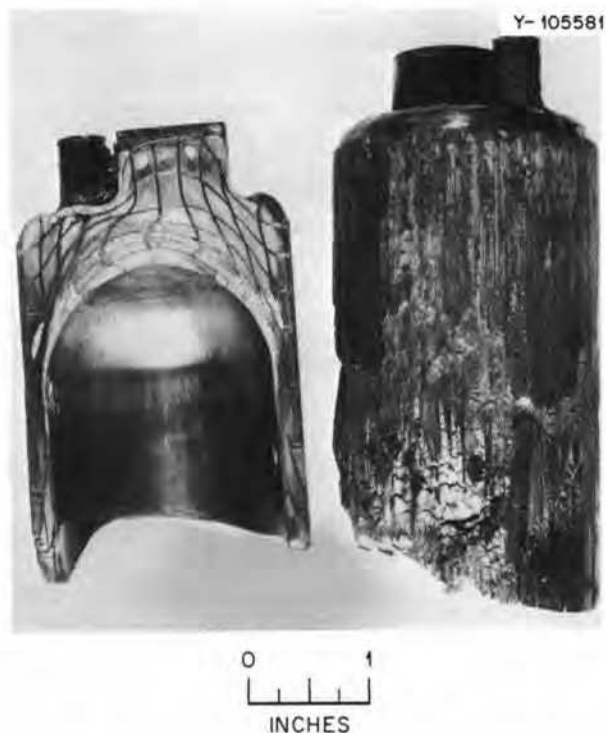
Fig. 16.2. Back-extruded molybdenum vessels. The cross section shows the deformation pattern produced by back extrusion of a square grid network in the original blank.
