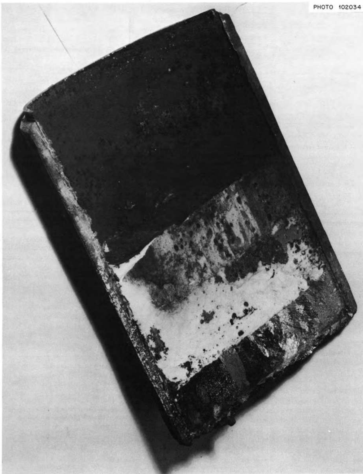
Fig. 19.5. Salt and bismuth phases from fluoride salt compartment on completion of metal transfer experiment MTE-2.
