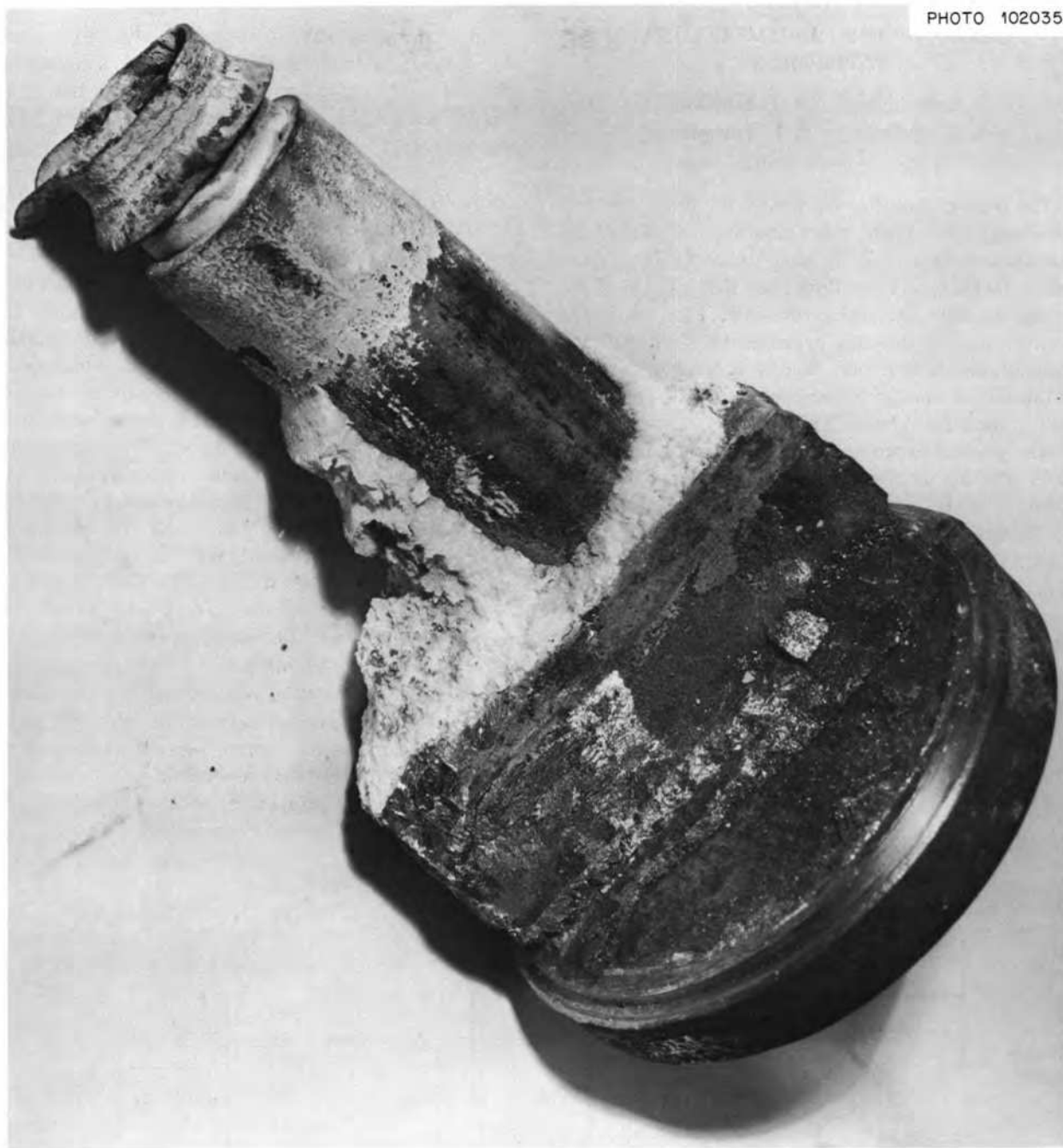
Fig. 19.6. View of LiCl compartment after removal of most of the LiCl following metal transfer experiment MTE-2.
