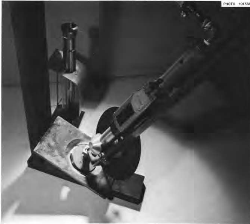
Fig. 1.7. Tool for excising fuel pump sampler cage, mounted on mockup of top of pump tank.
