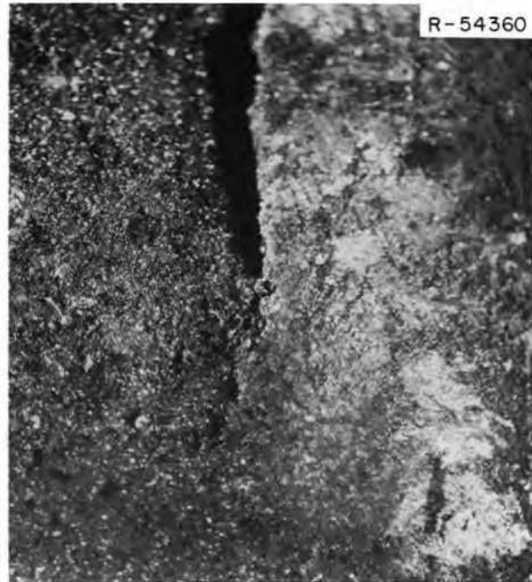
Fig. 13.18. Photograph of the crack formed in the copper sampler that was retrieved from the pump bowl. The outer surface was coated with deposited material.
