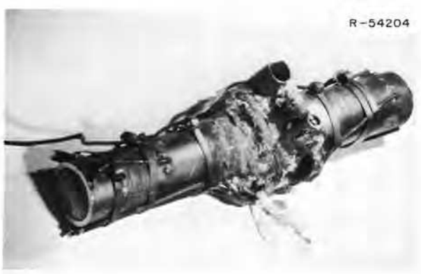
Fig. 13.30. Photograph of the bottom portion of freeze valve 105.
