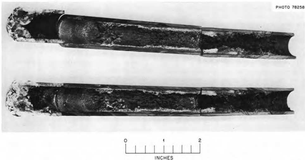
Fig. 15.35. Photograph of the inside of Inconel 600 bubbler tube from PKP-1 pump loop exposed to 13.5 vol % \text{BF}_3\text{-bal He} for 11,500 hr.
