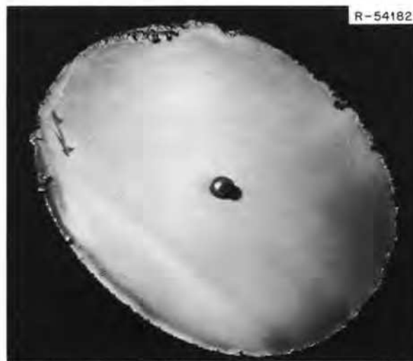
Fig. 13.22. Section 10 × 13 in. cut from the primary heat exchanger shell. The piece was cut with a plasma torch, and the center stud was used for guiding the torch.
