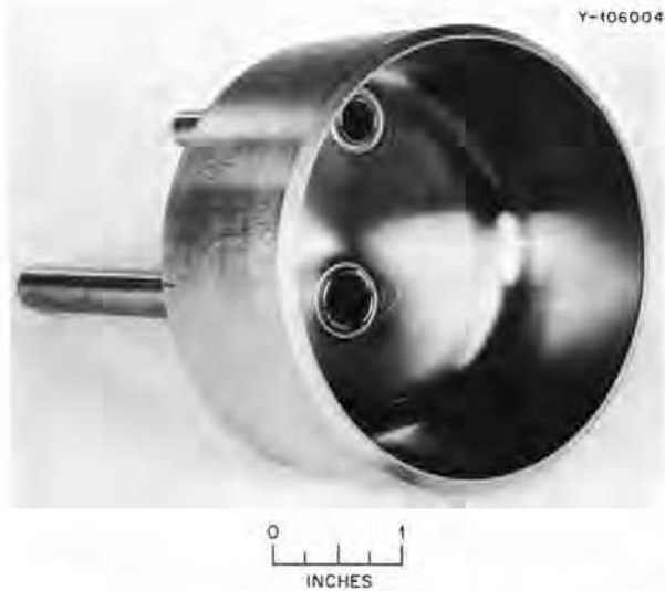
Fig. 16.5. Tubes (0.375 in. diam, 0.025 in. wall; 0.500 in. diam, 0.030 in. wall) electron-beam welded into a back-extruded molybdenum header.
