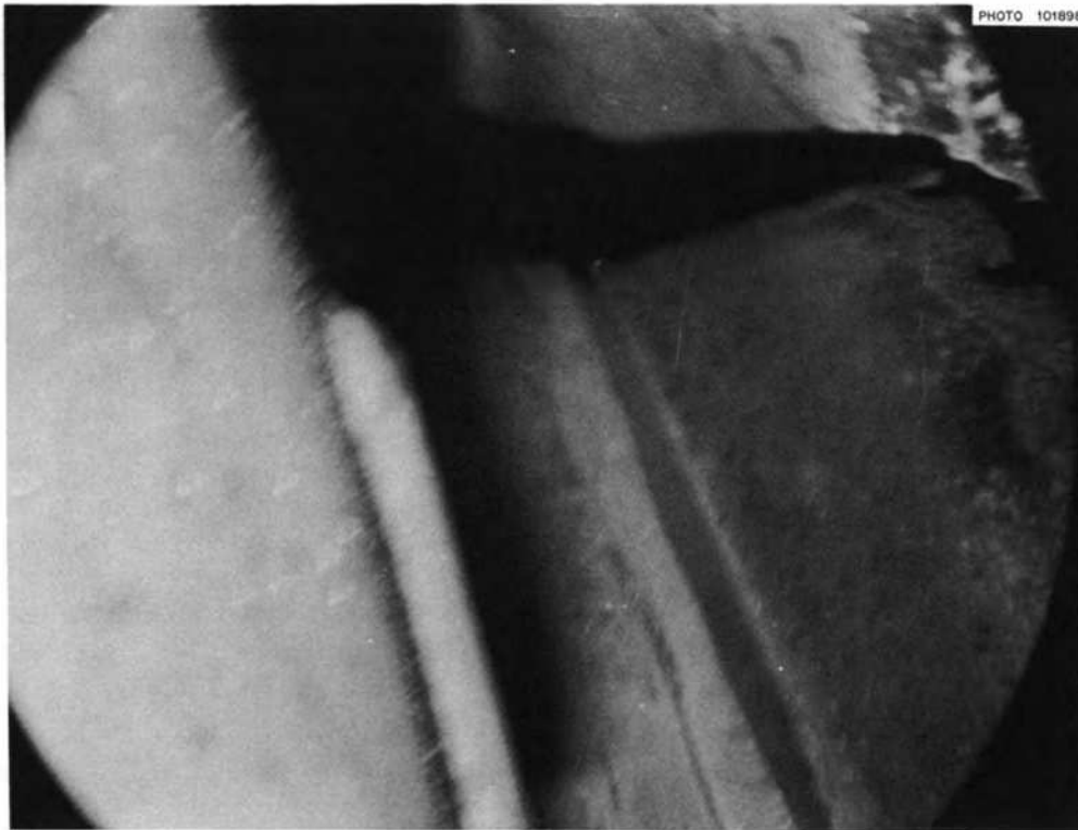
Fig. 1.11. View in lower part of pump bowl showing ports into volute suction.
