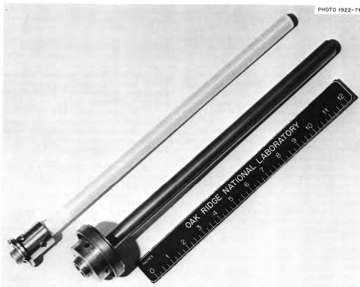
**Fig. 17.17. Prototype interface detector probe before assembly.** The molybdenum sheath tube and bifilar-wound primary and secondary coils are shown.
