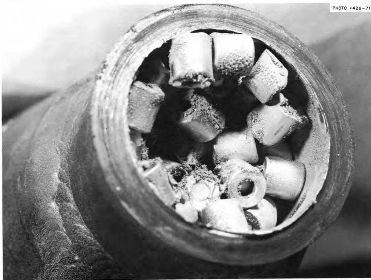
Fig. 18.1. View of Raschig-ring packing near top of packed column, showing metallic deposits and salt that did not drain from the packing.
