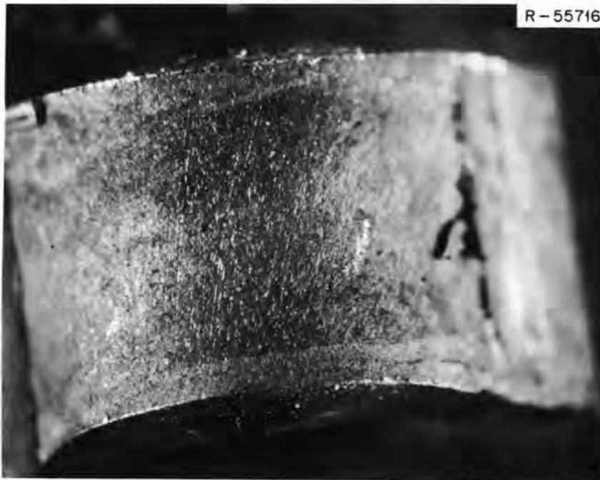
Fig. 11.13. Macrograph of tension side of bend specimen from top of core vessel of in-pile loop 2, exposed to flowing fuel salt. Specimen did not fail. 5.5x.
