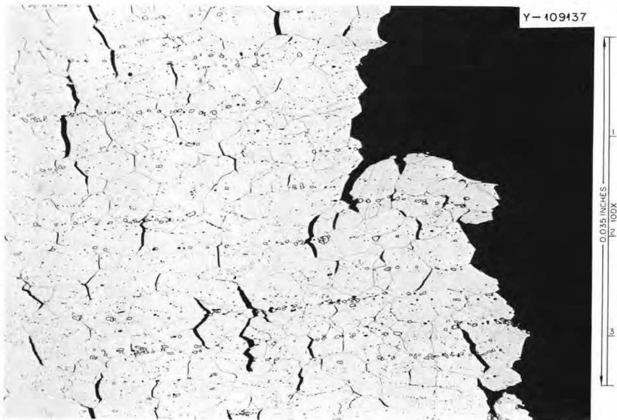
Fig. 13.28. Photomicrograph of the fracture of Hastelloy N (heat 5065) stressed at 60,000 psi at 593°C without NaCl coating. Etchant: Gly Regia.
