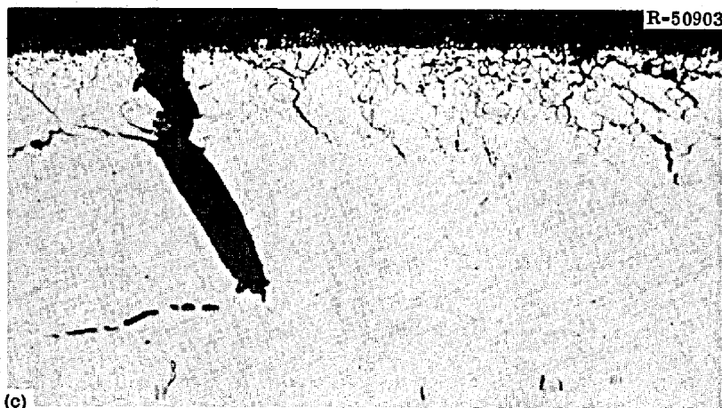
Fig. 46. Photomicrographs of INOR-8 (Heat 5085) Sample Tested at 25°C After Being Exposed to the MSRE Core for 19,136 hr Above 500°C and Irradiated to a Thermal Fluence of 1.5 \times 10^{21} neutrons/cm 2 . (a) Fracture, etched. 100x. (b) Edge, as polished. 100x. (c) Edge, as polished. 500x. (d) Edge, etched. 100x. Etchant: glyceria regia. Reduced 27%.
