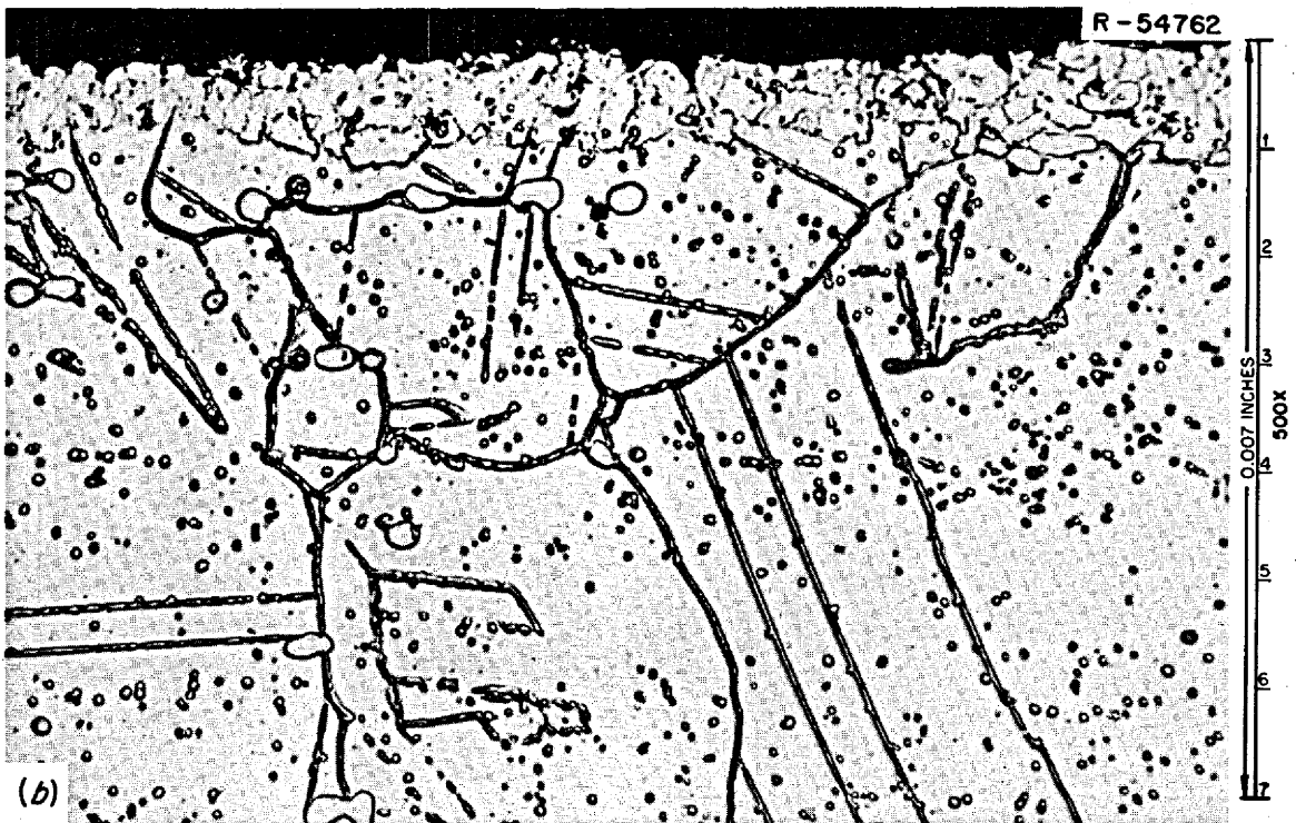
Fig. 77. Photomicrographs of the Inside Surface of the Primary Heat Exchanger Shell. The surface was exposed to fuel salt, and the modified structure to a depth of about 1 mil is apparent. (a) As polished. (b) Etched with aqua regia.
