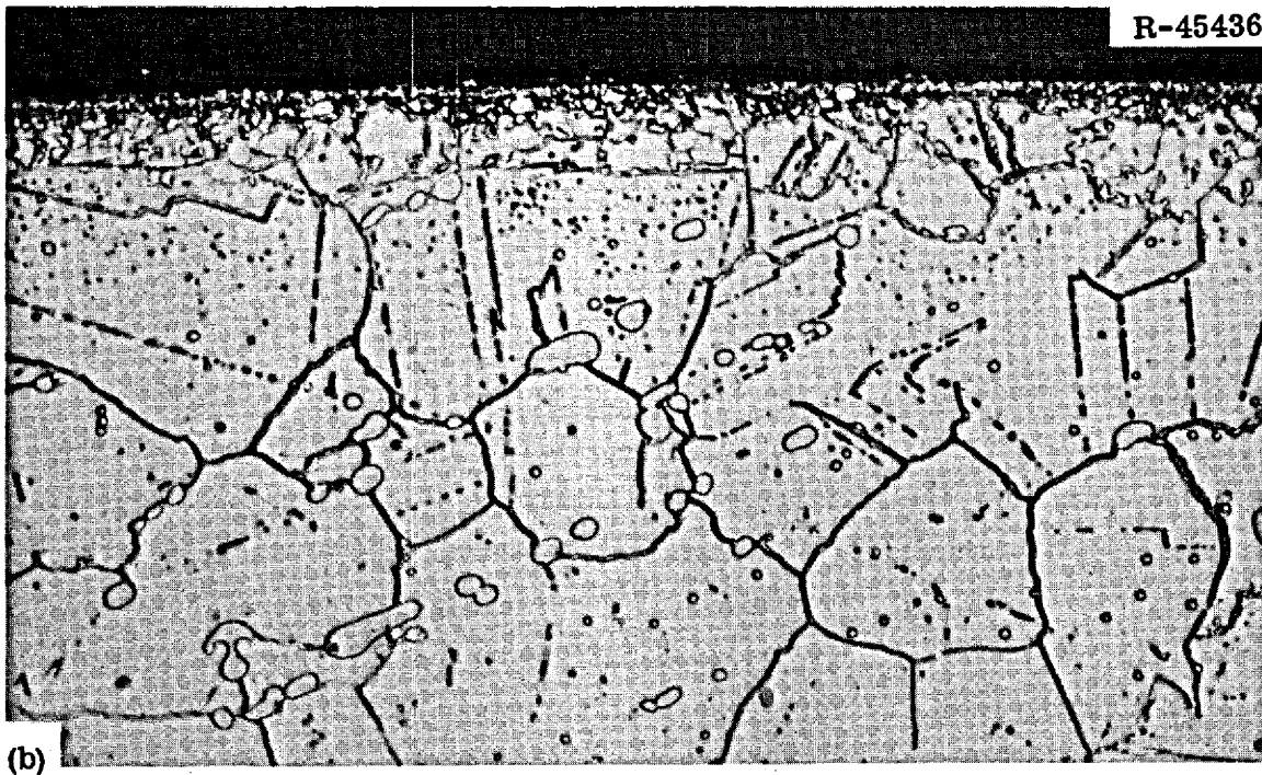
Fig. 19. Photomicrographs of INOR-8 (Heat 5065) Surveillance Specimens Exposed to Fuel Salt for 11,933 hr above 500°C, 500x. Shallow reaction layer is seen near surface. (a) Unetched. (b) Etched (glyceria regia).
