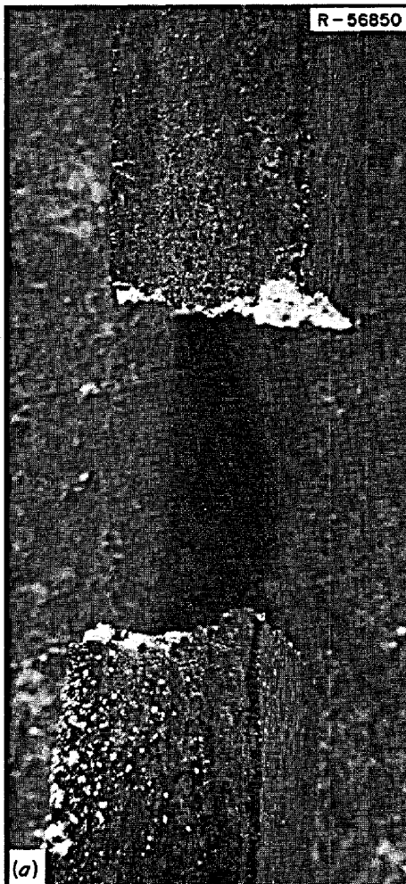
Fig. 102. The Surfaces Exposed to Salt in Freeze Valve 105 After Deformation at 25°C. (a) Fracture of ring specimen pulled in tension. Note surface cracks near the fracture. 4x (b) Surface of bend specimen. Note some cracks on surface and edge cracks. 7x. Reduced 18.5%.
