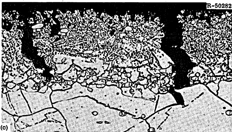
Fig. 49. Typical Photomicrographs of INOR-8 (Heat 5085) Sample Exposed to the MSRE Core for 19,136 hr Above 500°C. The sample was bent in a vise. (a) As polished, tension side. 100x. (b) As polished, tension side. 500x. (c) Etched, tension side. 500x. (d) Etched, compression side. 500x. Etchant: aqua regia. Reduced 27%.
