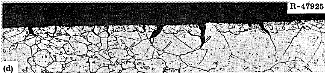
Fig. 26. Photomicrographs of INOR-8 (Heat 5085) Sample Exposed to Fluoride Salt in the MSRE for 11,933 hr above 500°C and then Tested at 25°C. Thermal fluence was 9.4 \times 10^{20} neutrons/cm 2 . (a) Fracture, as polished. 100x. (b) Fracture, as polished. 500x. (c) Fracture, etched. 100x. (d) Edge of stressed portion, etched. 100x. Etchant: aqua regia.
