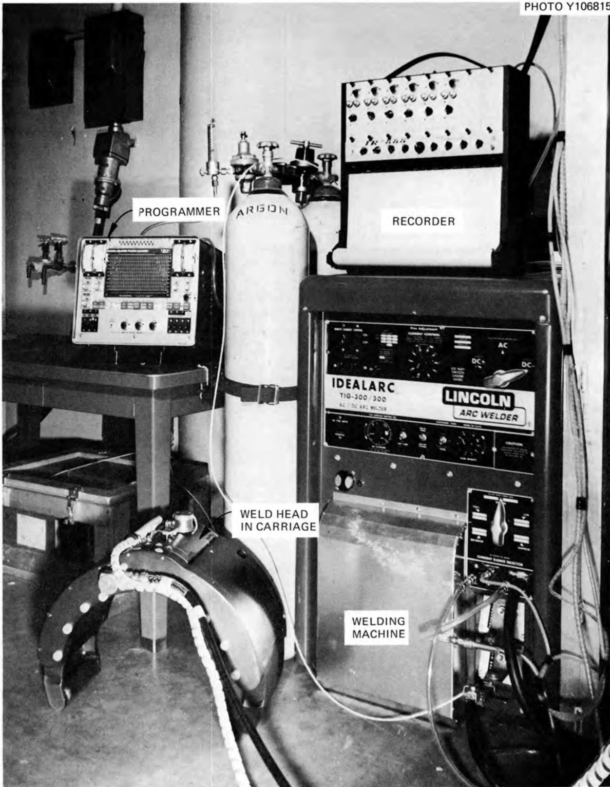
Fig. 1. ORNL automated welding system installation prior to carriage placement on 12- to 16-in. pipe.
