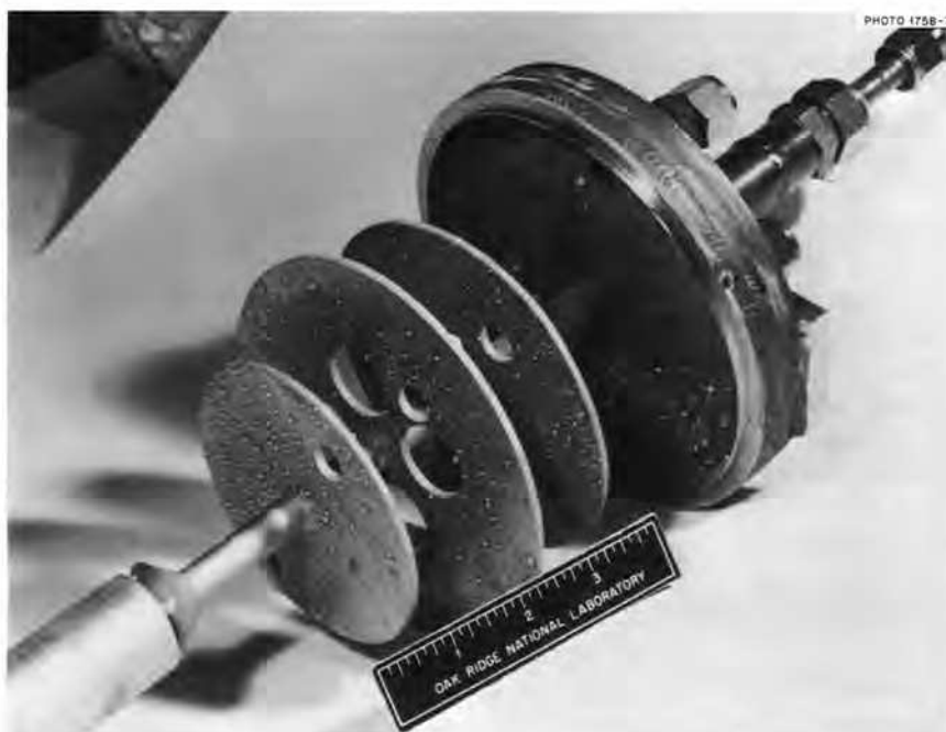
Fig. 16.8. Photograph of gas inlet and draft tube assembly removed from precipitator vessel at termination of operation.
