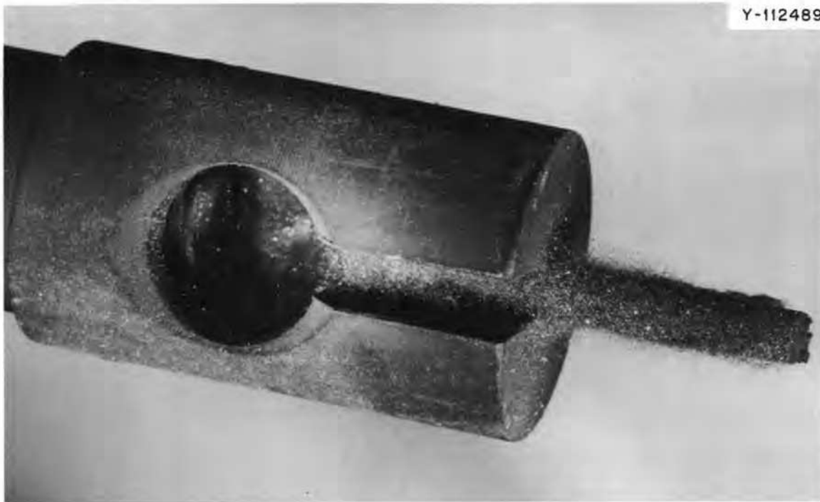
Fig. 10.22. Typical appearance of nickel telluride on a fractured Hastelloy N specimen exposed to tellurium during a 650°C creep test. The sample is still in the specimen grip.
