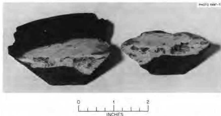
Fig. 16.7. Photograph of salt and oxide heel removed from precipitator vessel at termination of operation.
