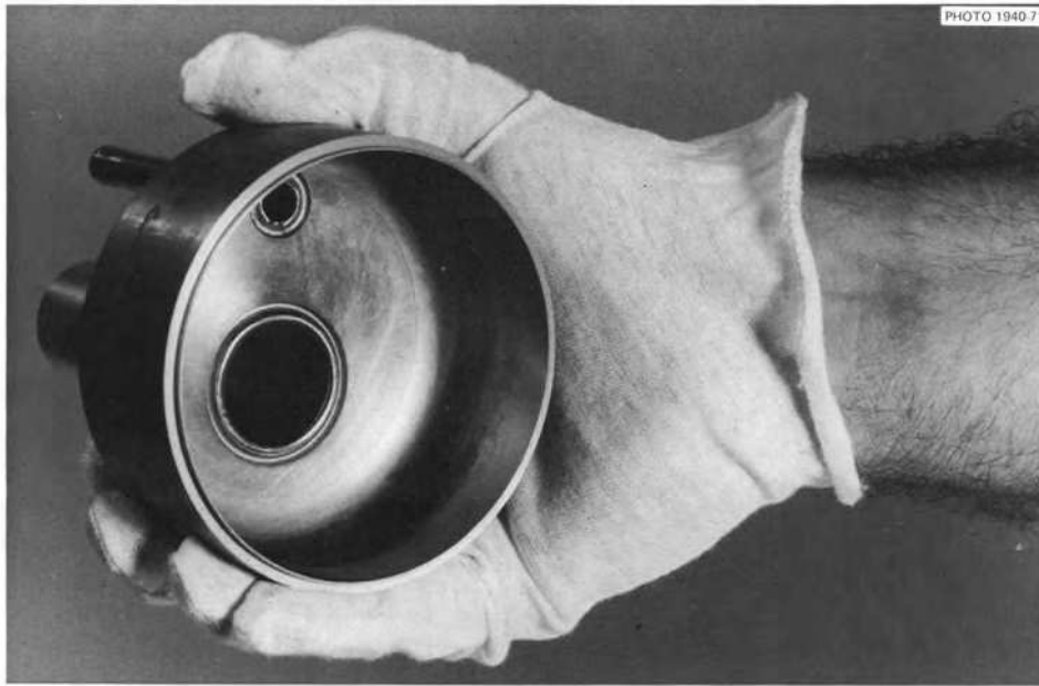
Fig. 12. Back-extruded half section with two tube-to-header welds made by the electron-beam process.
