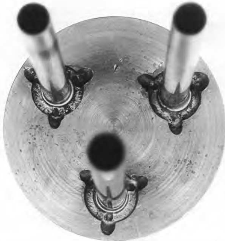
Fig. 27. Mockup of stainless steel nozzle body brazed to molybdenum tubes. Body diameter, 2 in.
