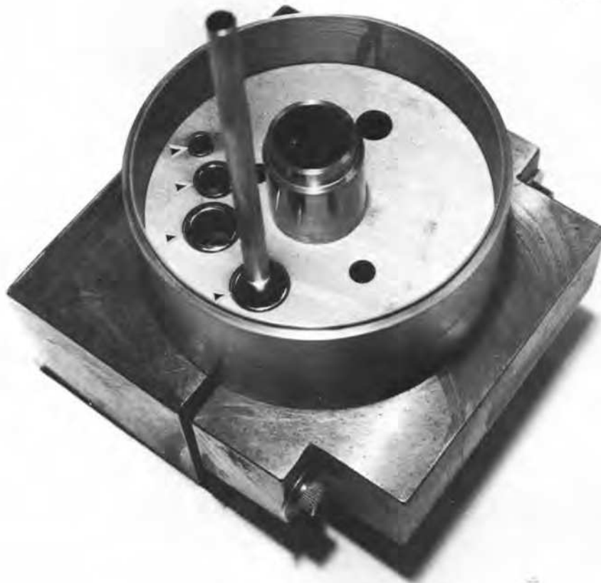
Fig. 11. Weirs electron-beam welded (at arrowheads) to one of the baffle plates shown installed in the upper half of the bismuth feed pot.
