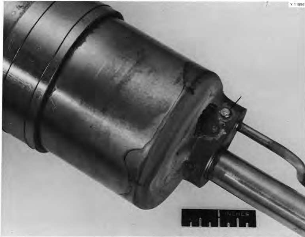
Fig. 37. Upper end of the bismuth feed pot after furnace brazing of the girth band and tube-to-header joints with the iron-base brazing filler metal. Note the molybdenum caps brazed over the reservoirs in the boss (arrow).
