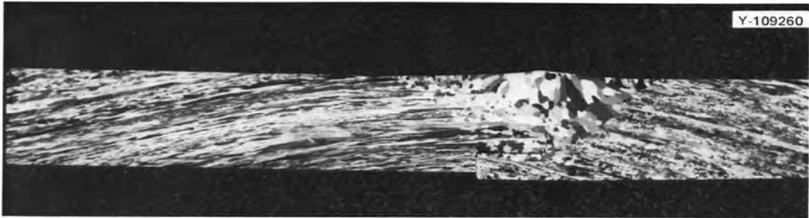
Fig. 19. Cross section through electron-beam cylindrical girth weld shown in Fig. 18. Etchant: 20 vol % \text{H}_2\text{O}_2 - 10 vol % \text{H}_2\text{SO}_4 (96% \text{H}_2\text{SO}_4 ) - 70 vol % \text{H}_2\text{O} . 6X.
