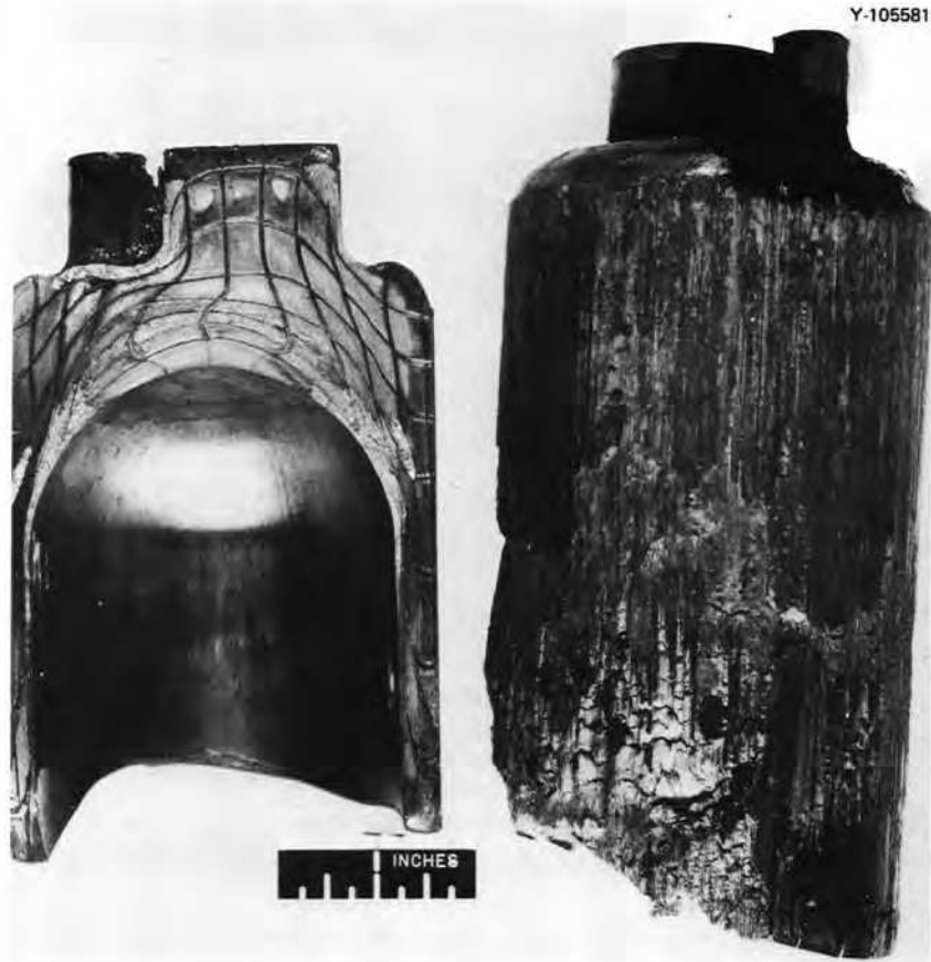
Fig. 6. Flow pattern in a molybdenum back extrusion revealed by a network of tantalum wires installed in half of the original blank.
