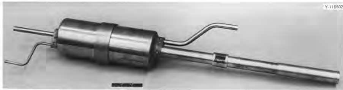
Fig. 28. Mockup of column joined to upper disengaging section. A split sleeve was brazed with Fe-15% Mo-5% Ge-4% C-1% B over a tungsten-arc weld.
