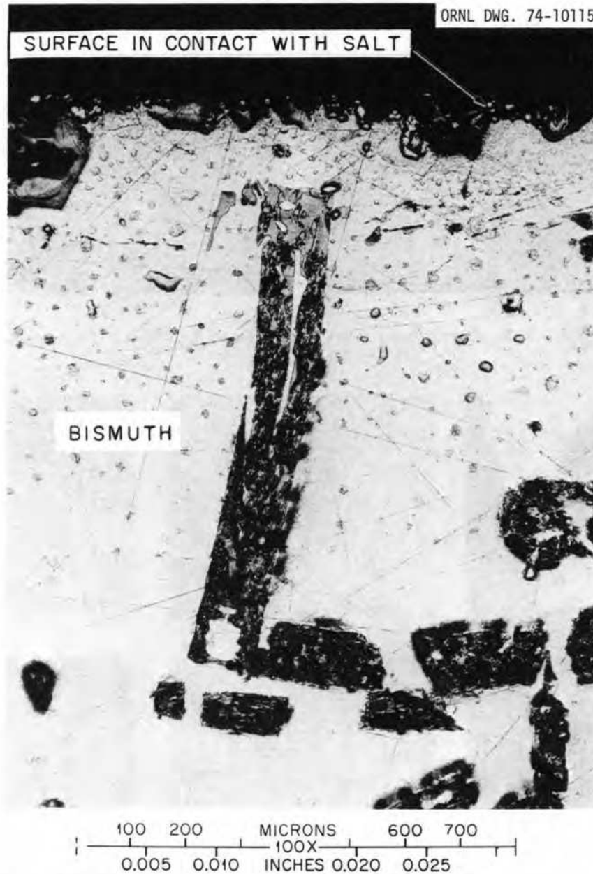
Fig. 14.5. Photomicrograph of the Li-Bi phase from the stripper at the LiCl interface, MTE-3.
