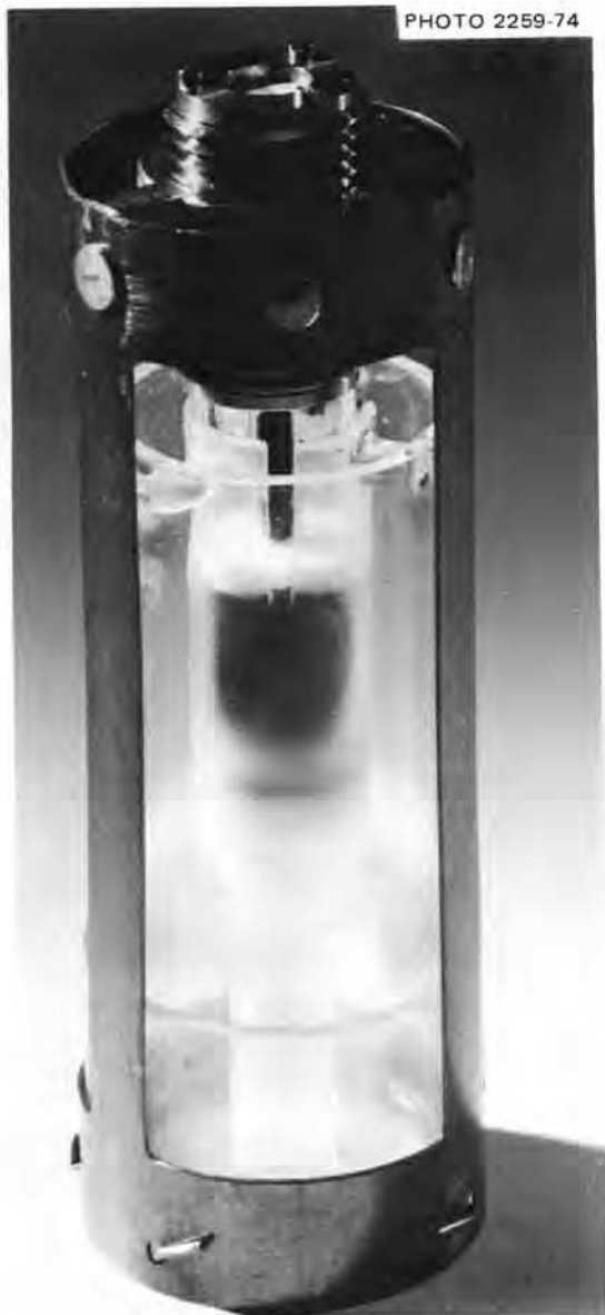
Fig. 9.3. Packed-bed electrode assembly with glassy carbon spheres for use in molten salts.
