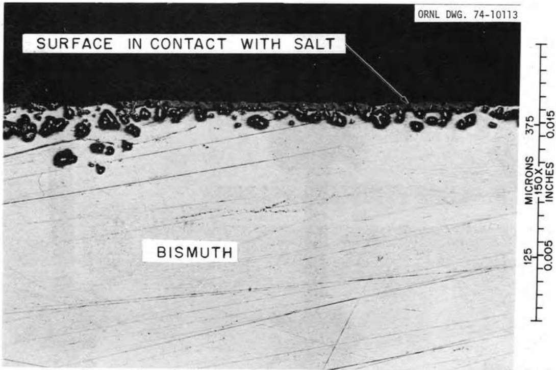
Fig. 14.3. Photomicrograph of the Bi-Th phase from the contactor at the fluoride salt interface, MTE-3.
