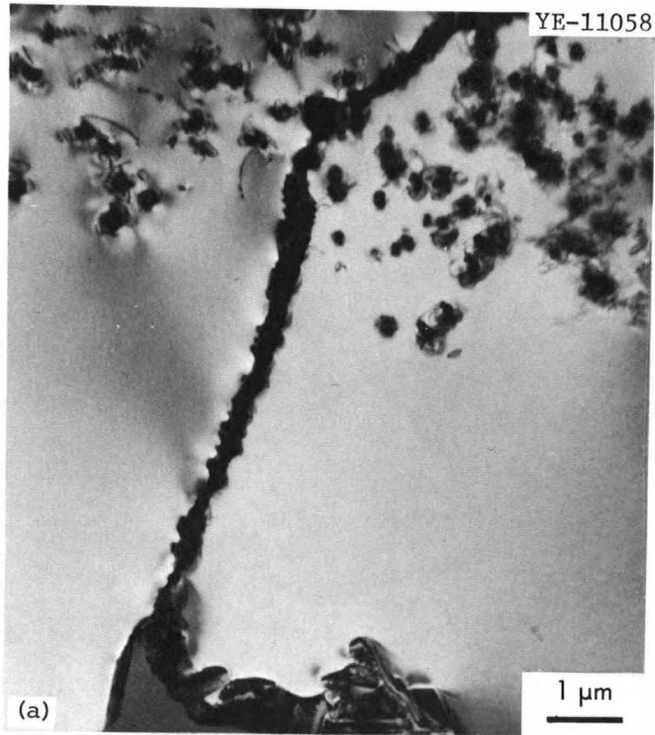
Fig. 10.8. Effect of aging at 760°C on microstructure of 1.2% Ti-modified Hastelloy N. (a) Solution annealed 1 hr at 1260°C. (b) Solution annealed 1 hr at 1260°C and aged 200 hr at 760°C.
