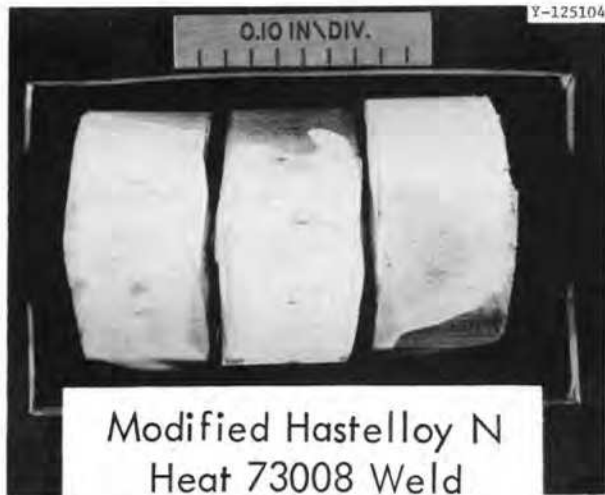
Fig. 10.1. Photomicrograph of side bend specimens 1/8-in. thick by 1/2-in. wide bent around a 3/8-in.-radius mandrel. Dye penetrant has been applied, and dark streaks indicate shallow cracks.
