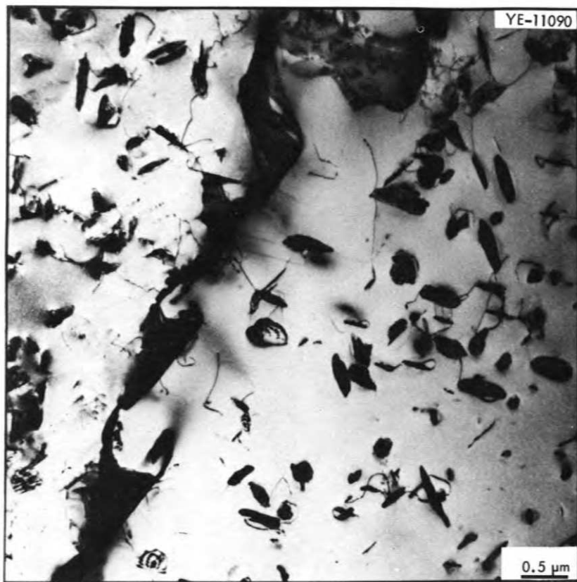
Fig. 7.24. Electron micrographs of alloys 503 (left) and 114 (right) after irradiation at 704°C for 1200 hr.
