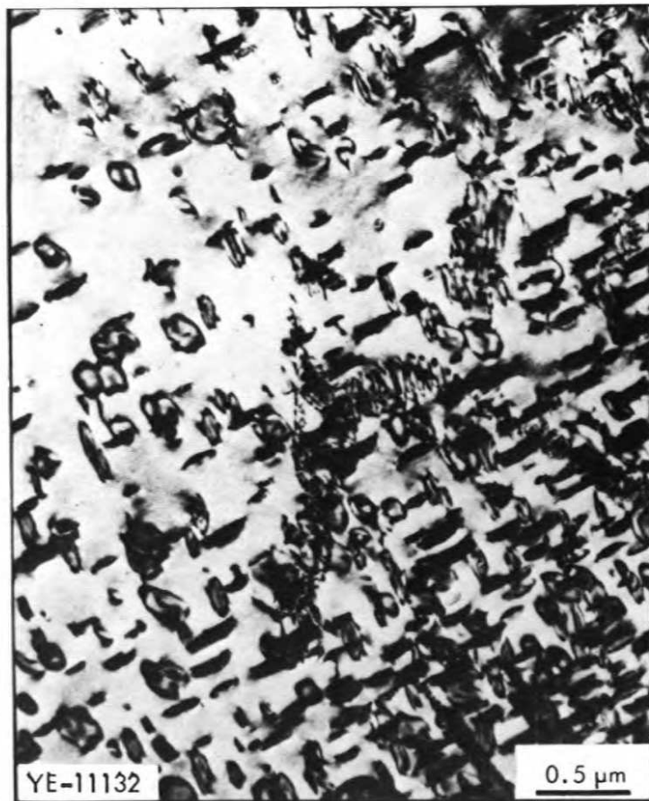
Fig. 7.16. Transmission electron micrograph of Heat 433, aged 100 hr at 704°C, showing dispersion of gamma prime and Ni, Nb platelets. On left, bright field contrast; on right, dark field contrast.
