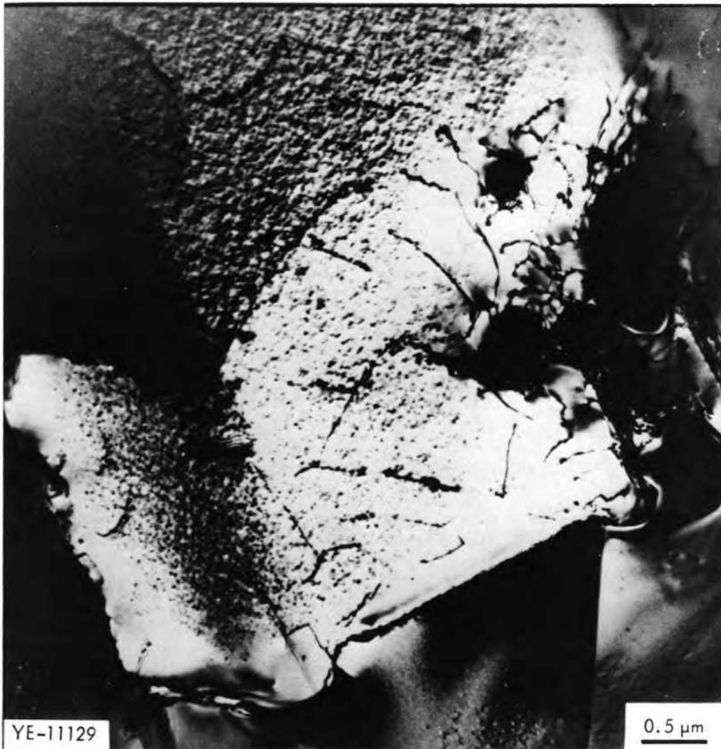
Fig. 7.14. Transmission electron micrograph of Heat 430, aged 100 hr at 650°C, showing dispersion of spherical gamma prime (200-300 Å diam) and coarser MC precipitates.
