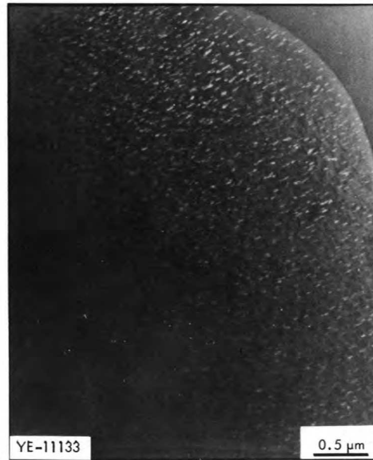
Fig. 7.16. Transmission electron micrograph of Heat 433, aged 100 hr at 704°C, showing dispersion of gamma prime and Ni, Nb platelets. On left, bright field contrast; on right, dark field contrast.
