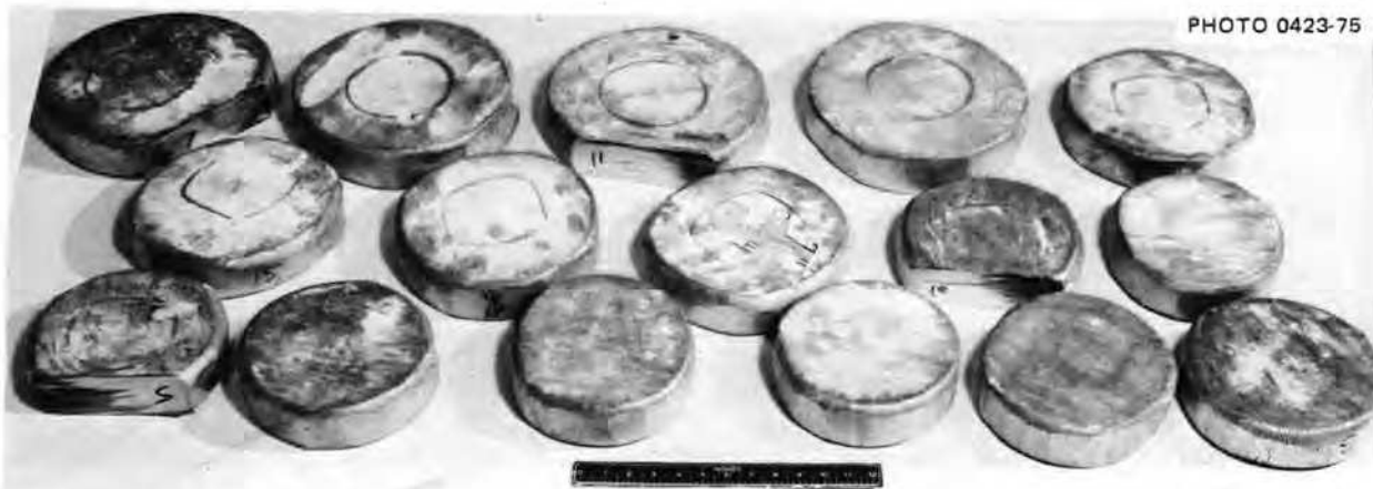
Fig. 7.3. Upset forgings of 2% Ti-modified Hastelloy N (Heat 2810-4-7901). Approximately 2\frac{1}{4} -in. thick.
