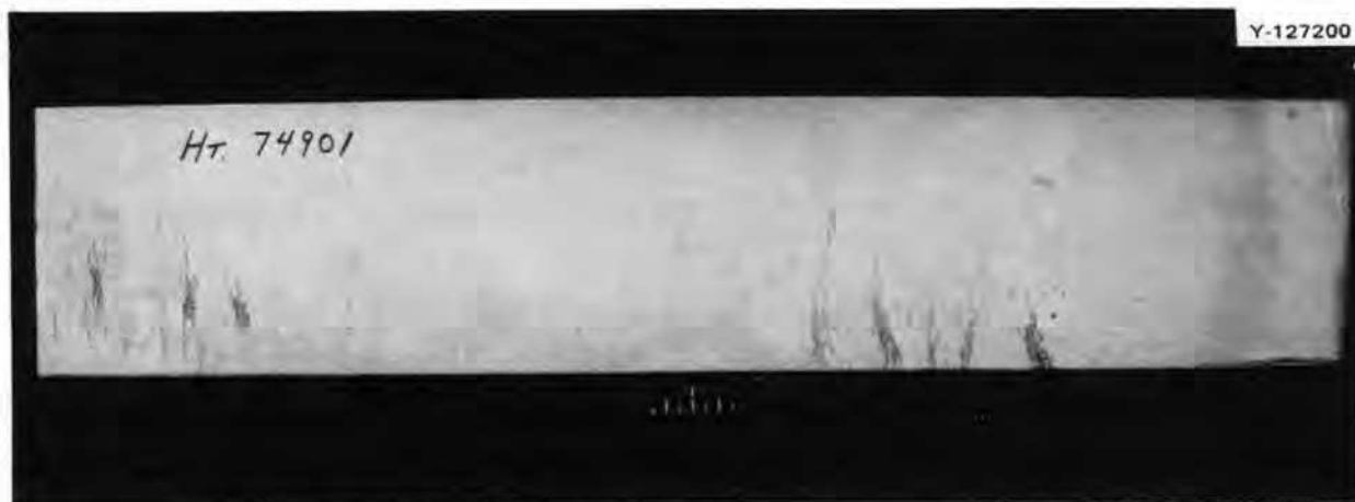
Fig. 7.1. Surface cracks observed on 1/2-in.-thick hot-rolled plate of production heat of 2% Ti-modified Hastelloy N (Heat 2810-4-7901).
