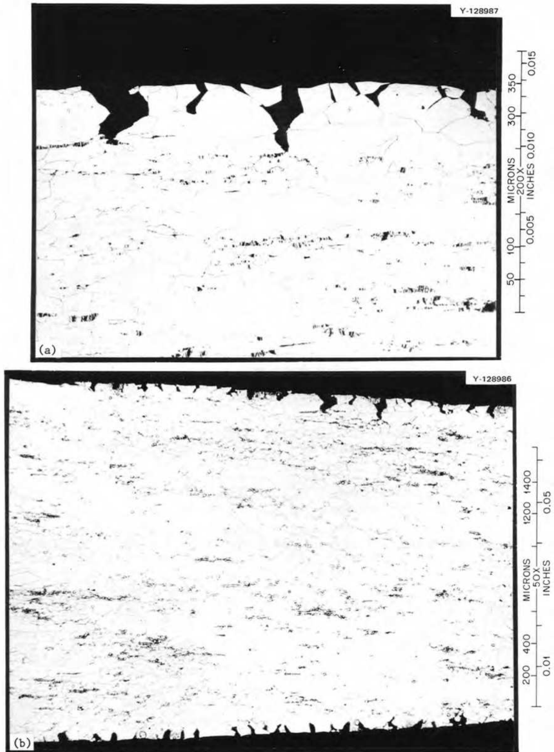
Fig. 4.1. Hastelloy N specimen after tensile testing. Specimen has been cut in half and etched to show the grain boundaries. (a) magnification 200x; (b) magnification 50x. Reduced 14%.
