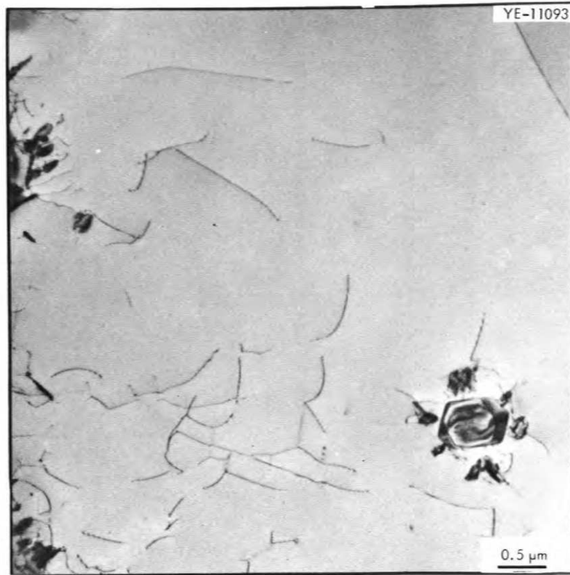
Fig. 7.25. Electron micrographs of alloys 503 (left) and 114 (right) after irradiation at 760°C for 1200 hr.
