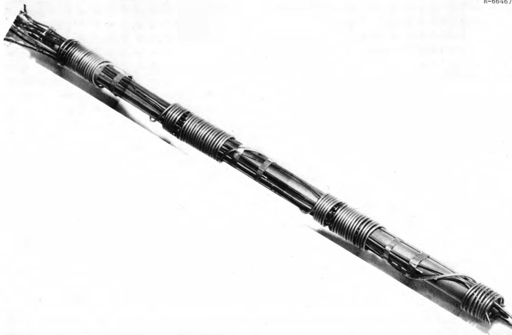
Fig. 7.50. Composite photograph of TeGen-1 fuel capsules as removed from assembly with heater coils, thermocouples and flux monitor intact. Inconel 601 fuel pin at bottom right, Hastelloy N in middle, and 304 stainless steel at top left.
