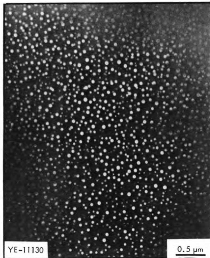
Fig. 7.15. Transmission electron micrograph of Heat 431, aged 100 hr at 800°C, showing dispersion of spherical gamma prime (300-600Å diam). On left, bright field contrast; on right, dark field contrast.
