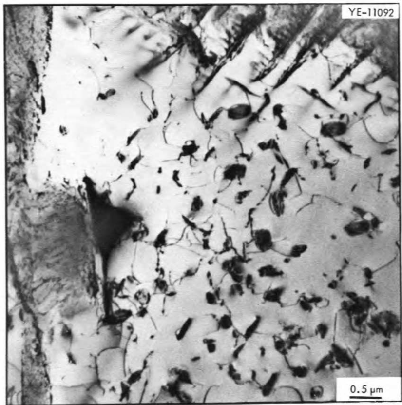
Fig. 7.25. Electron micrographs of alloys 503 (left) and 114 (right) after irradiation at 760°C for 1200 hr.
