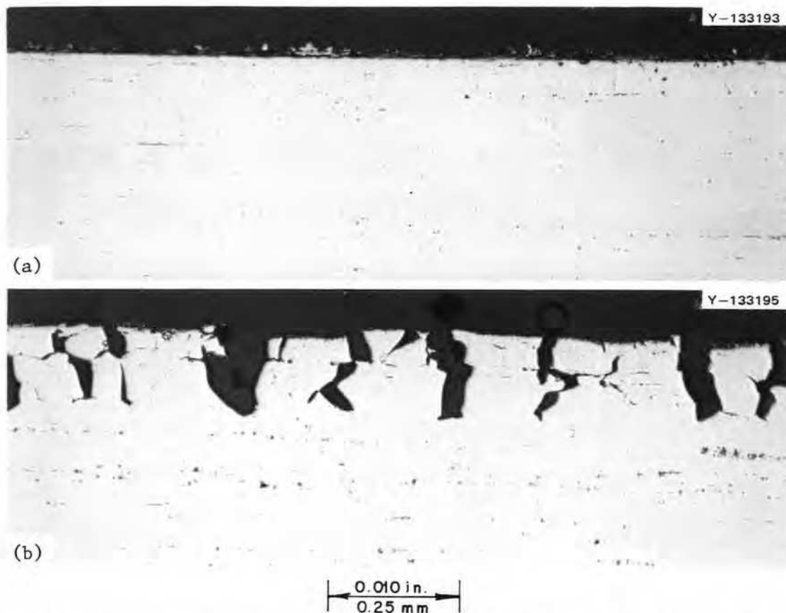
Fig. 6.56. Standard Hastelloy N (heat 5065) exposed to LiCl saturated with \text{Cr}_2\text{Te}_3 at 750^\circ\text{C} for 146 hr. (a) Edge of unstressed portion of specimen, (b) edge of stressed portion of specimen. As polished, 100X.
