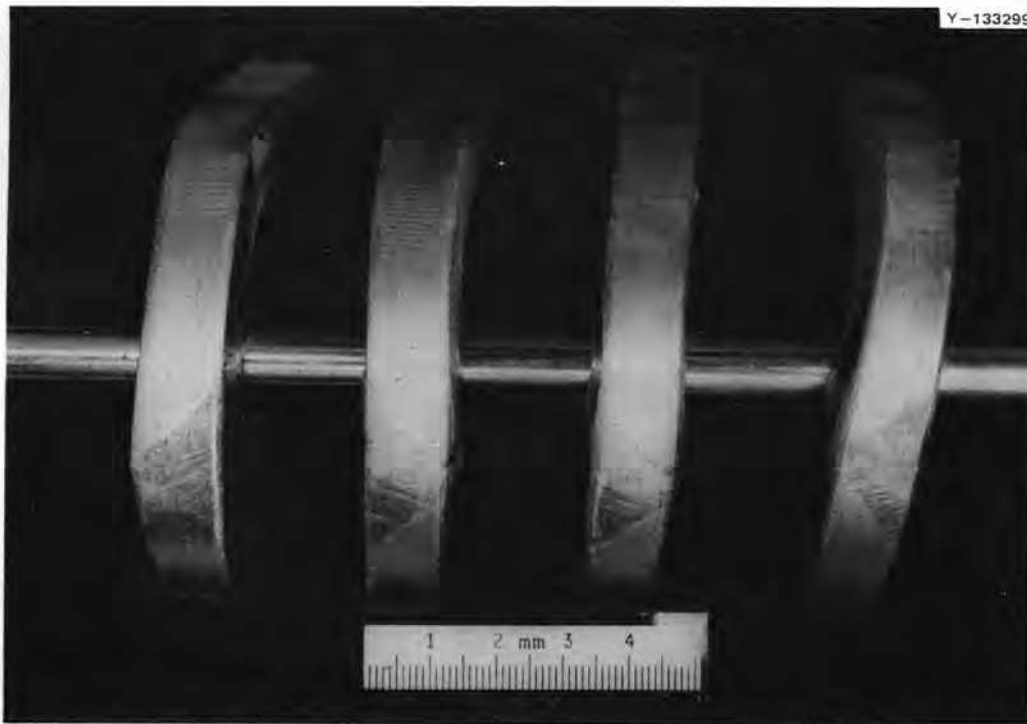
Fig. 6.23. Bend specimens of type 304 stainless steel and 2% Ti-modified Hastelloy N (heat 74-901) joined with 82T filler wire.
