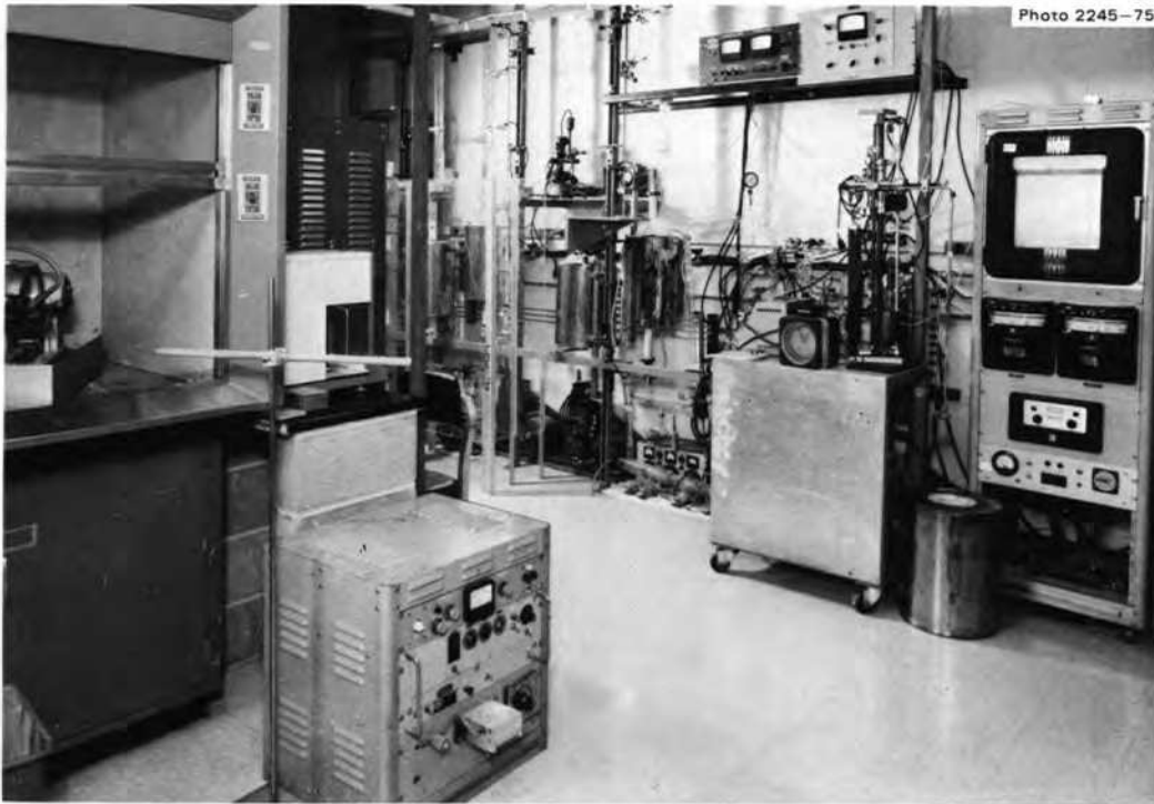
Fig. 6.13. Typical view of general-purpose laboratory used primarily to study tellurium-metal reactions. The hood on the left is used to clean salt from specimens tested in salt environments.
