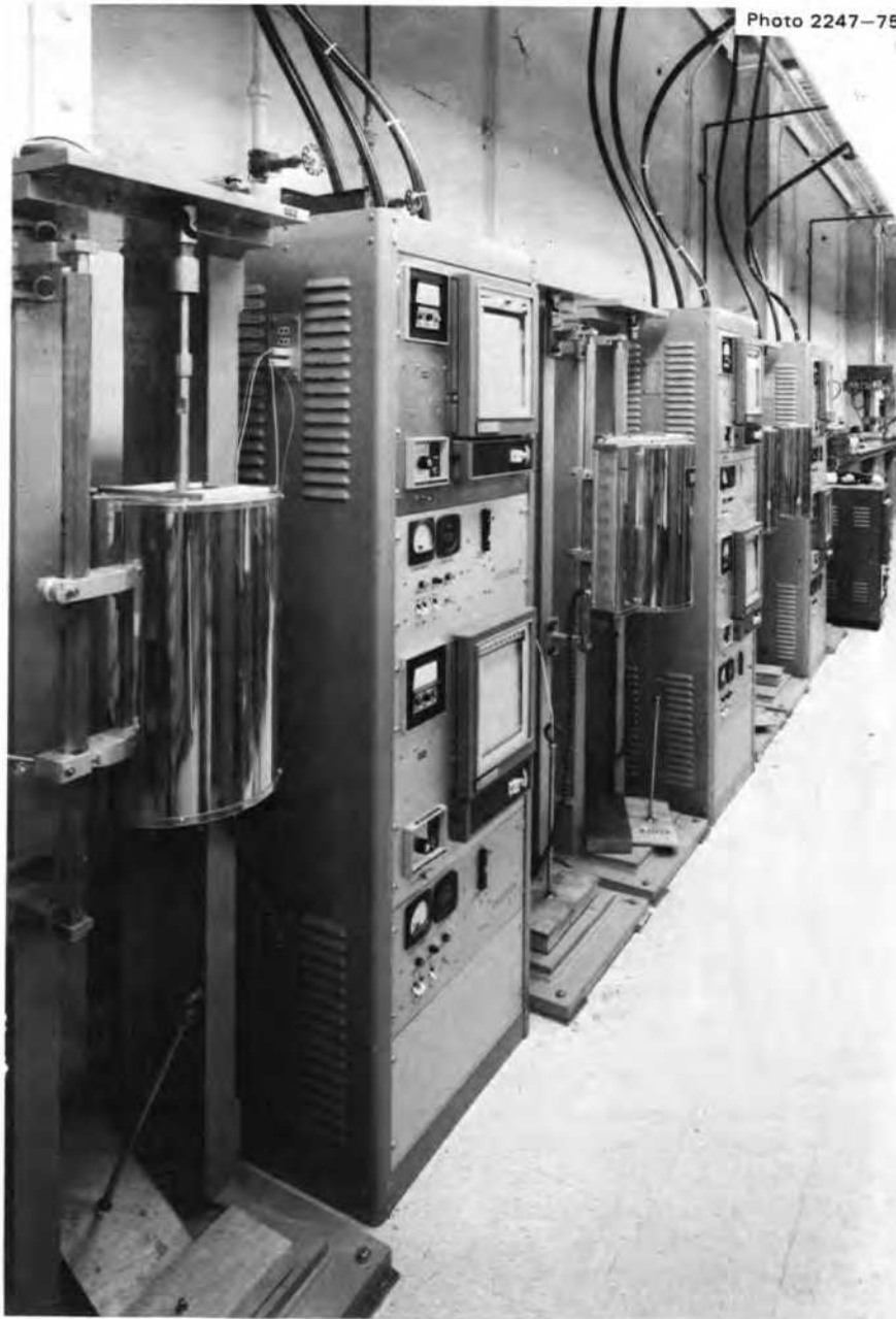
Fig. 6.7. General view of air-environment dead-load creep machines.
