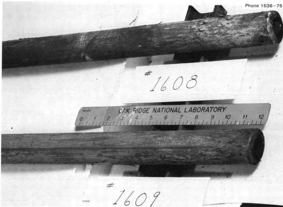
Fig. 6.17. Tube-blank extrusions of 2% Ti-modified Hastelloy N (heat 75-421). These are the leading ends of the two extrusions and were photographed in the as-extruded condition.
