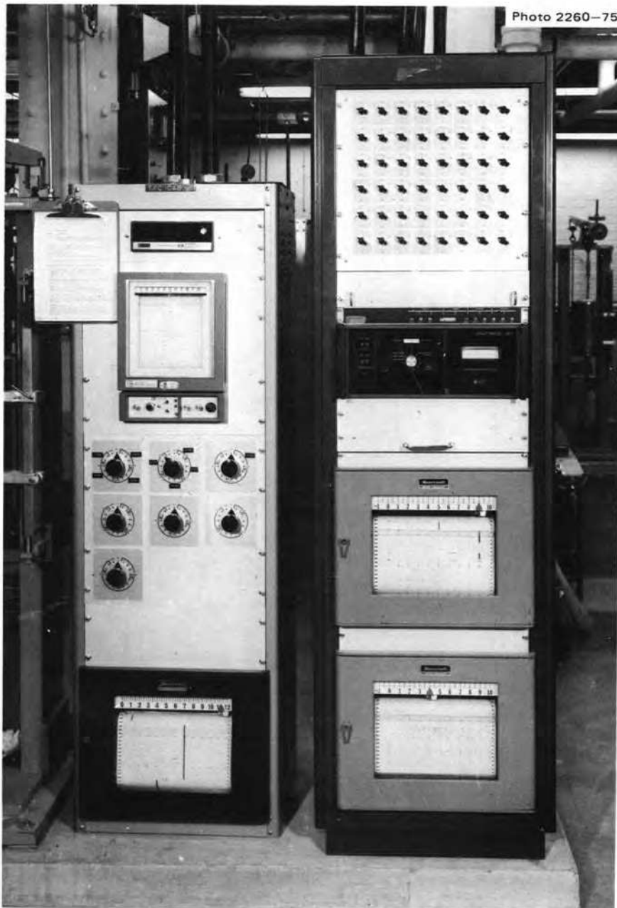
Fig. 6.11. The cabinet on the left is one of several readout stations for temperature. Chromel-Alumel sensors from several creep machines are run to this cabinet. The switches make it possible to read each thermocouple individually on the digital unit at the top of the cabinet. One point at a time can be recorded on the Azar recorder. The cabinet on the right contains a data logging unit for recording strain and temperature on all the machines on the first floor. The three recorders in the bottoms of the two cabinets record strain data from all machines.
