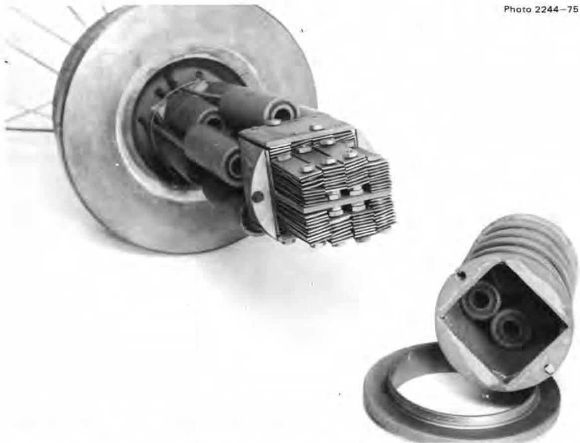
Fig. 6.50. Photograph of the steam corrosion chamber after 19,000 hr of exposure. Features to note are the stressed but uninstrumented specimens in the filter (foreground), the two groups of unstressed specimens, and the ten instrumented stressed specimens. The stressed specimens have an outside diameter of 1 in. and a length of 3 in.
