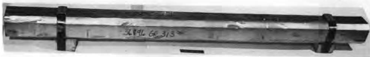
Fig. 6.16. Forged bar, 4 × 4 × 60 in., of 2% Ti-modified Hastelloy N (heat 75-421). Stock for extrusion billets to produce seamless tubing.
