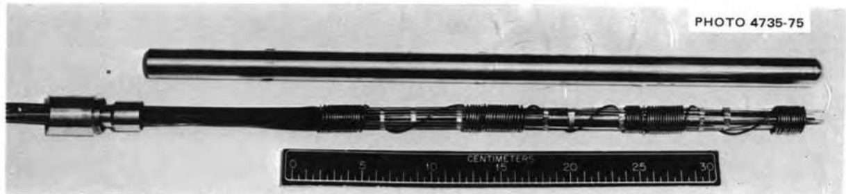
Fig. 6.78. TeGen-2 subassembly prior to insertion into the primary containment. The bottom of the assembly is on the right, and the fuel pins from left to right are numbered 1, 2, and 3 respectively.
