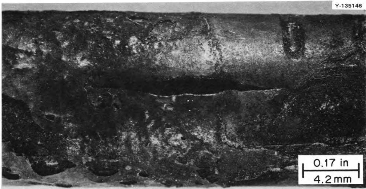
Fig. 6.28. Photograph of the second failure in FCL-2b. The tubing is \frac{1}{2} in. in diameter. 6x.
