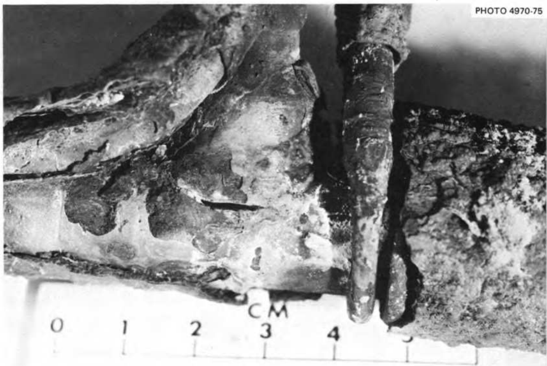
Fig. 6.31. Photograph of the third failure in FCL-2b.
