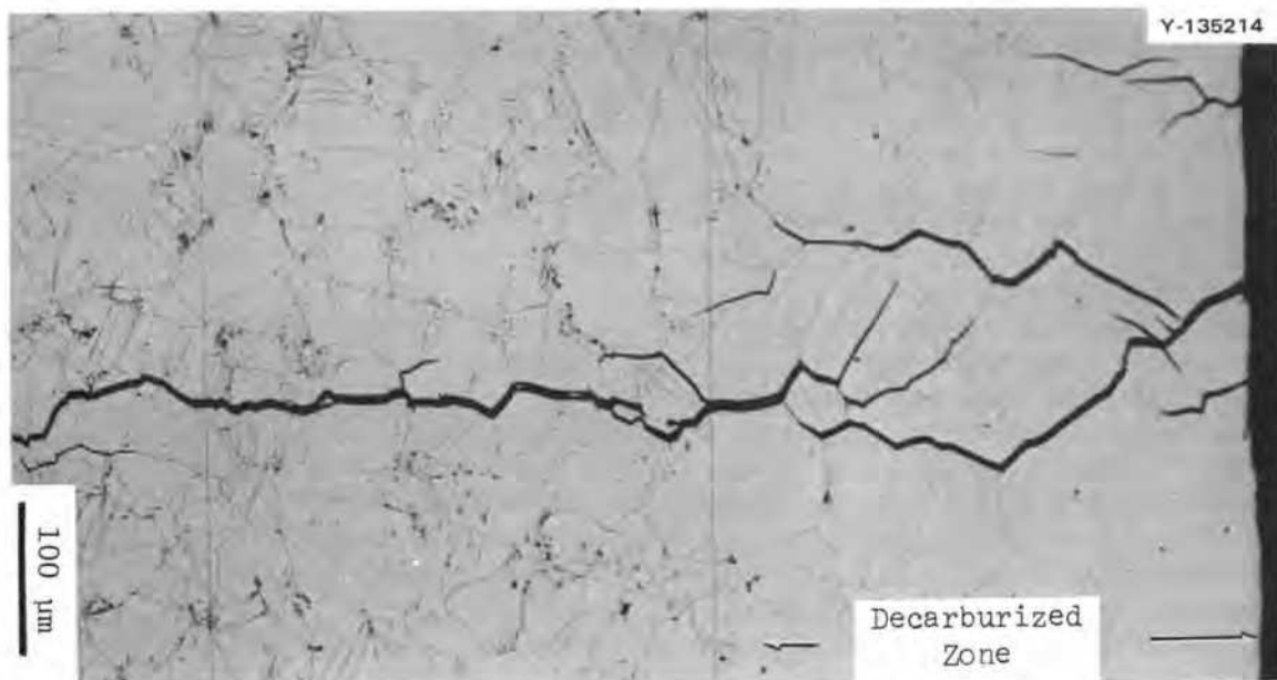
Fig. 6.46. Transverse section of 2% titanium-modified Hastelloy N annealed at 538°C for 6 hr and air cooled. Firecracking is due to thermomechanical treatments.
