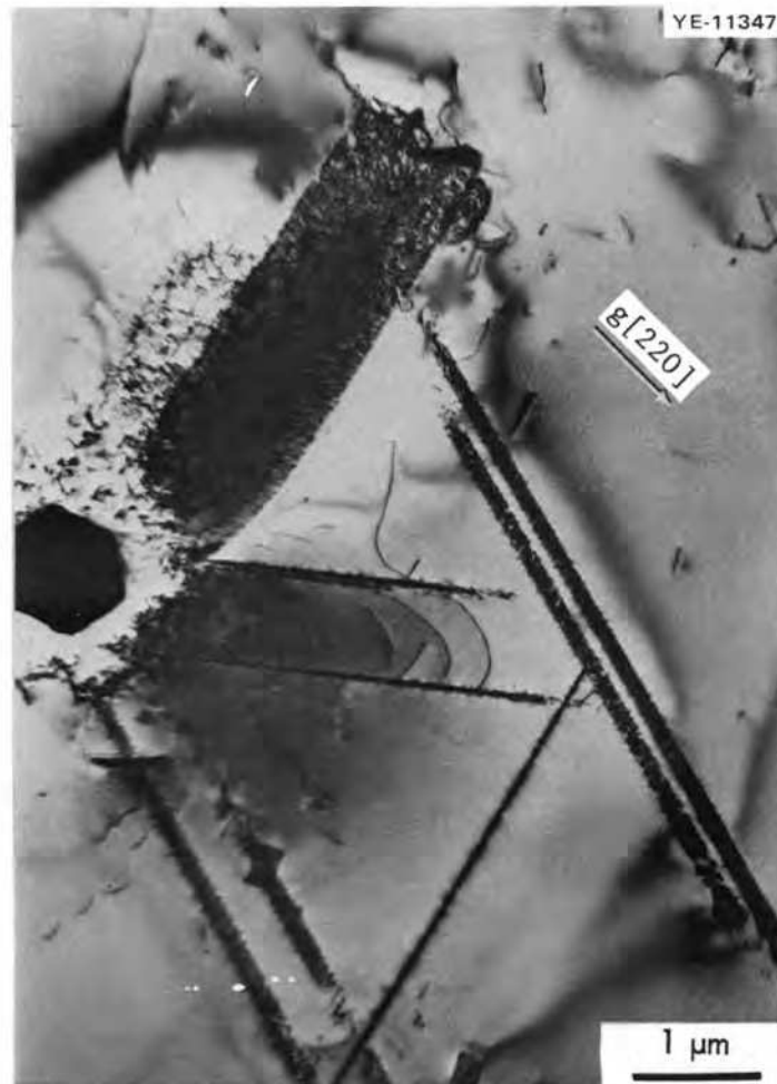
Fig. 6.9. Transmission electron micrograph showing stacking fault precipitates in alloy 452 after annealing 1 hr at 1177°C and 160 hr at 760°C.
