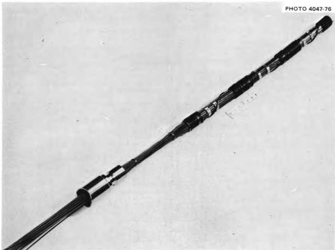
Fig. 6.79. TeGen-3 subassembly prior to insertion into primary containment. The bottom of the assembly is on the right, and the fuel pins from left to right are numbered 1, 2, and 3 respectively.
