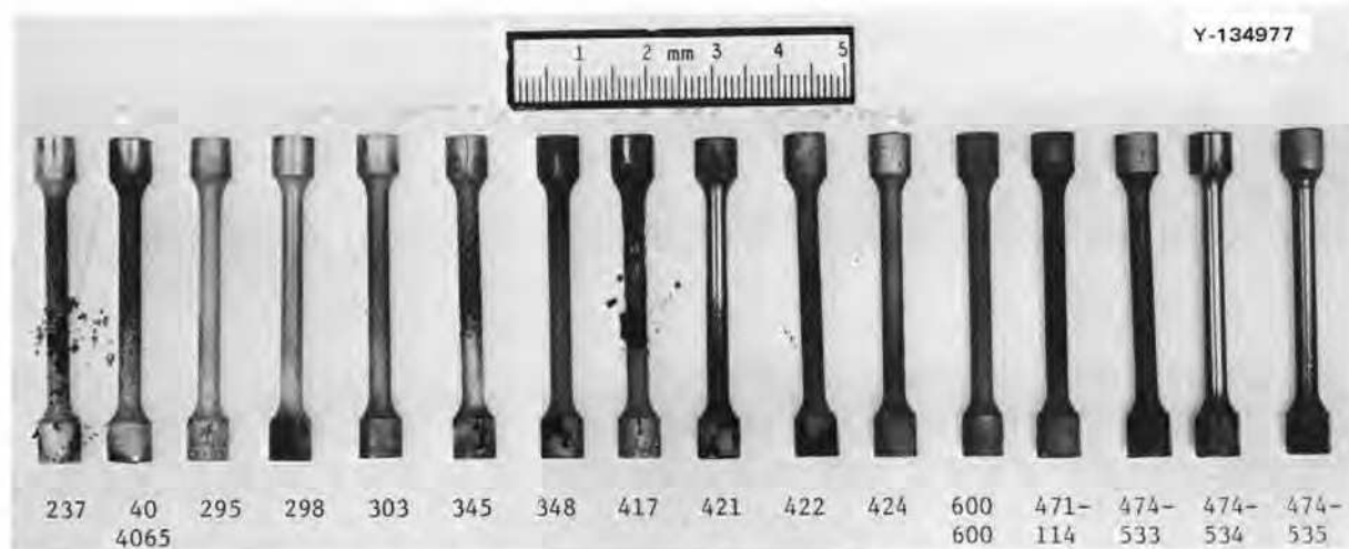
Fig. 6.58. Specimens after exposure for 1000 hr at 700°C to the vapor above \text{Cr}_3\text{Te}_4 at 700° (experiment 75-16).
