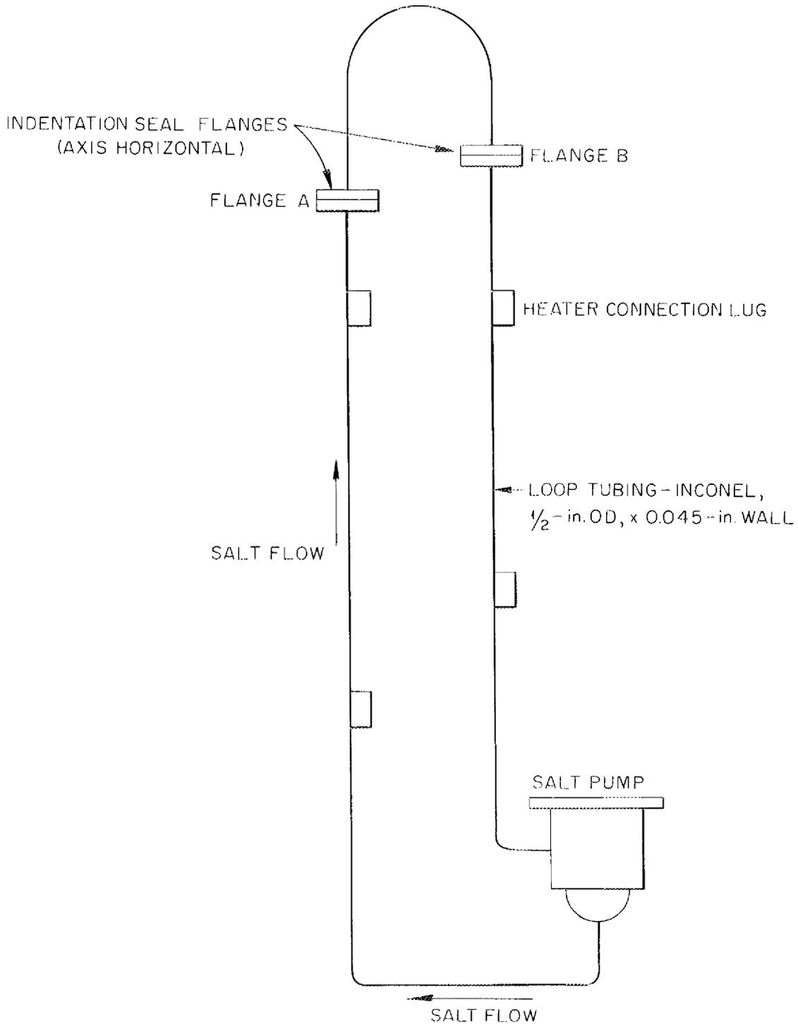
Fig. 17. Schematic Drawing of Test Loop for Indented Seal Flange Tests 1 and 2.
