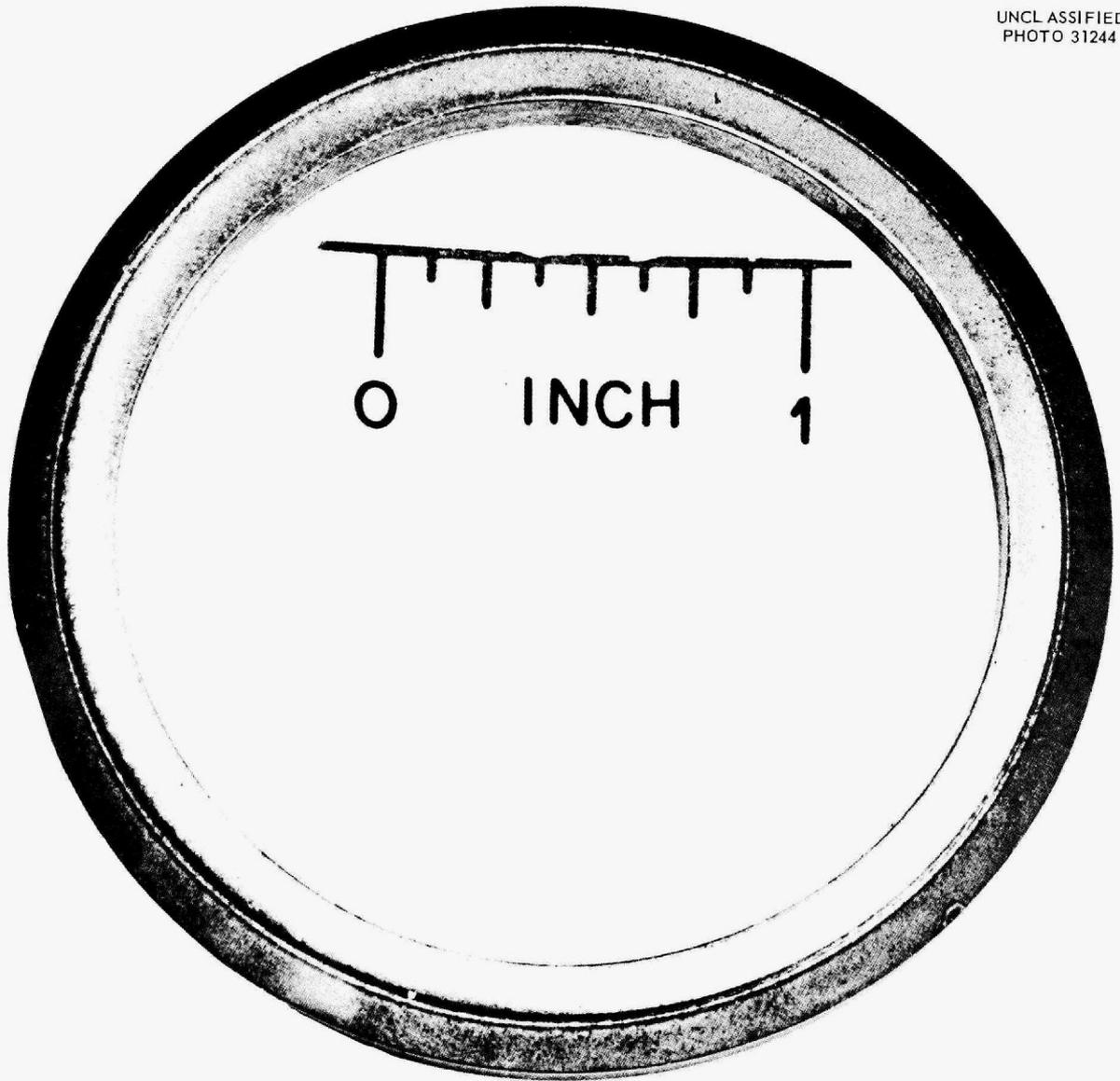
Fig. 28. Armco Iron Gasket After Testing in Indented Seal Flange.
