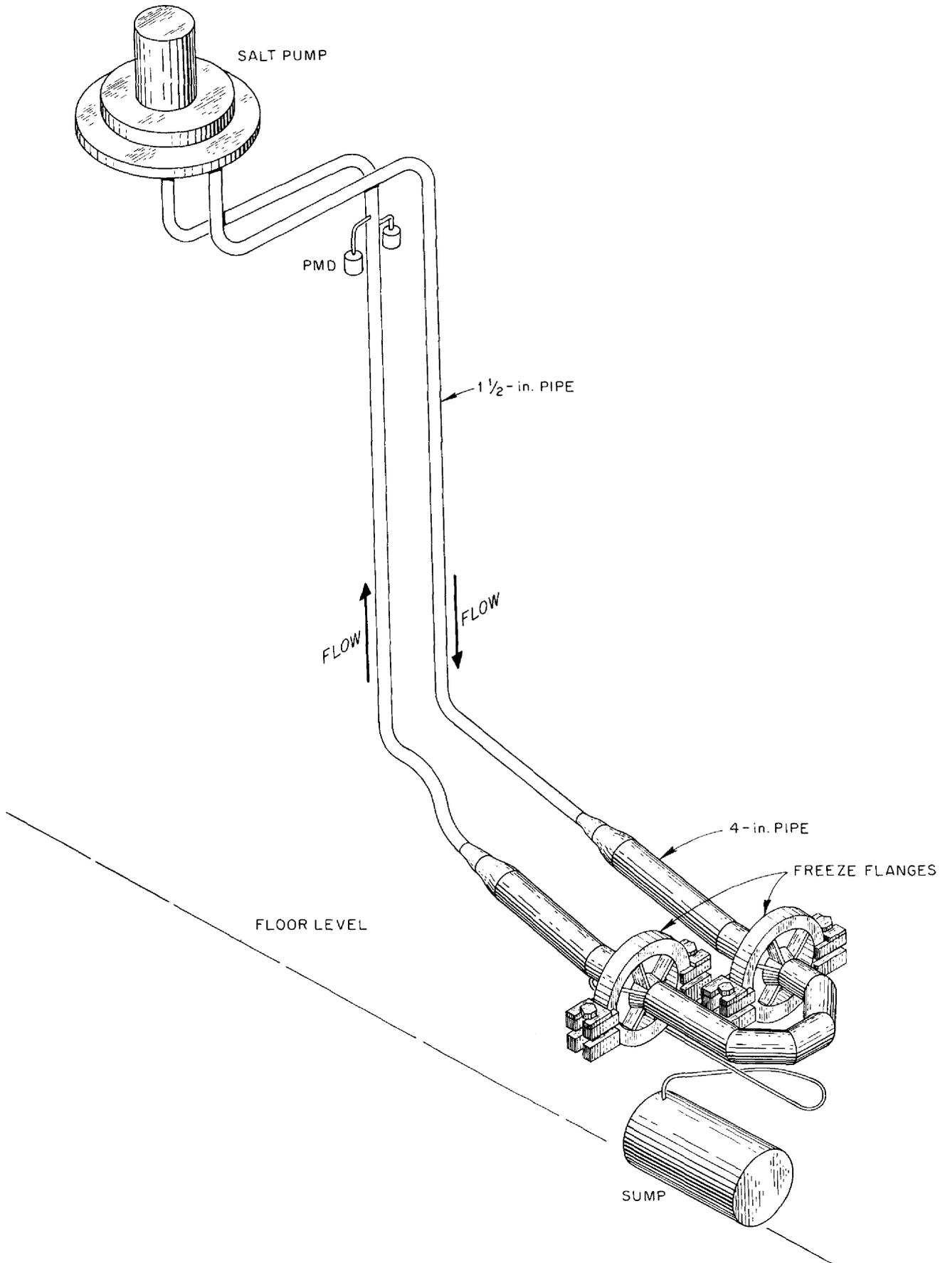
Fig. 34. Schematic Drawing of Test Loop for Large Freeze Flange.
