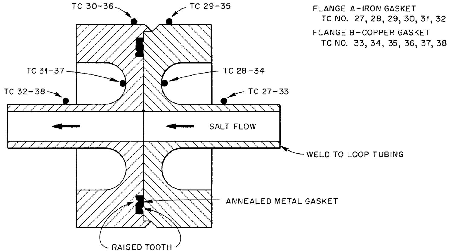
Fig. 3. Schematic Drawing of Indented Seal Mechanical Joint.
