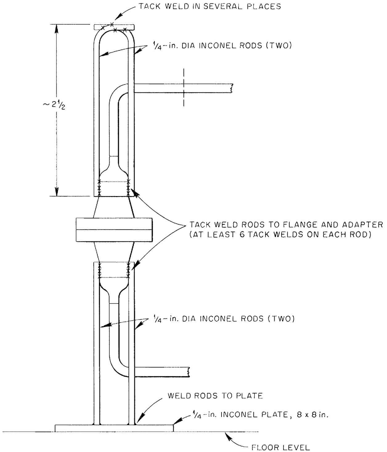
Fig. 15. Sketch of Extension Rods for Disassembly of Cast Seal Flanges.
