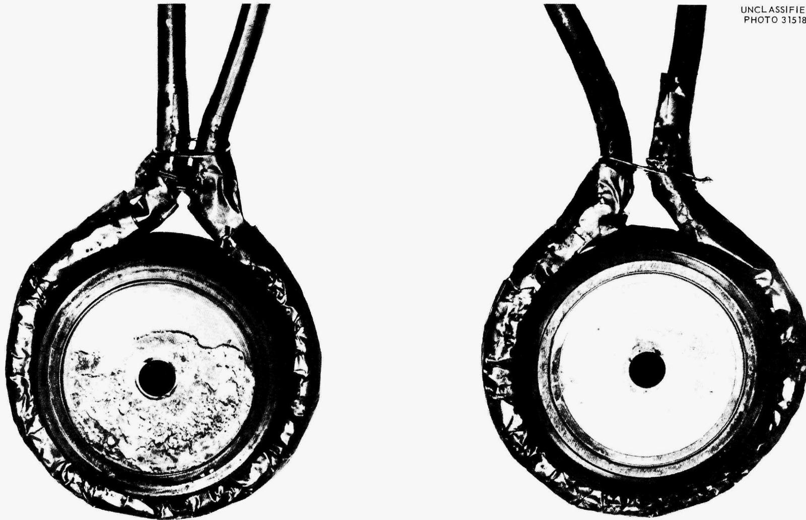
Fig. 29. Indented Seal Flange with Nickel Gasket After Testing.
