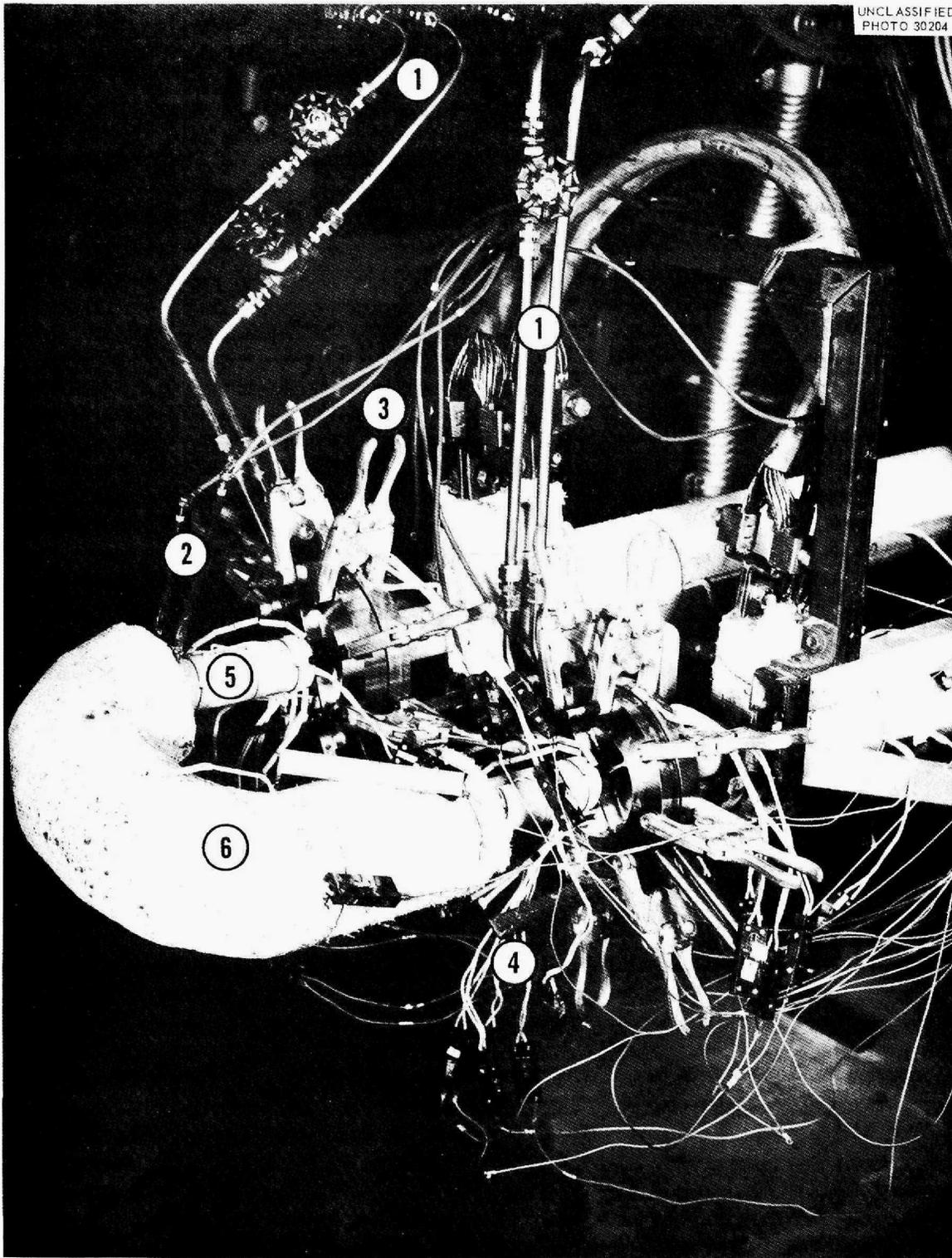
Fig. 2. Freeze Flanges Installed in Inconel Test Loop.
