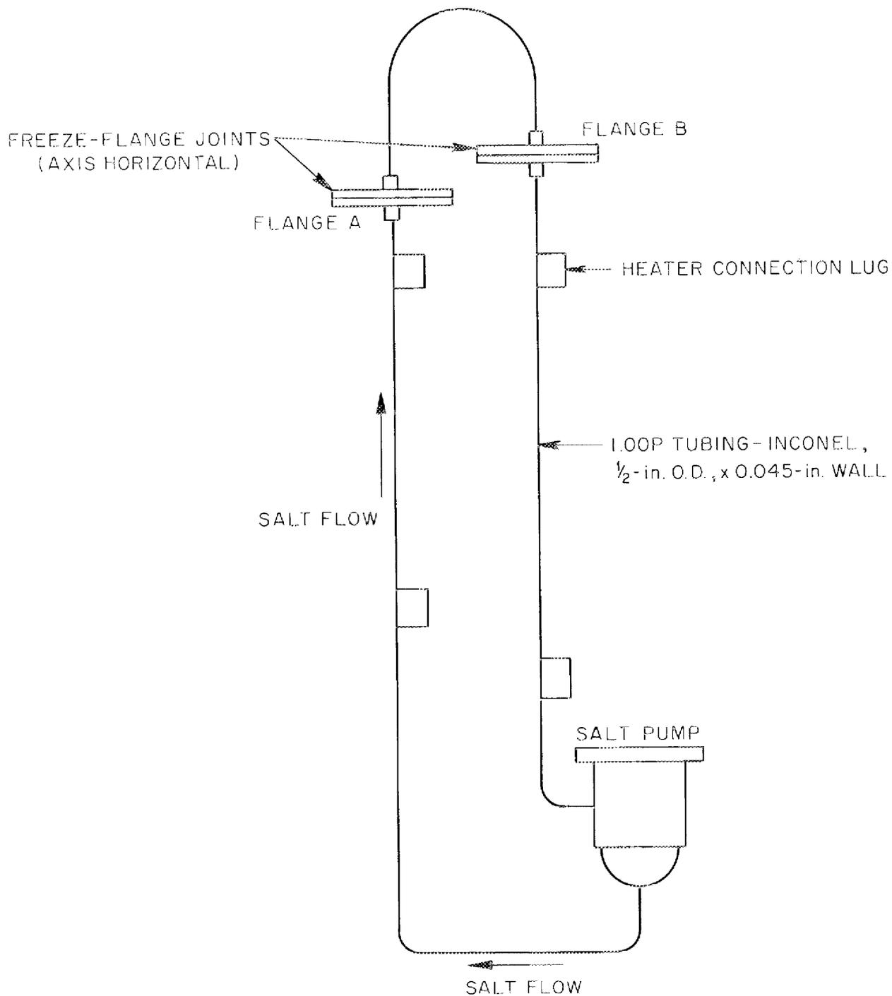
Fig. 11. Schematic Drawing of Test Loop for Freeze Flange Tests 1 and 2.
