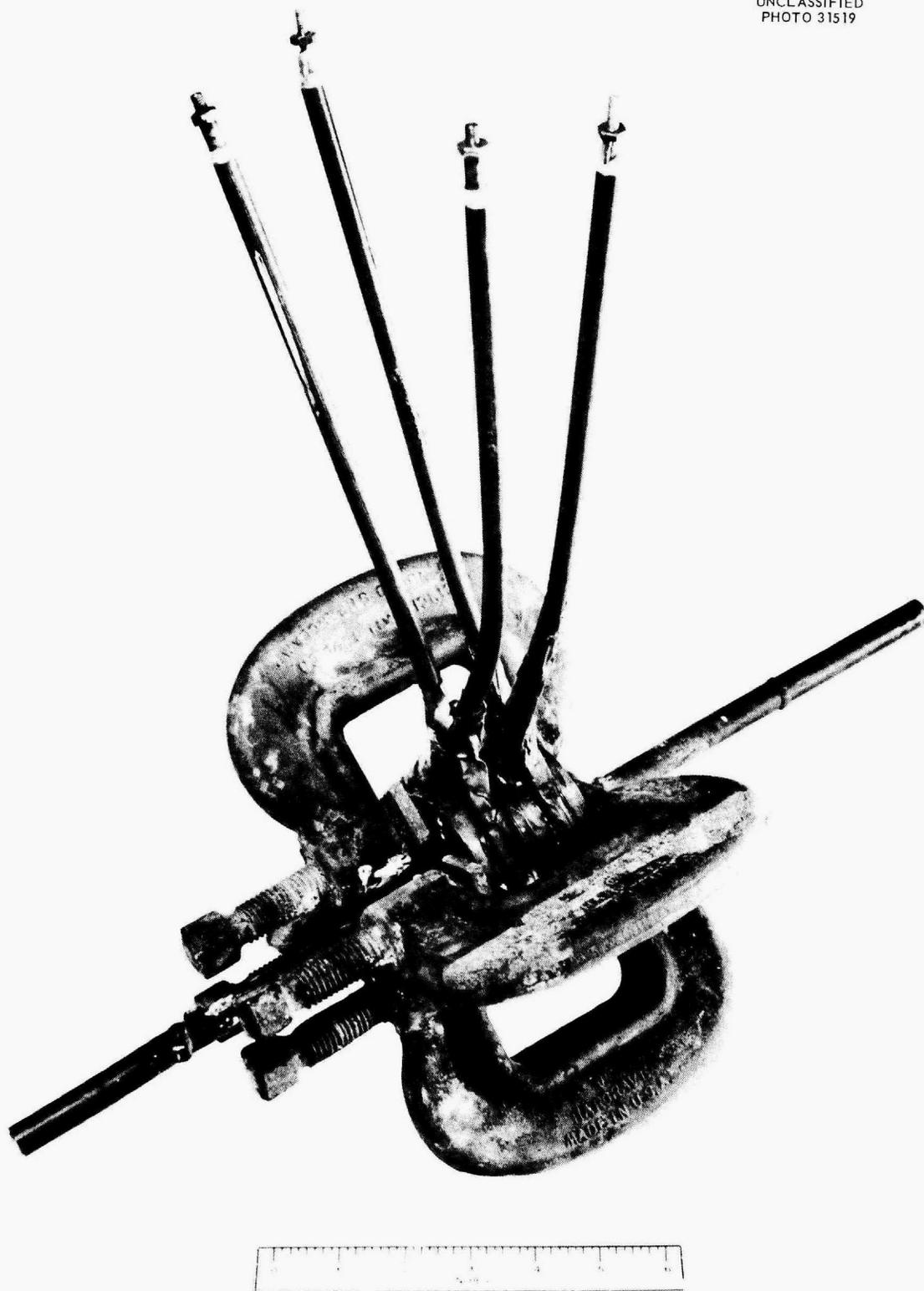
Fig. 6. Indented Seal Flange Shown Assembled with "C" Clamps.
