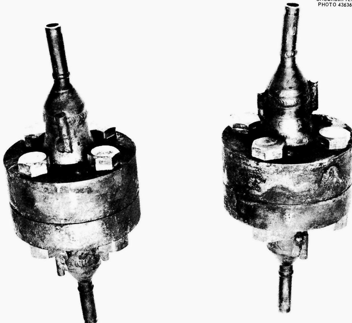
Fig. 8. Assembly of Cast Seal Flanges.
