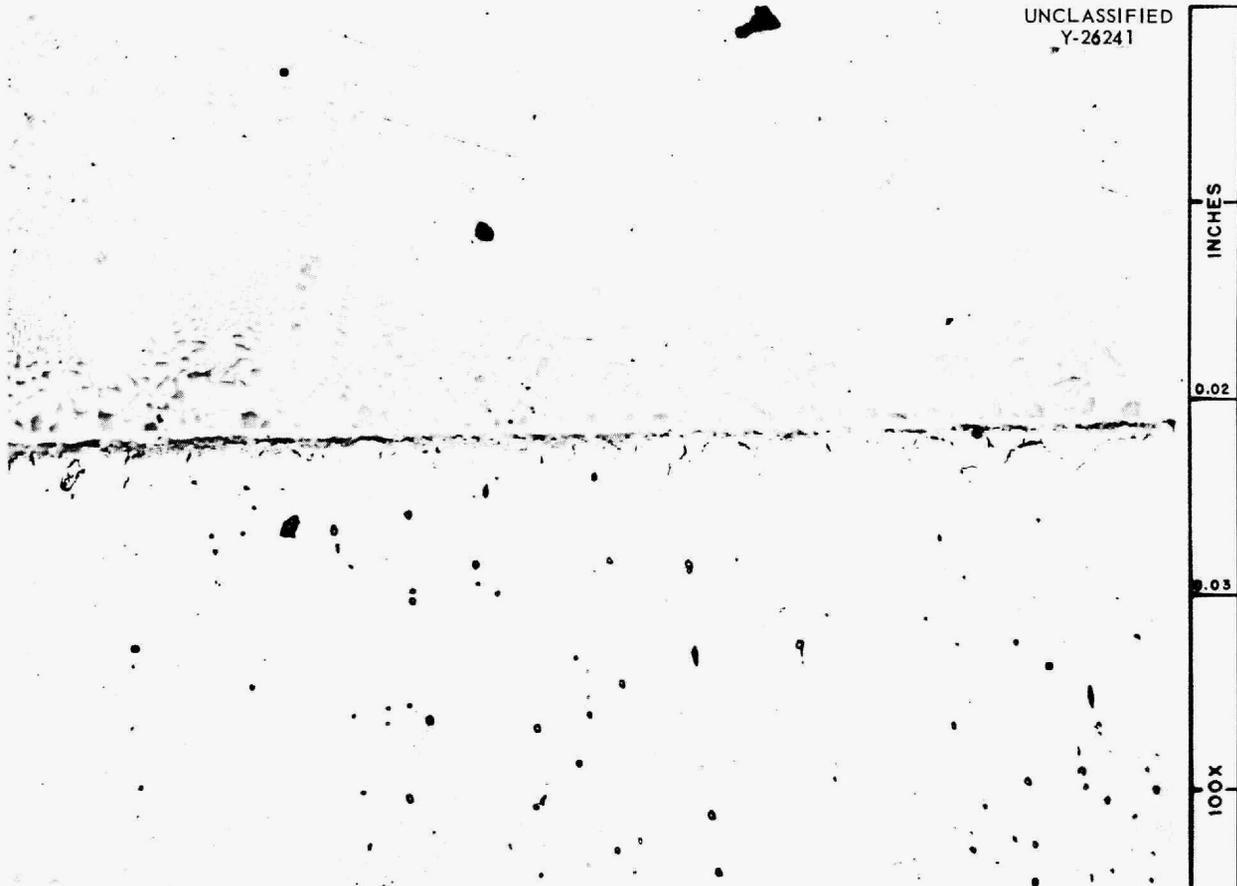
Fig. 37. Cast Seal Flange with Copper-Silver Alloy Seal; Photomicrograph of Interface of Alloy and Inconel Wall.
