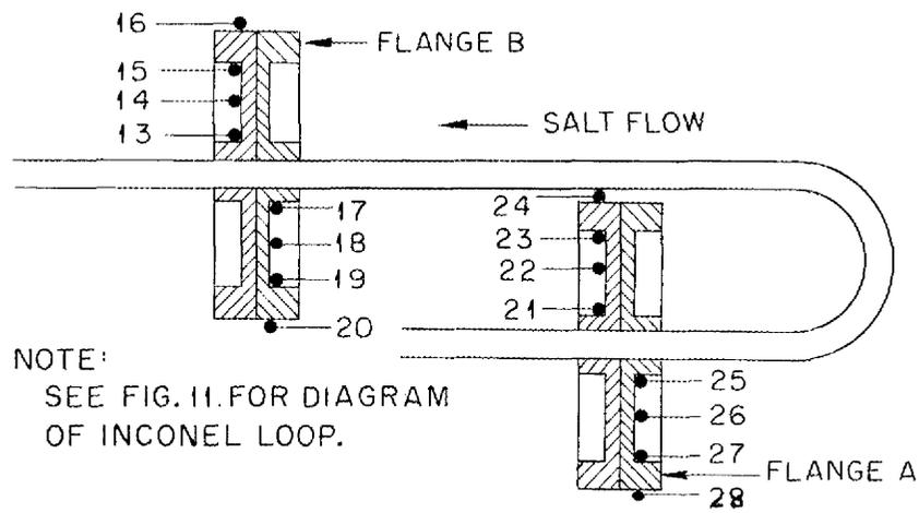
Fig. 12. Schematic Drawing of Thermocouple Locations on the Freeze Flanges for Tests 1 and 2.
