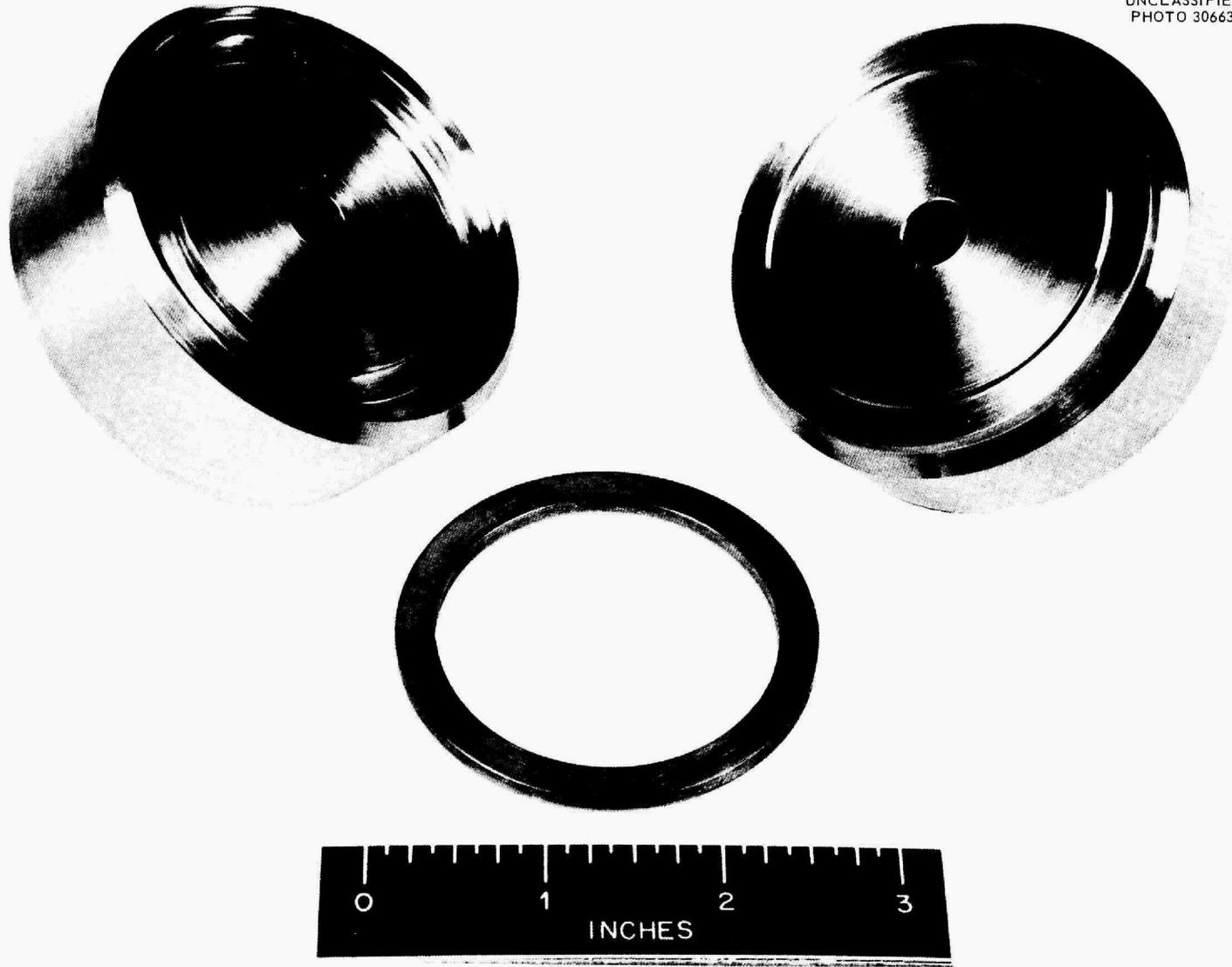
Fig. 5. Parts of Indented Seal Flange Before Testing.
