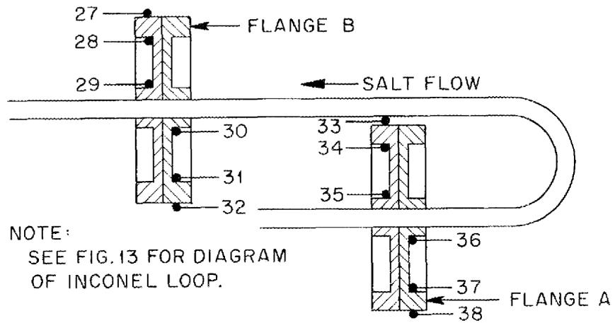
Fig. 14. Schematic Drawing of Thermocouple Locations on the Freeze Flanges for Tests 3 and 4.
