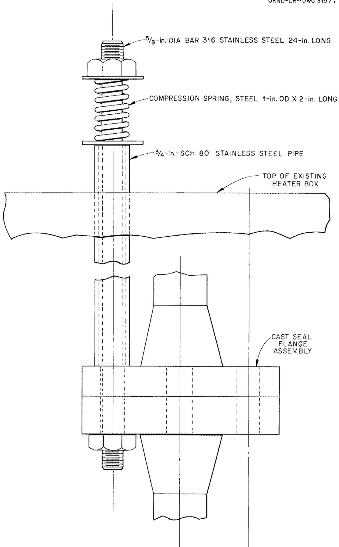
Fig. 16. Sketch of Spring-Loaded Tie Rods for Reassembly of Cast Seal Flanges.
