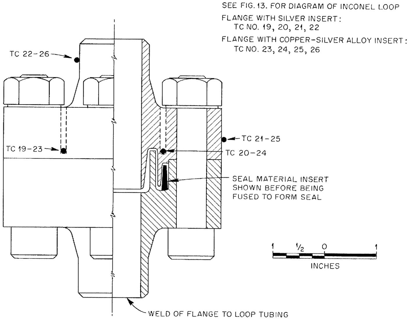
Fig. 7. Cast Seal Flange Showing a Cross Section View and Thermocouple Locations.
