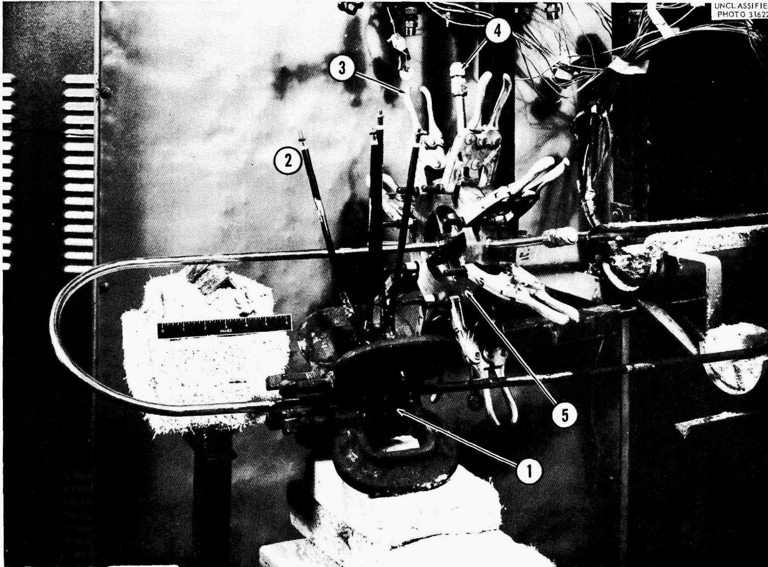
Fig. 31. Freeze Flange and Indented Seal Flange Installed in Test Loop for Cycling Tests with Molten Sodium.
