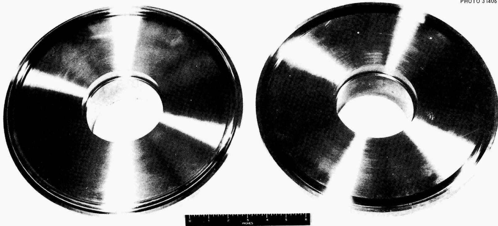
Fig. 33. Large Freeze Flange Shown Open with Copper Seal Ring in Place.
