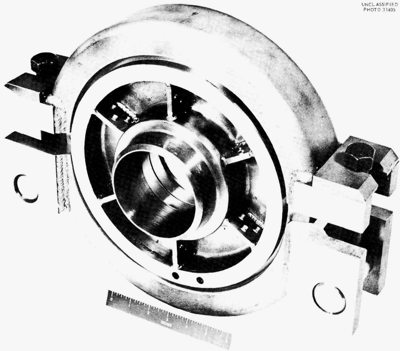
Fig. 32. Assembly of Large Freeze Flange.
