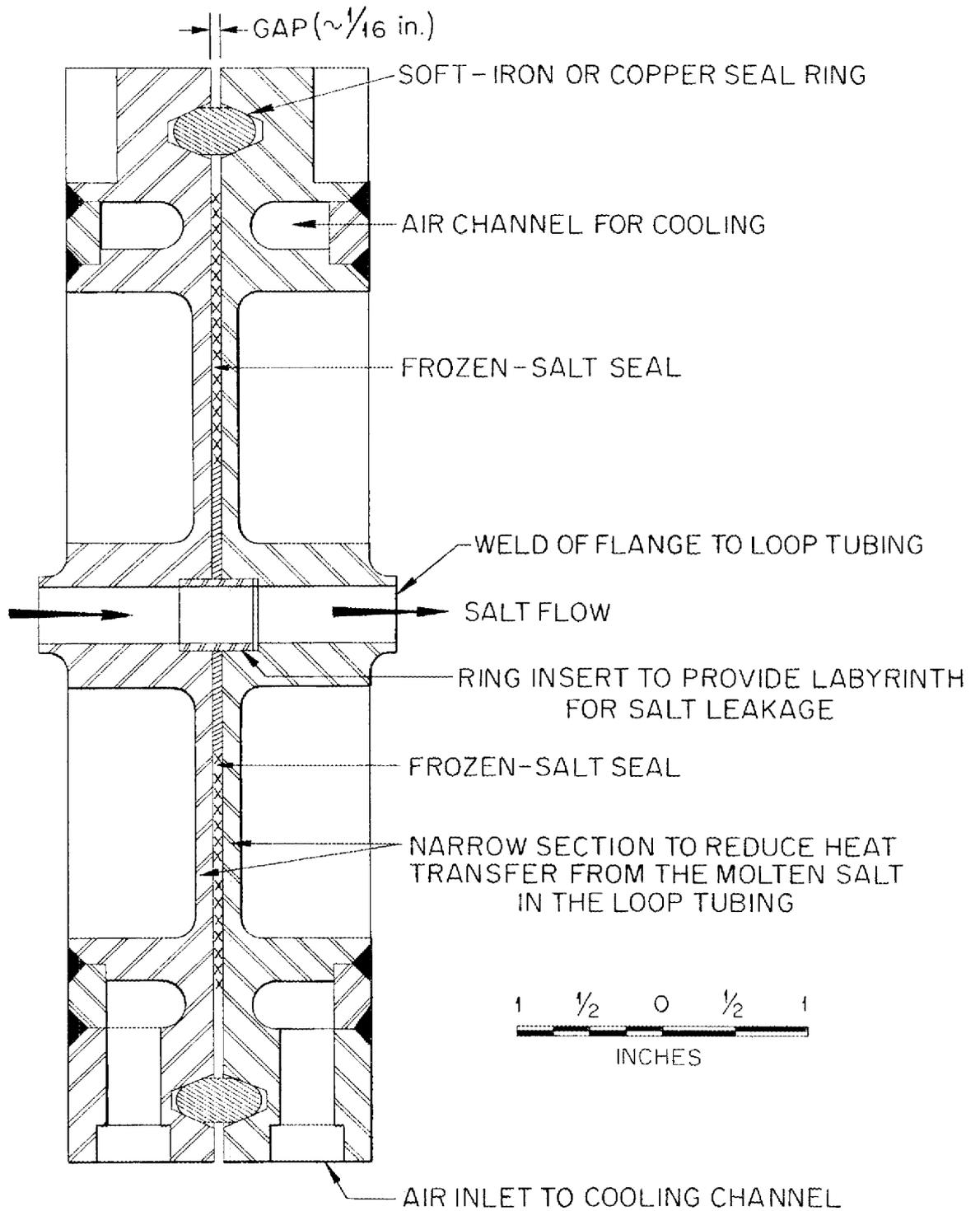
XXXXX BETWEEN FLANGE FACES INDICATE REGION OF FROZEN-SALT SEAL;
