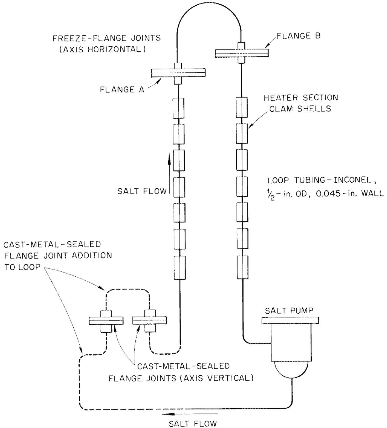
Fig.13. Schematic Drawing of Test Loop for Freeze Flange Tests 3 and 4 and Cast Seal Flange Tests 1 and 2 .
