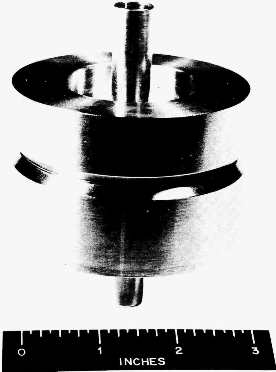
Fig. 4. Assembly of Indented Seal Flange Before Testing.
