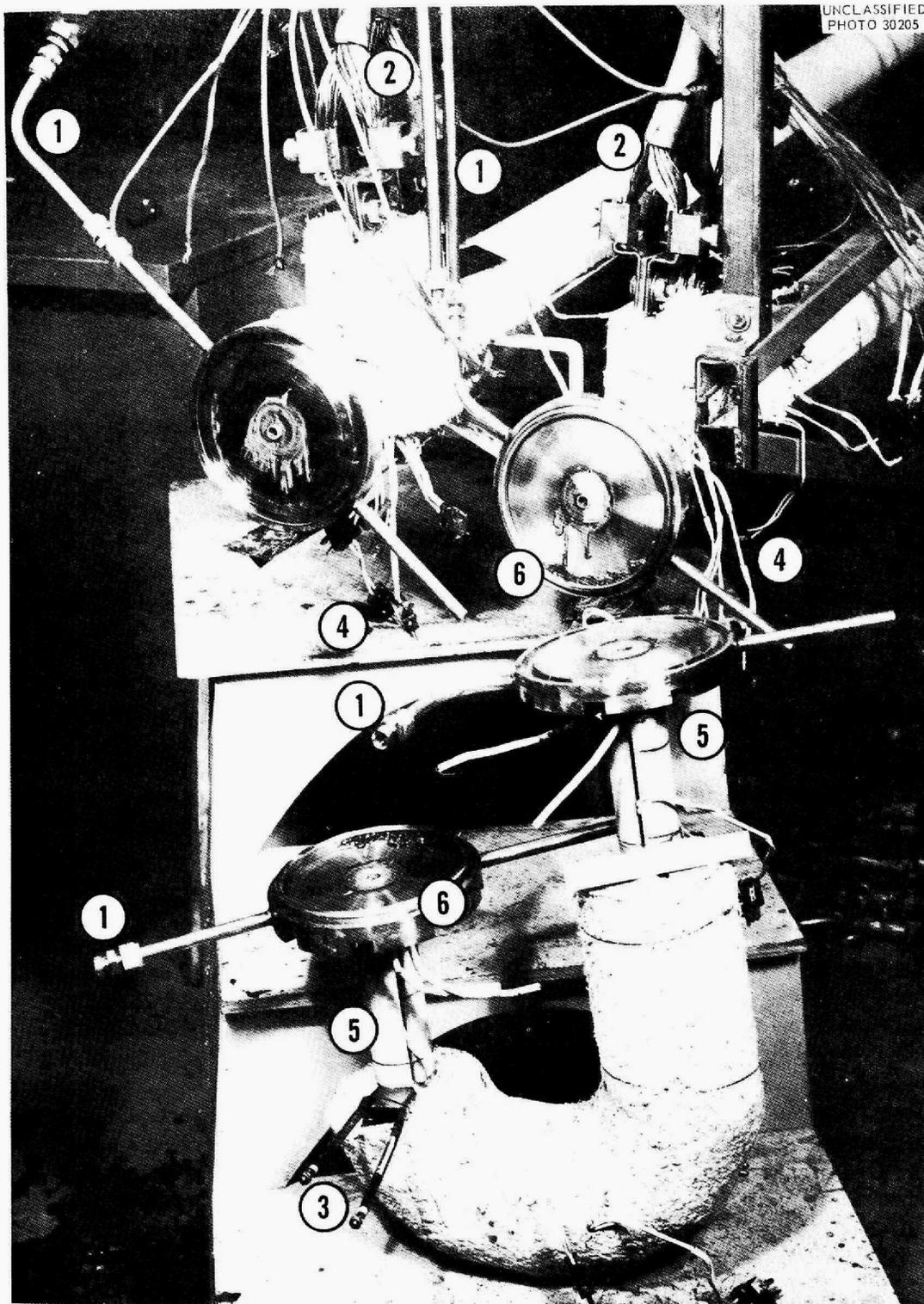
Fig. 22. Freeze Flanges Installed in Test Loop After Disassembly of the Flanges. Photo showing both flanges disassembled.
