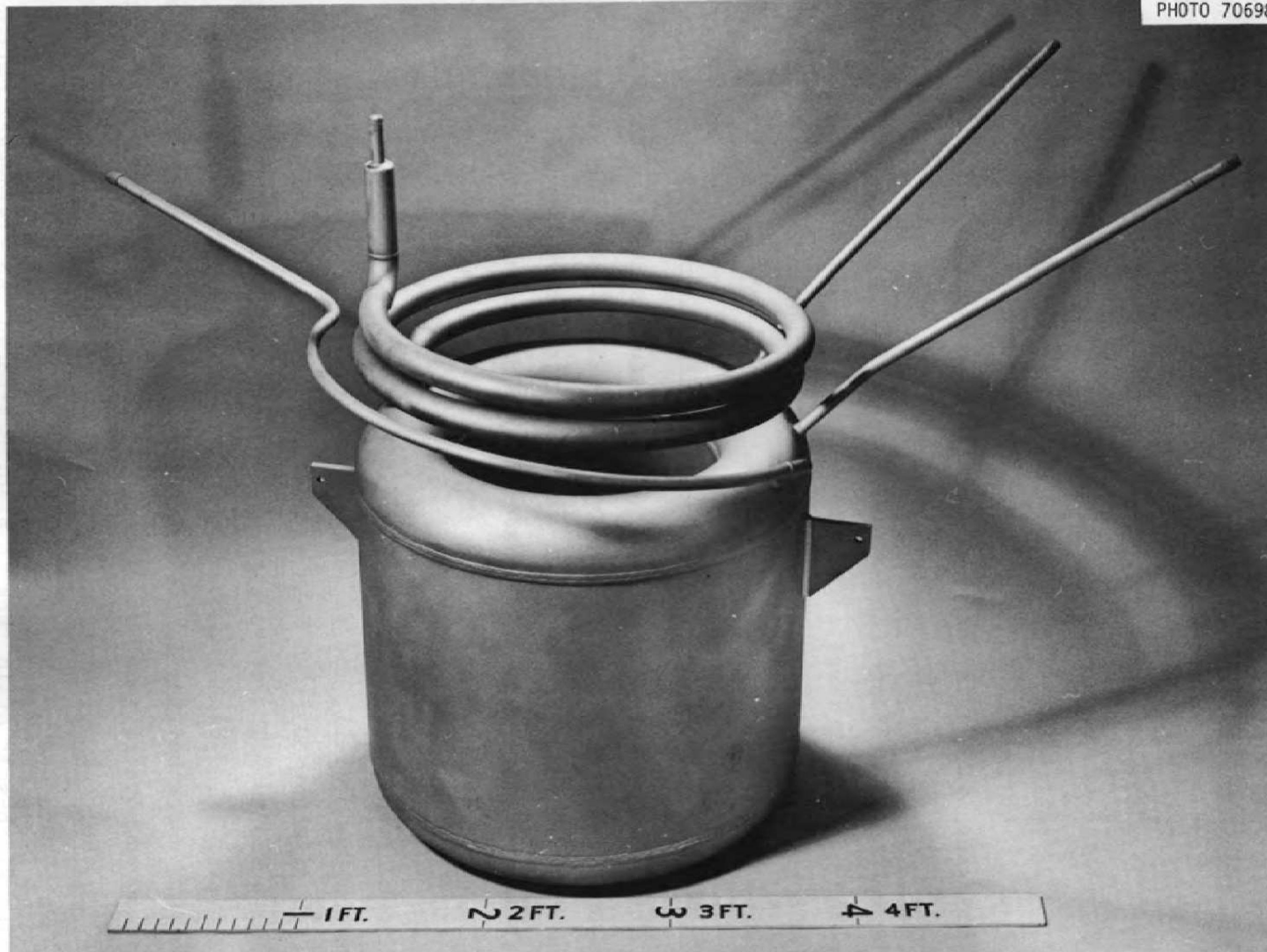
Figure 25. Fuel Pump Overflow Tank
